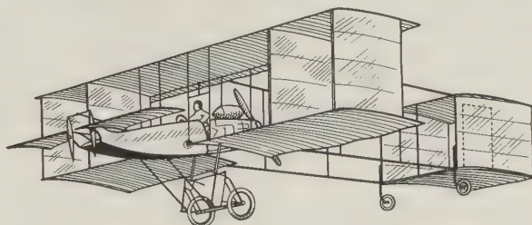
FIGURE 215—The 1908 Voisin: prototype of thirty years of successful biplane designs.
