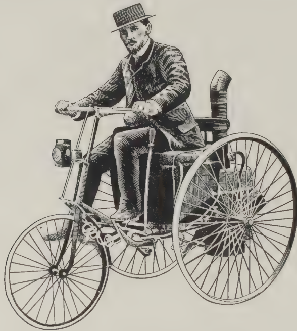
FIGURE 227— Léon Serpollet's coal-fired steam-tricycle of 1887.
