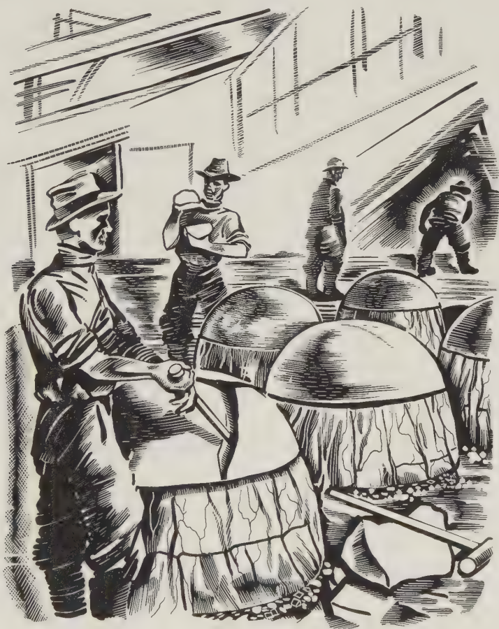
FIGURE 32—Orford 'tops and bottoms' process for separating copper and nickel.
