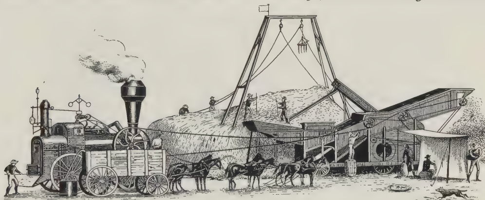
FIGURE 1—Threshing in California, 1883. The work was done on a large scale, requiring many men. In the figure, two 'tablers' are continuously employed in feeding material into the 'self-feeder'. At the right of the machine another team is continuously employed hauling away the straw, part of which is used in the furnace of the steam-engine.
