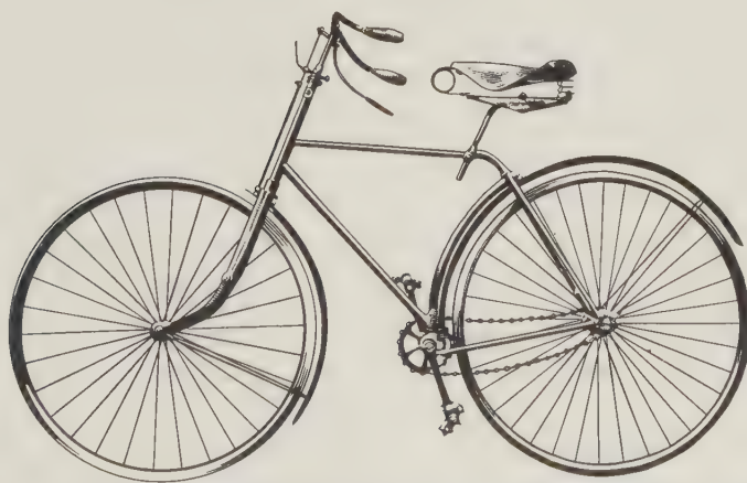
FIGURE 222—The Singer safety bicycle, 1890. Note that the steering axis passes through the point of contact of the tyre and the ground, thus improving the steering.
