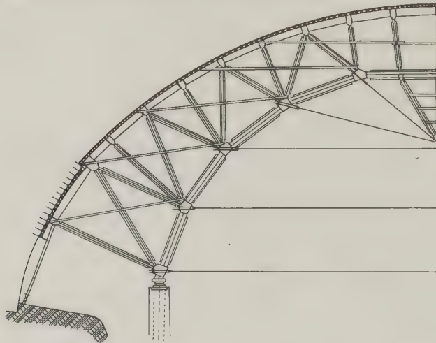
FIGURE 272—Suspended centring used for the erection of the Pont Adolphe.
