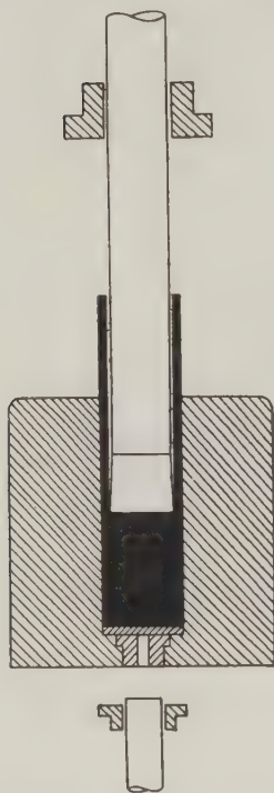
FIGURE 333—Vertical press for making closed-end copper tube shell (in section).
