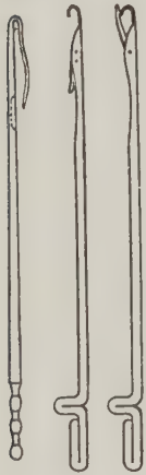
FIGURE 315—Examples of bearded needles, showing open and closed position of the latter.
