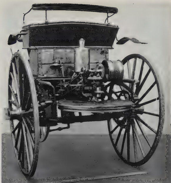
A. Rear view of an early Benz three-wheeled motor car, with back cover off, c 1888. (p 427)
