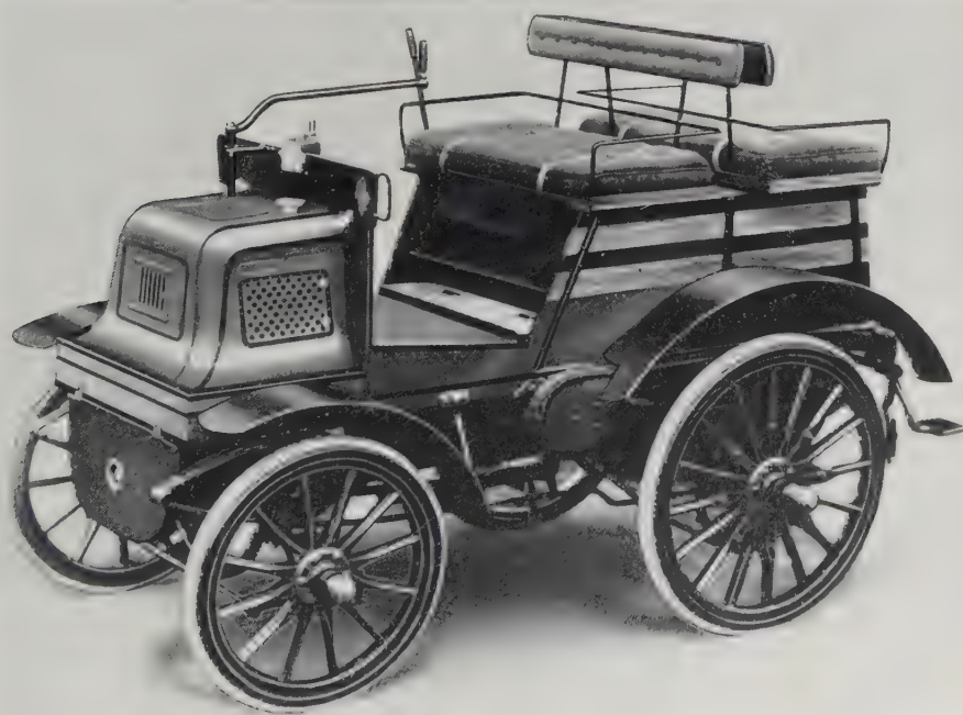
B. The earliest type of Coventry-built Daimler car, a dog-cart of 1897 fitted with a 4-hp twin-cylinder engine. (p 428)
