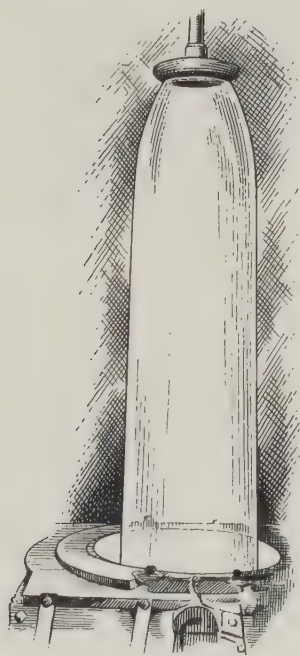
FIGURE 361—The Lubbers cylinder-blowing machine, 1903.
