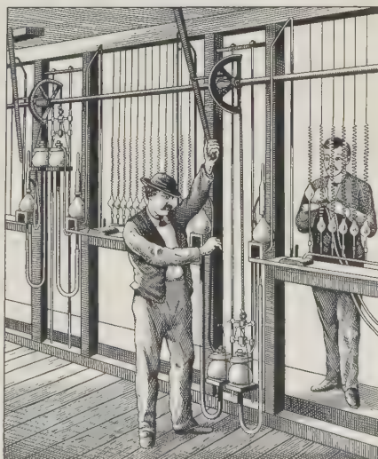
FIGURE 120—Mercury air-pump in use in a lamp factory, c 1883.
