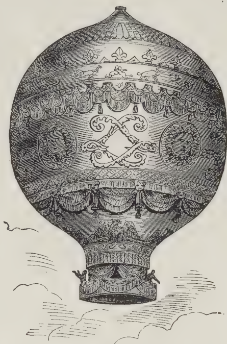
FIGURE 207—'Montgolfière' hot-air balloon of the type used for the first ascents in 1783.
