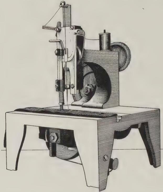
FIGURE 314—Isaac M. Singer's sewing-machine, 1851. This was the prototype of all later domestic sewing-machines, with every main feature present.
