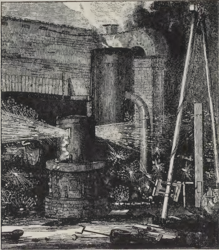
FIGURE 15—Bessemer's fixed converter. (Centre rear) Cupola furnace on the usual principle; (foreground) the Bessemer furnace; (extreme left) vessel in which the crude iron is received from the smelting furnace and then passed into the refining chamber.
