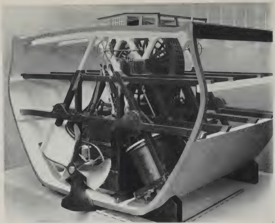
A. Model of geared engines of S.S. Great Britain, 1843. (p 147)
