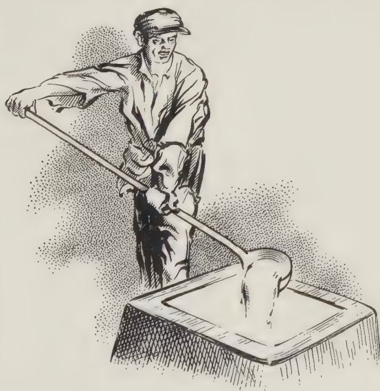
Lading refined copper in the form of flat cakes. These would be hot rolled to sheet.
