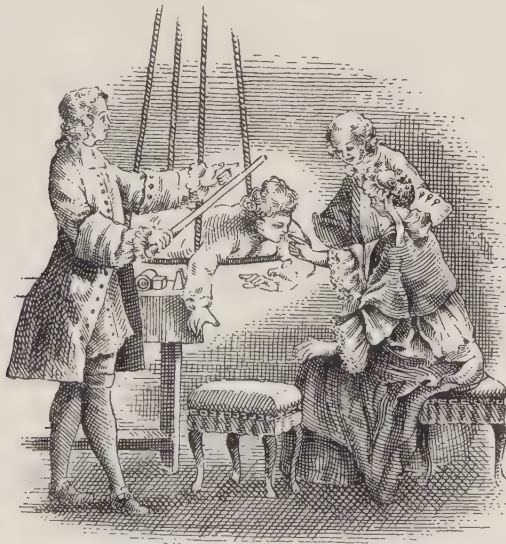
The electric fluid displayed. In Abbé Nollet's experiment, c 1750, the lady lies on an insulated plate which is charged by a cylinder machine. The bystander is amusing herself by drawing a spark from the lady's nose.
