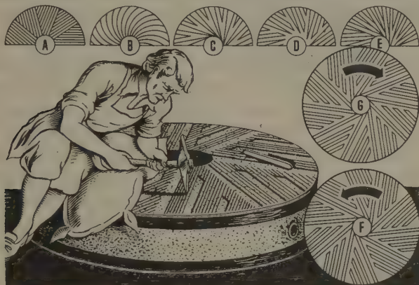
FIG. 19. Dressing millstones by hand. Insets show some traditional designs. (A) Late Roman; (B) eighteenth century; (C), (D), and (E) nineteenth century; (F) and (G) right-handed and left-handed stones in 'four-quarter' dress
