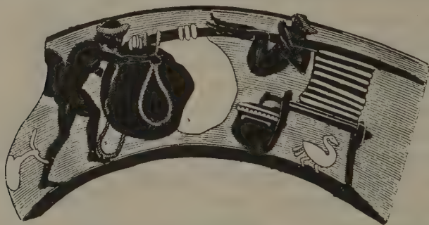
FIG. 16. Simple beam-press for olives and grapes, from a Greek vase of the sixth century B.C.
