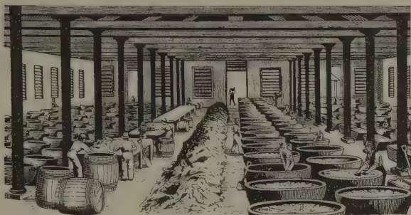
FIG. 267. Purification of soda by crystallization
