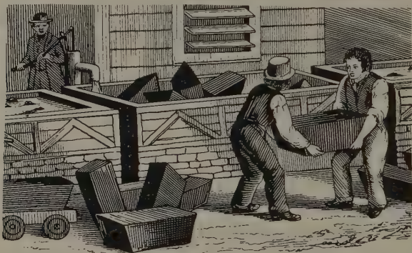
FIG. 266. Extraction of soda from black ash, in the Leblanc process
