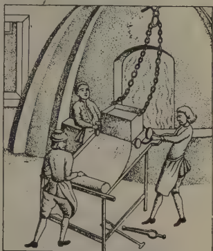
FIG. 295. Casting plate glass, c. 1780
