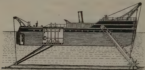
FIG. 222. French steam-driven sand-pump, from a model, c. 1865
