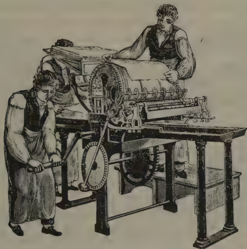
FIG. 324. Flat-bed cylinder-press made by Napier, c. 1819
