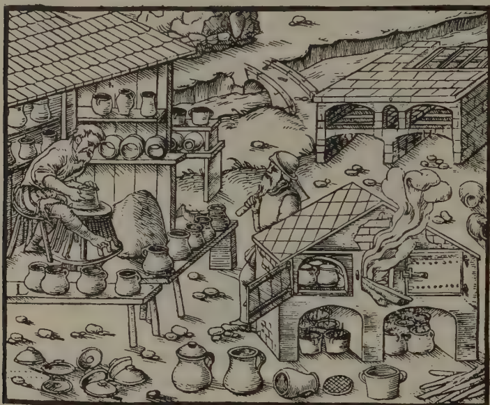
FIG. 32. Potter using kick-wheel. Agricola, De re metallica , 1556
