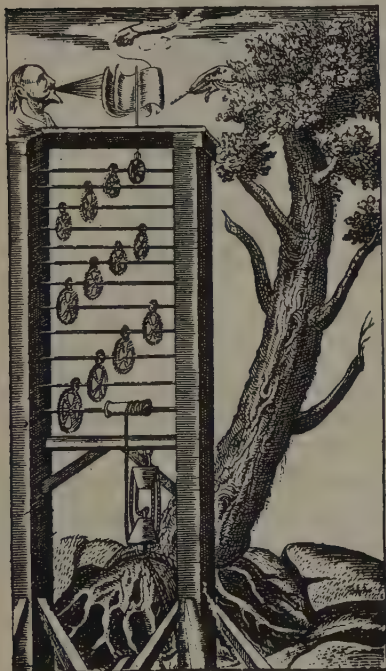
FIG. 114. Fanciful design for developing sufficient force from the wind to uproot a tree, using gearing, 1680
