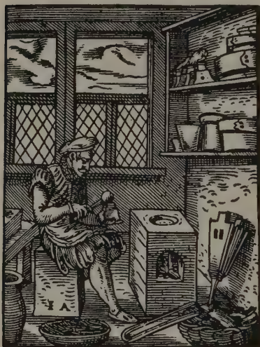
FIG. 109. Typefounder pouring molten metal into mould, 1568
