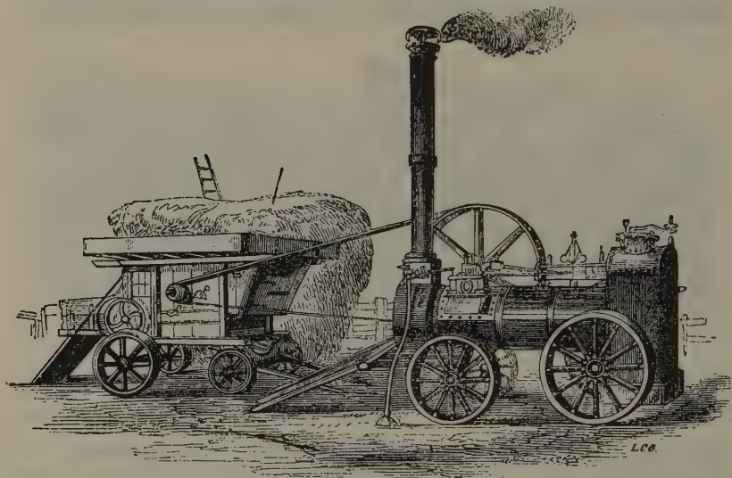
FIG. 342. Steam-driven threshing-machine, c. 1840
