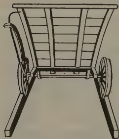
FIG. 176. Coal-wagon with flanged wheel, 1783
