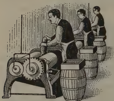
FIG. 264. Rubber-mixing mills, with pipes for steam heating
