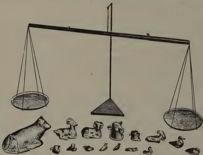
FIG. 96. Egyptian wooden balance, with 30-cm beam, showing typical animal and bird weights. El-Amarna, c. 1350 B.C.
