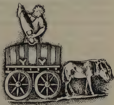
FIG. 174. Late Roman tank-wagon for the conveyance of wine
