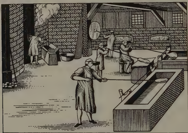
FIG. 294. Glasshouse for making crown glass, c. 1800
