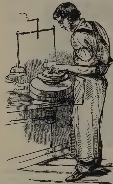
FIG. 291. Pressing flat hollow-ware, c. 1814
