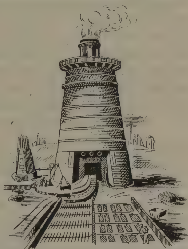
FIG. 245. British blast-furnace, showing preheater and moulds in which the pig iron is cast, c. 1850
