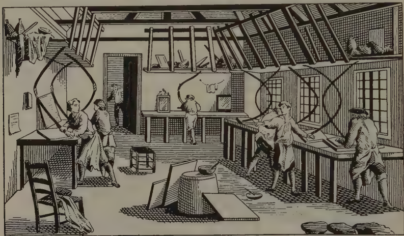
FIG. 296. Buffing or polishing plate glass for mirrors
