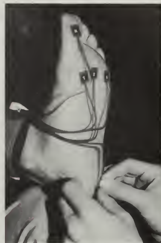
Foot sensors are placed on a runner's feet to capture his movements in a computer memory.
