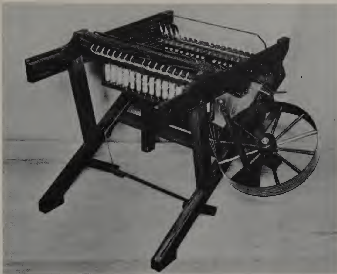
Reconstruction of the spinning jenny, patented by James Hargreaves in 1770, by which 16 threads could be spun simultaneously (Crown copyright; courtesy of the Science Museum, London)
