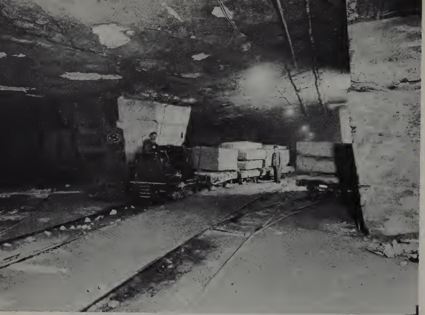
Monks Park Quarry: haulage system and pillars of stone left to support roof
