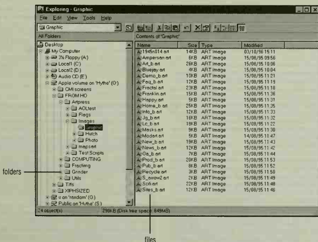
directory A graphical illustration of the directory filing system on a computer. On the left hand side of the screen are the sub-directories available from the root; on the right are the files contained within the active directory.
