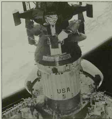
Galileo The Galileo spacecraft about to be detached from the Earth-orbiting space shuttle Atlantis at the beginning of its six-year journey to Jupiter. National Aeronautics and Space Agency
