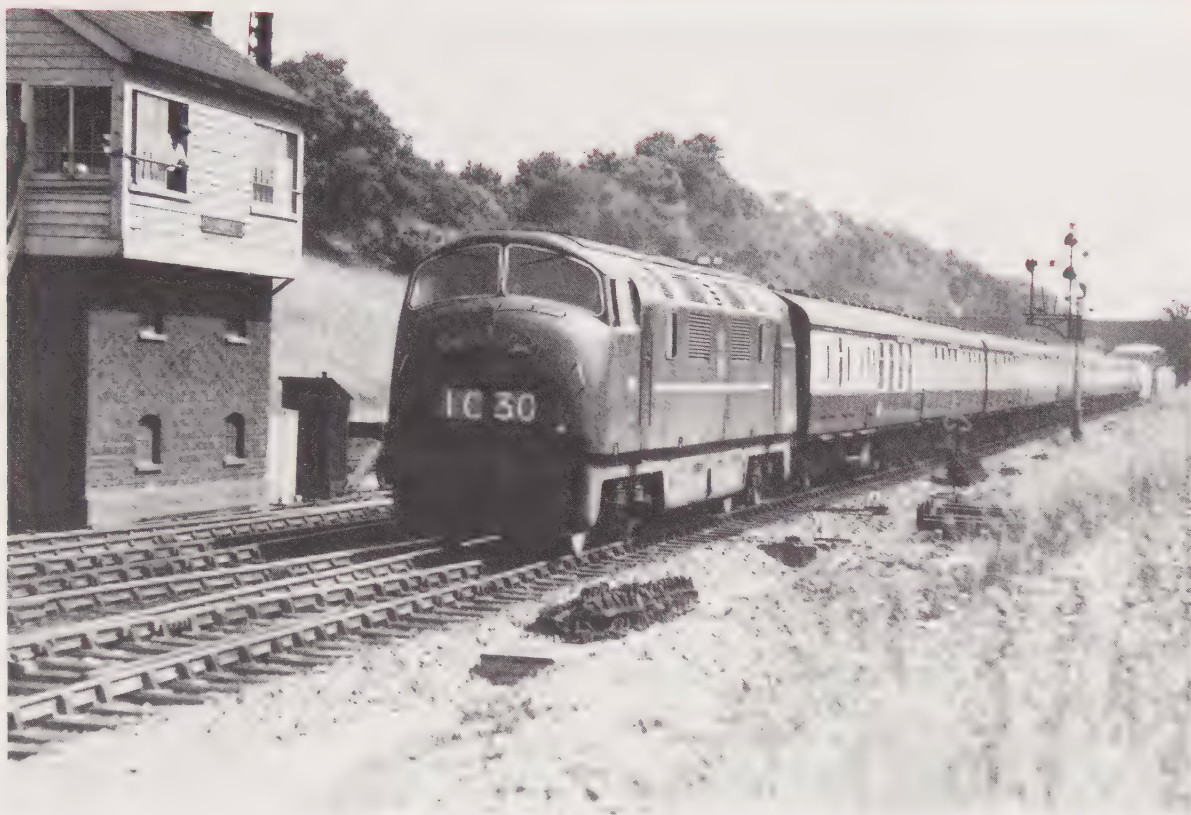
Plate 87: BR class 42 'Warship' diesel-hydraulic on the 'Cornish Riviera' train in 1960.
