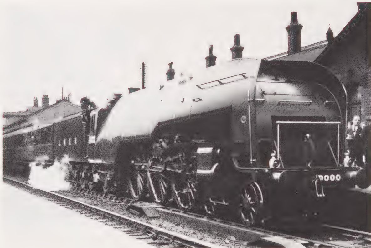
Plate 60: Gresley's experimental W1 4-6-4 express locomotive, equipped with a marine boiler and streamline casing. The novel external design was to become familiar on the LNER with the appearance of the P2 2-8-2s and the A4 Pacifics.
