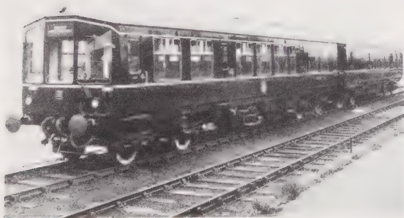
Plate 88: BR two-car lightweight diesel multiple unit built in 1954 for service on the North Eastern Region.
