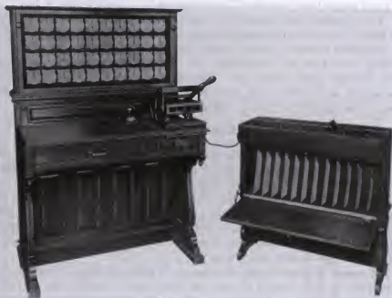
Fig. 94. Hollerith's original tabulating and sorting machine. (Photo courtesy of IBM archives.)
