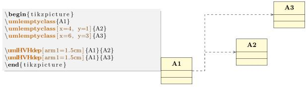
The arm1 and arm2 options also take negative values. How does it work then? A positive value means an arm oriented to the right direction (to the right or to the top), whereas a negative valuemeans an arm oriented to the opposite direction, that allows you to draw other 3-segments relations:
