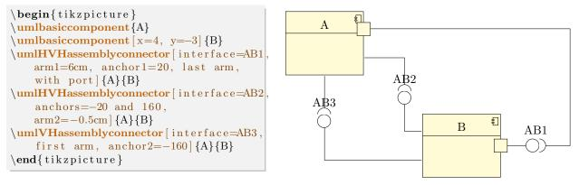
The position of the ports is automatically evaluated according to the values given to these options and to the geometry option.
