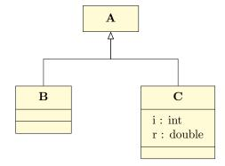
In a similar way, you may use anchor=east to right align classes, anchor=west to left align classes or anchor=south to bottom align classes.
