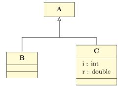
The y coordinate defines the center of the class node. It will be better in this example to have classes B and C top-aligned. A solution is to define manually the y value for C, but it is not very convenient. You may prefer use the anchor option. If you specify anchor=north, the y coordinate will define the top center anchor of the node, instead of the center. You may take a look at the differences between both codes.
