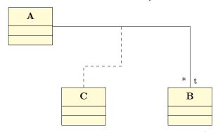
As the command is like a class and a relation, you can use the following options: x, y, width (default is 10ex), type (default is class), template coming from the umlclass environment, and name, geometry (default is - -), weight, arm, anchor1, anchor2, and anchors coming from the umlrelation command.
