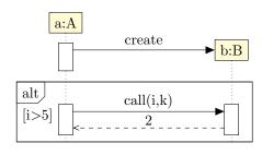
The inner xsep option allows to shift type and label to the left. The default value is 1 and its unit is ex.
