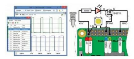
We will use the PWM feature to fade an LED by changing the duty cycle value.
