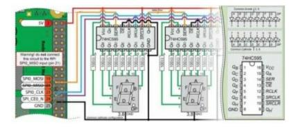
The 74HC595 can be connected to the Raspberry Pi board using three of the four SPI lines.
