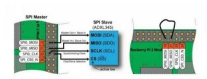
SPI bus works using one of the four modes that are chosen based on the specification defined in the data sheet of the SPI device. The data can be synchronized by the clock signal and any of the communication modes. The polarity can be defined if the clock is low or high.
