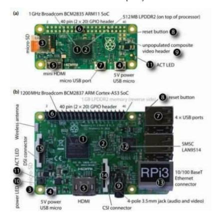
**1. Processor**: The Raspberry Pi uses the Broadcom BCM2835/BCM2836/BCM2837 processor.
