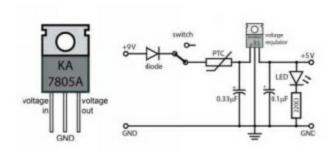
A diode is a semiconductor that allows the current to pass in one direction.
