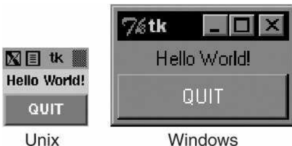
Figure 19-3. Tkinter Label and Button widgets (tkhello3.py)
