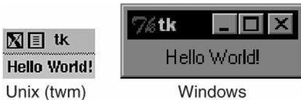
Figure 19-1. Tkinter Label widget ( tkhello1.py )
