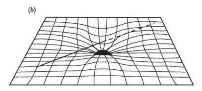
4. The curvature of space. In the absence of a source of gravitation, light travels in a straight line. If a massive object is placed near the light path, the distortion of space produces a bent light ray.
