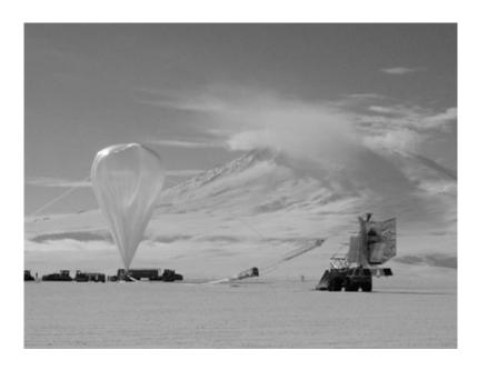
26. BOOMERANG. The picture shows this experiment about to be launched on a balloon in Antarctica. The experimental payload is perched on the vehicle to the right. The flight path of this balloon took it around the South Pole, making use of circulating winds to return it near the point of launch. Antarctica is very dry, making it the best place on Earth for microwave background experiments, but it is still better to get out into space if possible.
