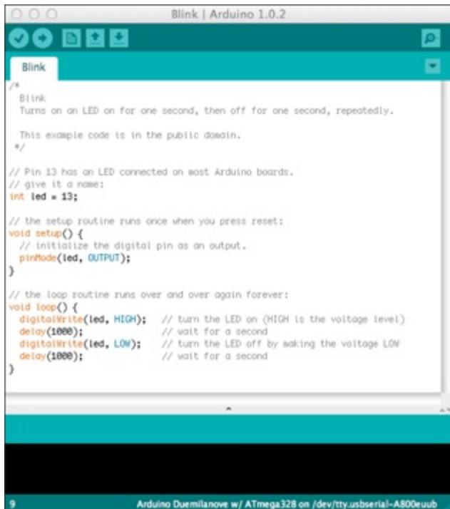
Figure 3-2: The Blink program loaded into the Arduino IDE.
