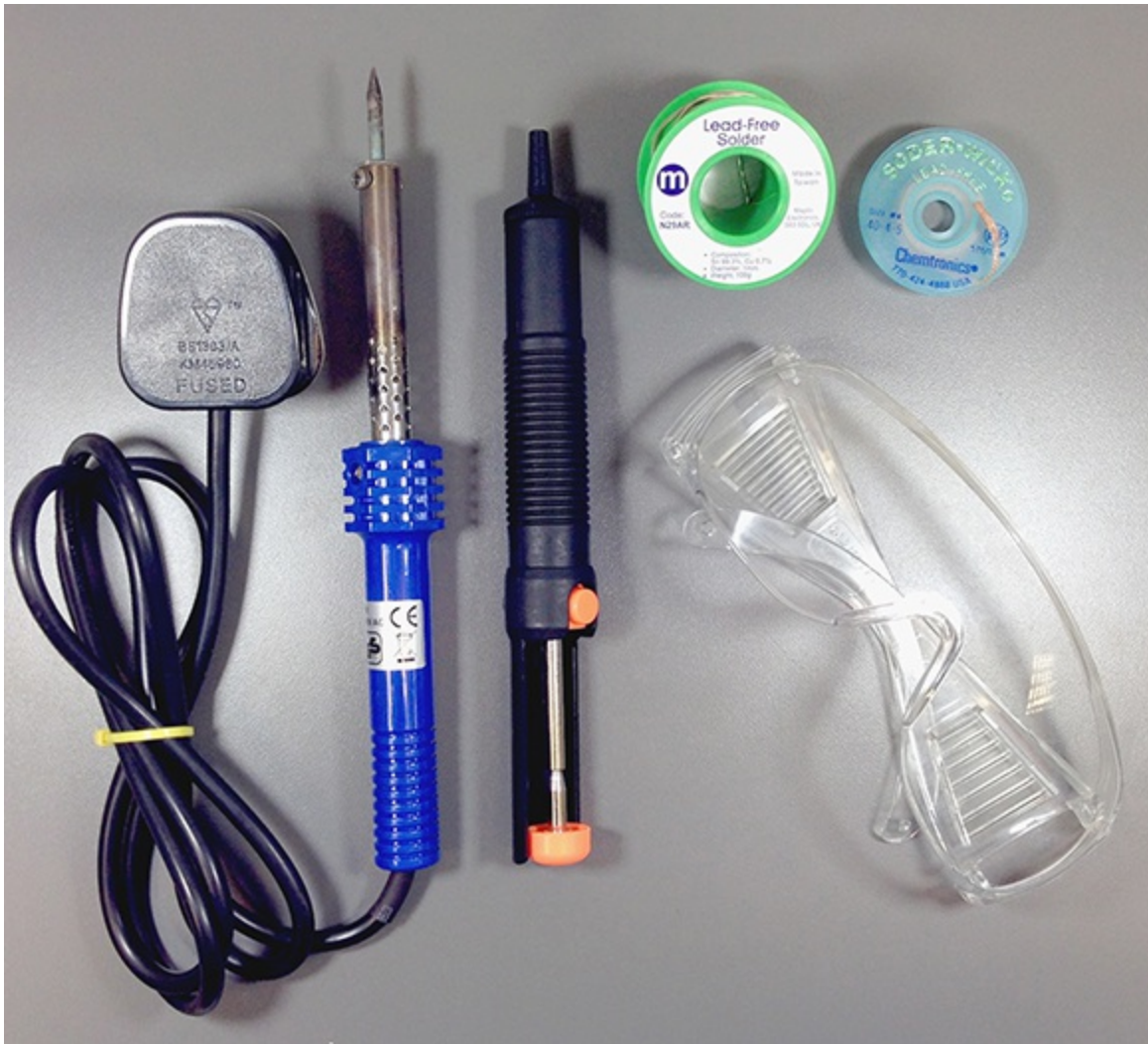
Figure 2-6: An entry-level soldering iron and essential accessories.
