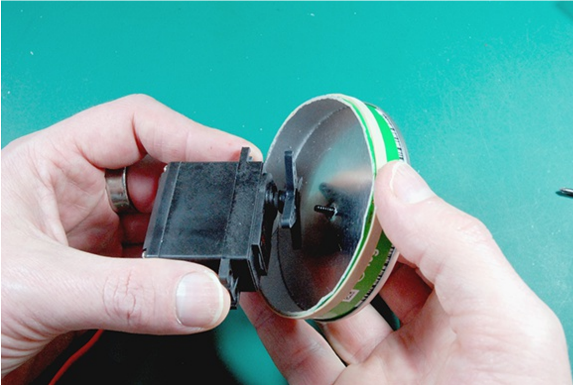
Figure 14-12: Mounting your wheels to the servo motors.
