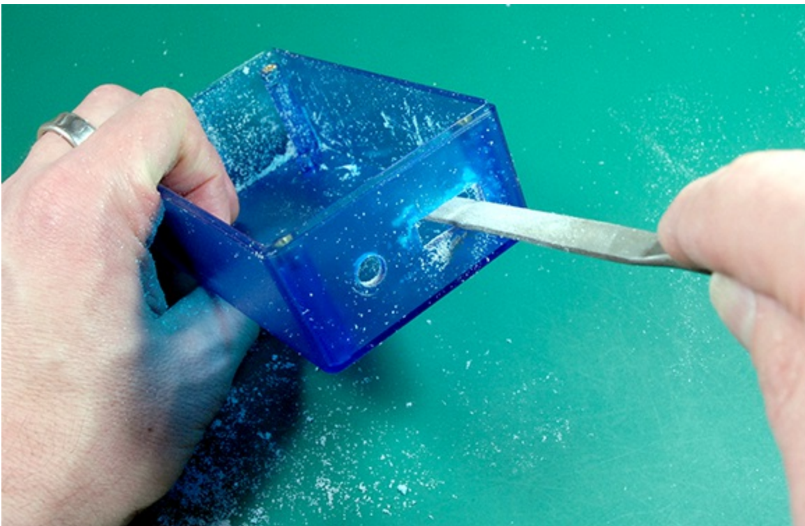
Figure 13-12: Filing the hole for your rocker switch.
