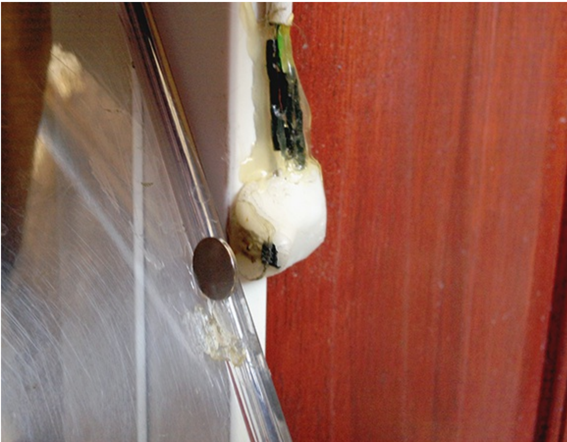
Figure 11-10: Mounting your sensors and magnets.
