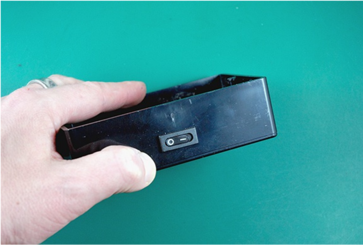
Figure 15-11: Testing the fit of the power switch.
