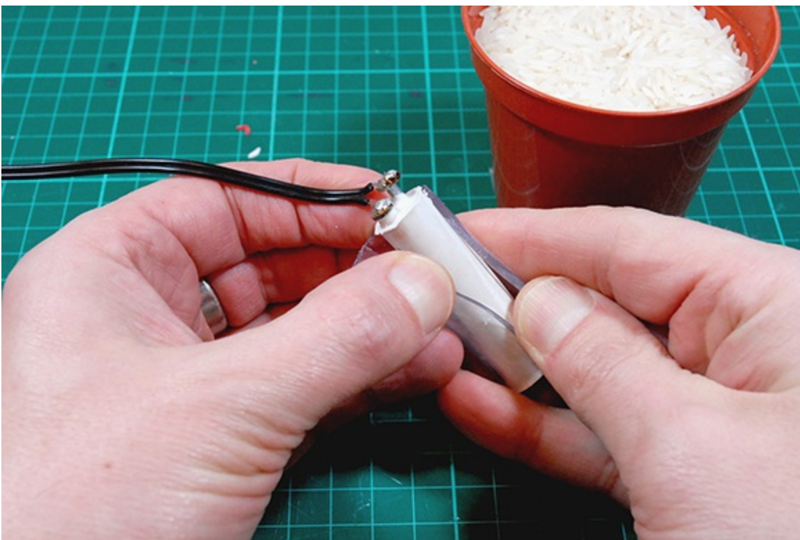
Figure 10-7: Removing your probe from the mold.
