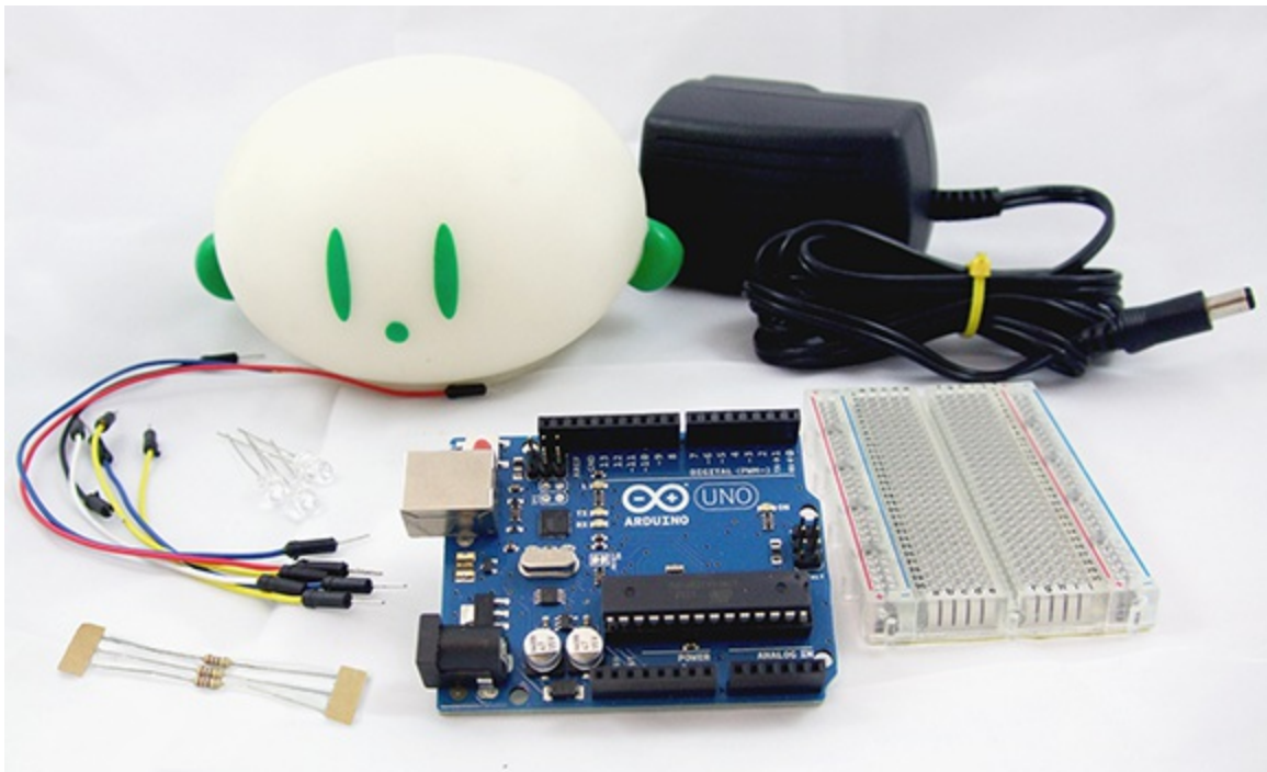
Figure 5-1: All the parts you need for the light pet. Get creative with your enclosure!
