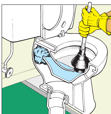
Figure 5-1: Positioning the plunger.
