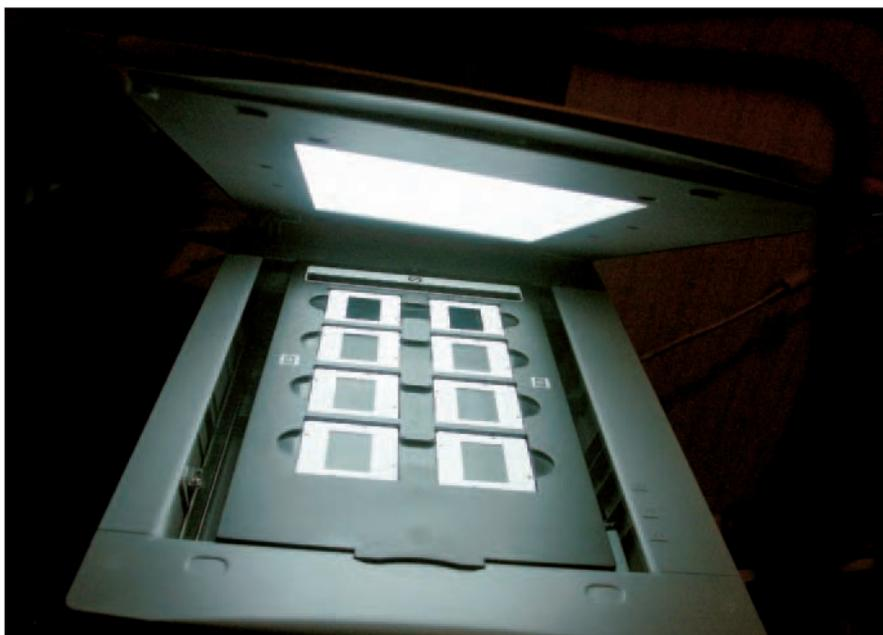
**Figure 4-4:** A flatbed scanner with a light source in its lid can scan film.
