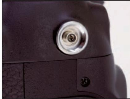
**Figure 2-6:** Your camera may have a connection for plugging in an external flash unit.
