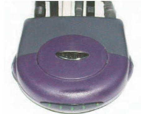
**Figure 3-2:** A powered USB hub allows connecting many different peripherals at once.
