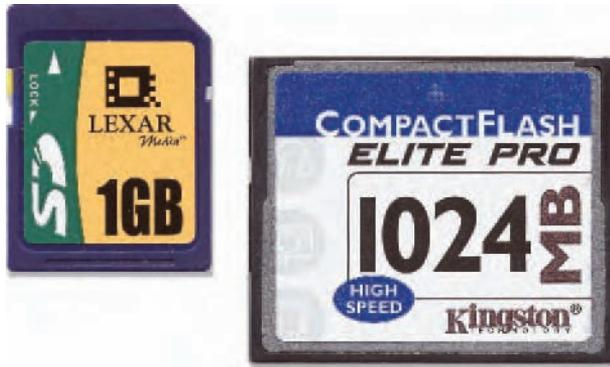
**Figure 3-5:** Secure Digital (left) and CompactFlash (right) are the most popular digital memory card formats.
