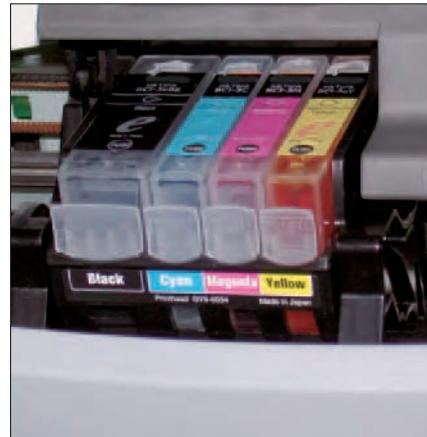
**Figure 4-2:** Using replaceable separate ink tanks is more economical.
