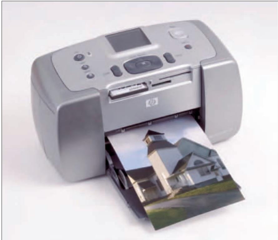
**Figure 1-4:** Plug a memory card into the slot on this printer, choose an image on the built-in LCD, and you can make a print without using a computer.
