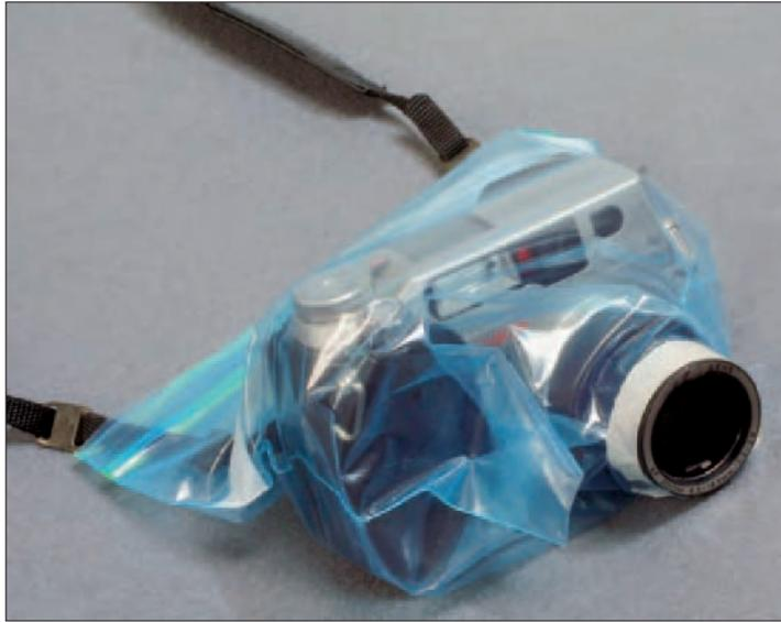
**Figure 6-7:** A zip-closure bag and tape can make a raincoat for your camera.
