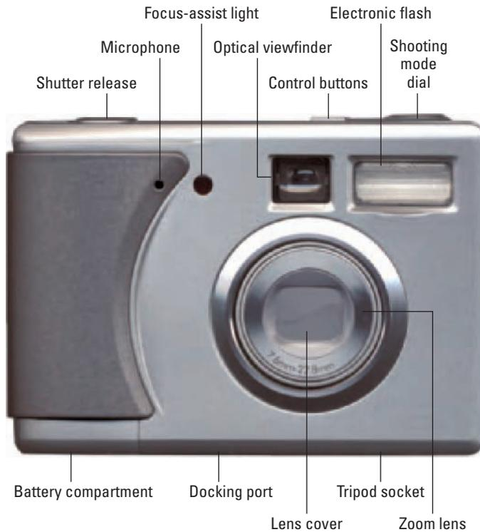
**Figure 1-1:** The front of a typical digital camera.
