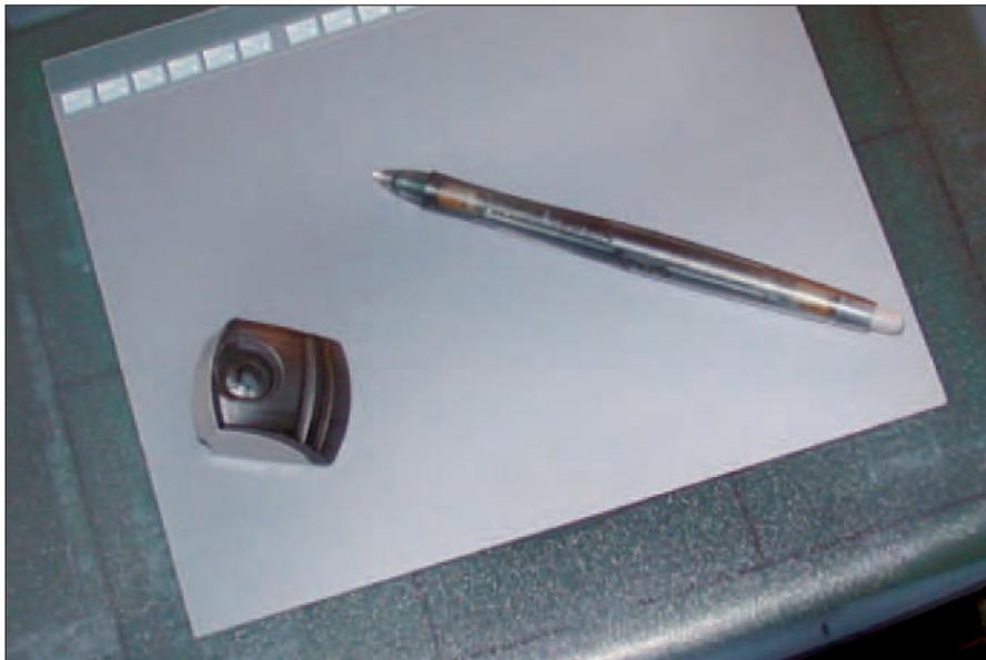
**Figure 2-4:** Digital photos can be edited more precisely with a pressure-sensitive tablet and stylus.
