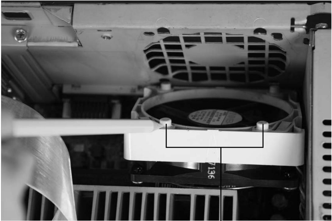
Remove screws or clips that hold the fan in place.
