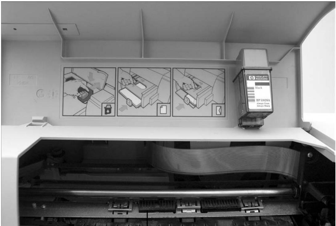
Open your printer case, and follow the directions for replacing cartridges.
