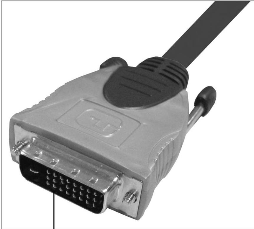
Check for bent or broken pins at both ends of the cable.
