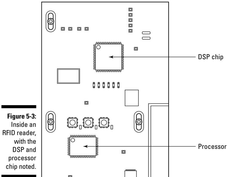
**Figure 5-3:** Inside an RFID reader, with the DSP and processor chip noted.
