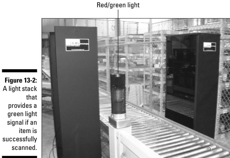
**Figure 13-2:** A light stack that provides a green light signal if an item is successfully scanned.
