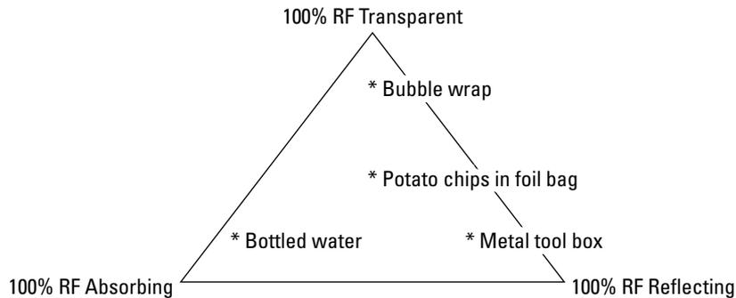
You can also use the pyramid to help you determine the optimal location to begin testing. In a typical case, you should be able to choose the top four or five locations to test based on basic knowledge of the laws of electromagnetism discussed in Chapter 5. If the object you want to tag is made up of many items with various RF properties, you can rate the various parts of the object based on their RF friendliness by using the pyramid.
