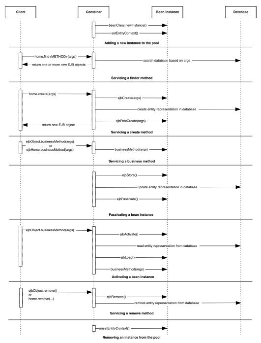
Figure E.12 Sequence diagram for container-managed persistent entity beans. For simplicity, the Container object represents all container subsystems, including EJB objects, home objects, transaction services, and so on.
