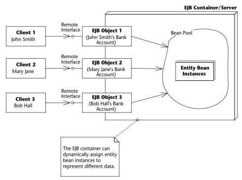
**Figure 6.4** EJB container pooling of entity beans.
