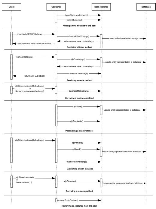
**Figure E.11** Sequence diagram for bean-managed persistent entity beans. For simplicity, the Container object represents all container subsystems, including EJB objects, home objects, transaction services, and so on.
