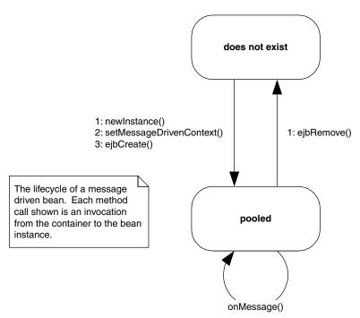
**Figure E.13** The life cycle of a message-driven bean. Each method call shown is an invocation from the container to the bean instance.
