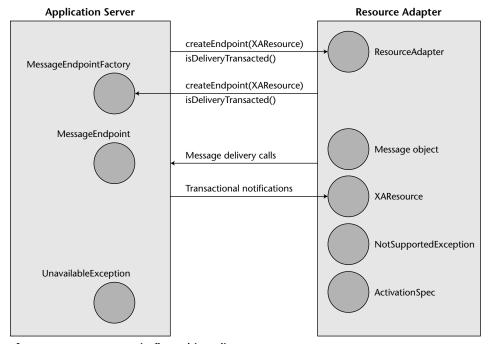
Figure 17.13 Message in-flow object diagram.
