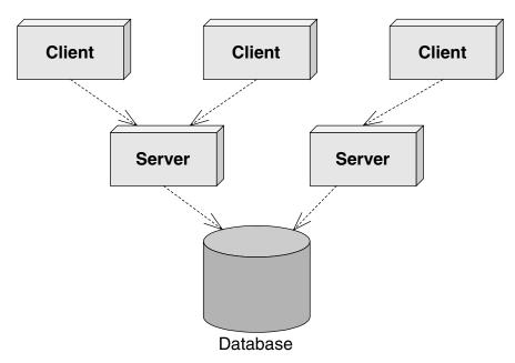
Figure 1.1 Standard multitier-only deployment.
