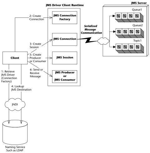
Figure 9.3 Client view of a JMS system.
