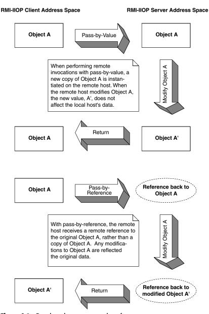
**Figure A.1** Pass-by-value versus pass-by-reference.
