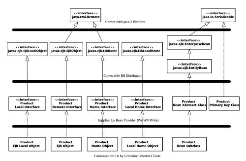
Figure 8.3 The class diagram for the product line example.
