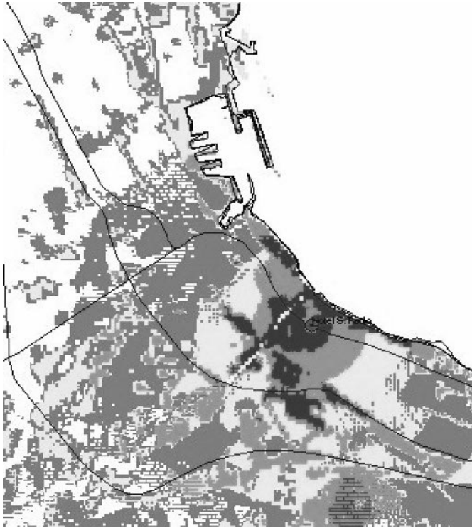
Figure D.9 Prediction of radio coverage offered by a radio base station
