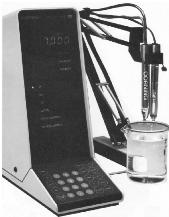
Figure 5.8 A modern microprocessor-controlled pH meter.
