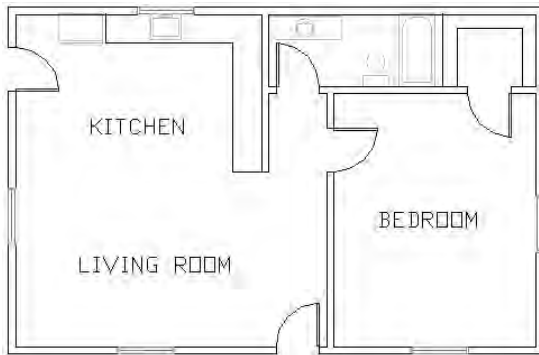
Figure 16-31: A floor plan of an apartment drawn by using multilines
