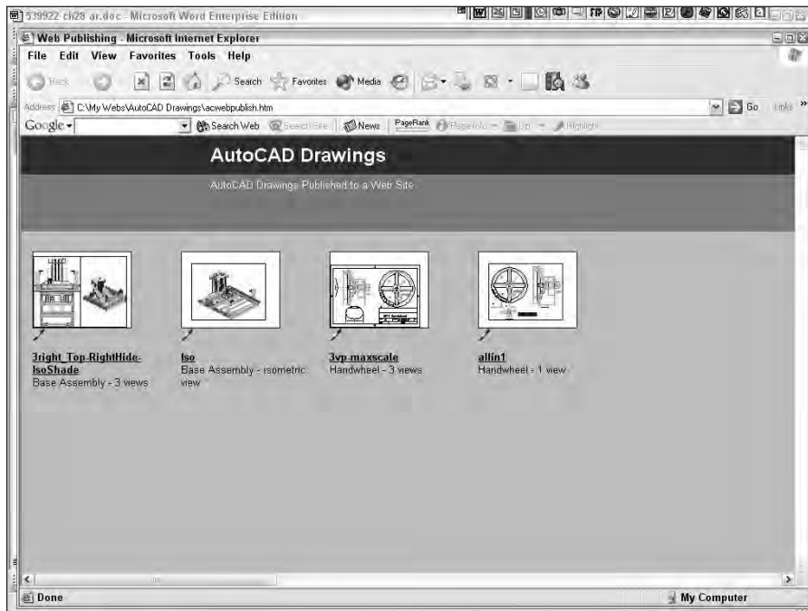
Figure 28-15: A preview of some drawings using the Array of Thumbnails template and DWF files. You can click on any thumbnail to see the full-size DWF file. Note the i-drop icons.
