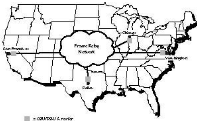
FIGURE 2.3 A private network using a frame-relay net.
