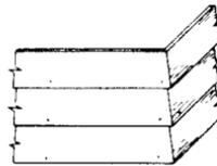
**Figure 16-12** The mitered corner treatment.
