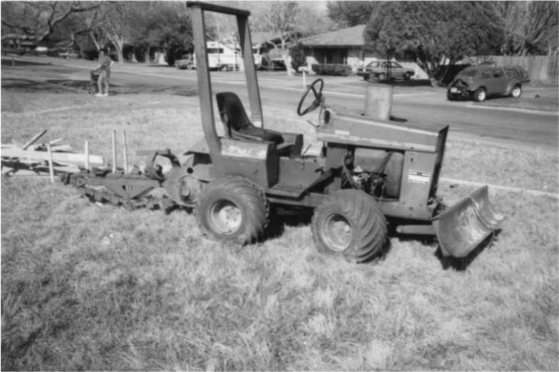
**Figure 2-13 Tractor with trencher attached.**
