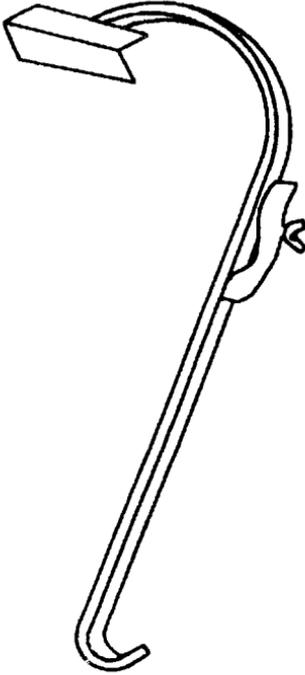
**Figure 4-18 Ladder hook.** (Courtesy of Waco Scaffolding and Equipment)
