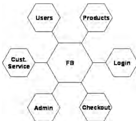
Figure 37-1: The Fusebox architecture as a hub-and-spoke arrangement.
