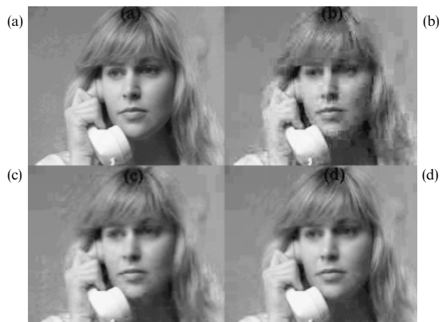
Figure 2.23 (a) 150th frame of original Suzie sequence, its compressed version at 64 kbit/s and 25 f/s; (b) H.261; (c) H.263 default mode; (d) H.263 with four negotiable options
