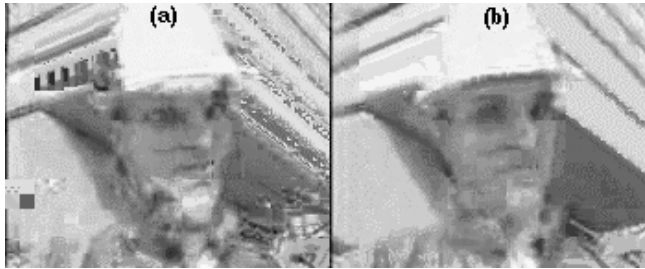
Figure 4.18 One hundred and ninety-ninth frame of H.263 coded Foreman sequence at 64 kbit/s and transmitted over a channel with random errors at \text{BER} = 10^{-5} : (a) ordinary H.263 stream, (b) H.263 stream with duplicated MV data sent on a GOB-level
