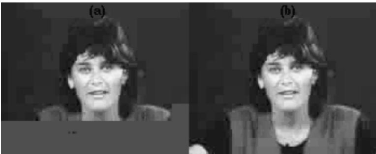
Figure 4.25 The first frame of QCIF Miss America sequence encoded with H.263 at 47 kbit/s, 1.2 I-f/s, BER = 10 -4 : (a) ordinary H.263, (b) robust I-frame coding
