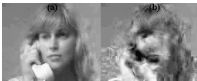
Figure 3.16 Frame 150 of the Suzie sequence encoded with H.263 at 55 kbit/s and subject to 5 per cent information drop: (a) on the sub-stream of DCT coefficients of a P-frame, (b) on the MV sub-stream
