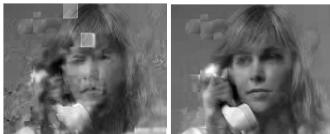
Figure 4.10 One-hundred-and-fiftieth frame of QCIF-size Suzie sequence coded with MPEG-4 at 64 kbit/s: (a) without error resilience, (b) data partitioning + UEP
