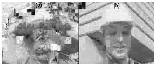
Figure 4.16 One hundred and twenty-fifth frame of the Foreman sequence encoded with H.263 at 64 kbit/s and transmitted over an AWGN channel of SNR = 12 dB: (a) ordinary H.263 stream, (b) H.263 with MB-level duplicated MV data
