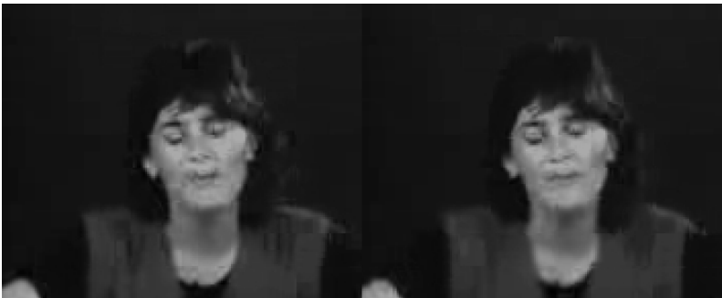
Figure 3.9 Frame of the Miss America sequence encoded at 14.4kbit/s: (a) conventional variable-Qp TMN5 rate control, (b) ROI coding for enhanced-face rate control
