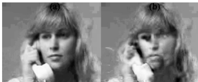
Figure 3.14 Frame 150 of the Suzie sequence encoded with H.263 at 55 kbit/s: (a) error-free, (b) subject to 5 per cent drop rate of MV and AC coefficients of P-frames due to network congestion
