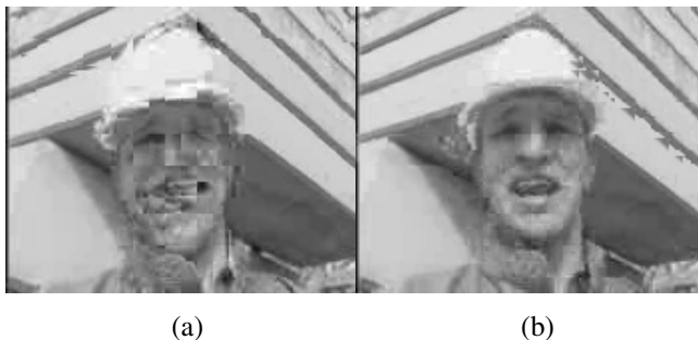
Figure 5.20 A frame extracted from the Foreman sequence coded with MPEG-4 at 32 kbit/s and 5 f/s and transmitted over GPRS at C/I = 12 dB using CS-1 and five time slots: (a) no error resilience, (b) full error resilience
