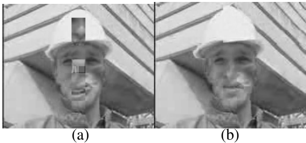
Figure 4.14 Seventy-fifth frame of the Foreman sequence encoded with MPEG-4 and sent over a mobile channel of BER = 3 \times 10^{-4} : (a) without CRCs (variance = 3.00 dB), (b) with CRCs (variance = 0.08 dB)
