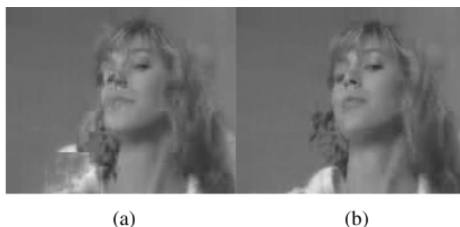
Figure 4.44 Fifty-sixth frame of the Suzie sequence coded at 25f/s, after frame 55 was fully dropped during transmission: (a) non-error-resilient case at 57 kbit/s, (b) RPS ACK mode with a delay of 2 frames at 60.5 kbit/s
