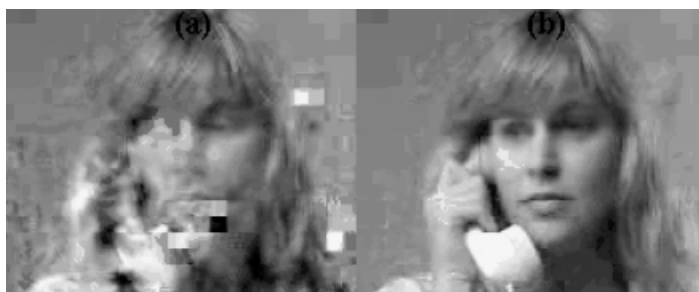
Figure 4.11 One-hundredth frame of H.263 coded Suzie sequence at 64 kbit/s with the MV stream transmitted over an AWGN channel of SNR = 12.5 dB: (a) no FEC protection, (b) MVs protected with a one-half rate convolutional coder
