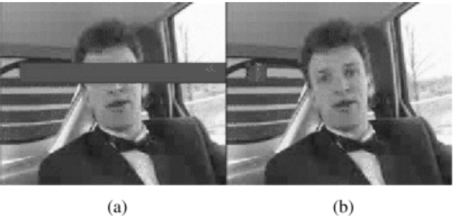
Figure 4.32 One frame of the Carphone sequence coded with H.263 at 28 kbit/s and 12.5 f/s using: (a) ordinary decoding, (b) two-way decoding
