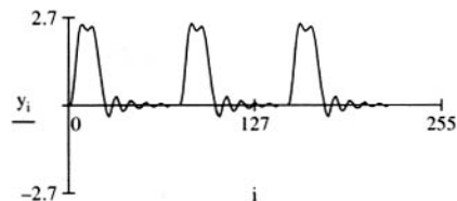
Figure 4.14 Convolution example. The dynamic response at the support of a belt conveyor
