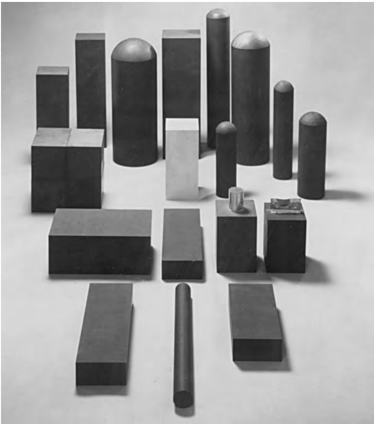
Fig. 4.3 Isostatically pressed tin oxide electrodes for producing high quality glasses; the length of the longest electrode in the illustration is approximately 500 mm. (The contacting stubs may be wrapped with silver foil to reduce resistance.) (Courtesy of Dyson Technical Ceramics.)
