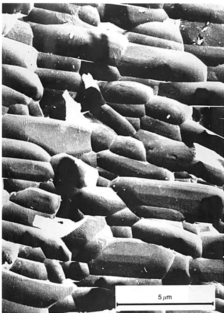
Fig. 9.33 Microstructure of an oriented barium hexaferrite. (Courtesy of Philips Technical Review.)
