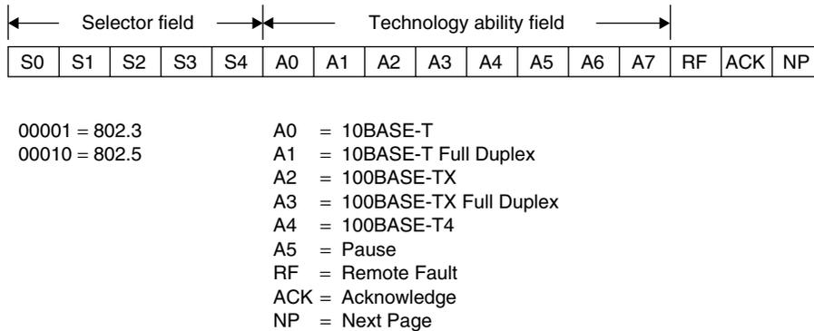
**Figure 3.38** The format of the link code word.
