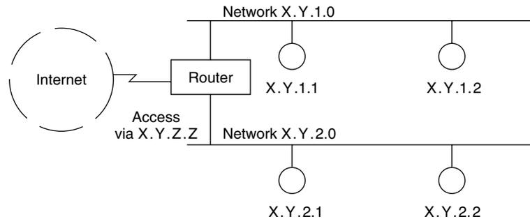
**Figure 5.41** A Class B network address location with two physical networks using subnet addressing. IP datagrams with the destination address  $X.Y.Z.Z$ , where  $Z$  can be any decimal value representing a Class B network address that can consist of 256 subnets, with 256 hosts on each subnet.
