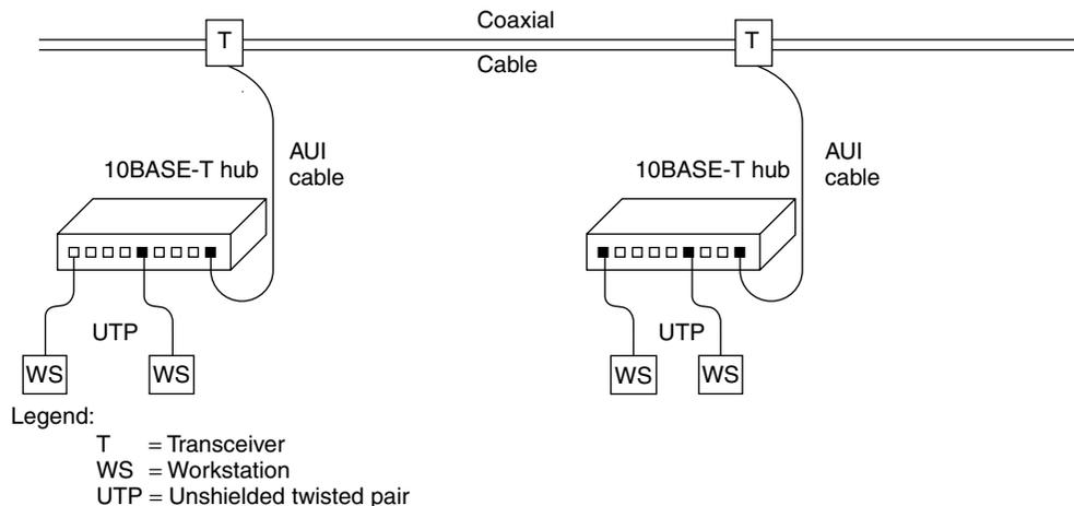
**Figure 3.7** Using 10BASE-5 as a backbone. The use of 10BASE-5 as a backbone enables 10BASE-T hubs to be located further from one another than if they were wired together using unshielded twisted-pair cable.
