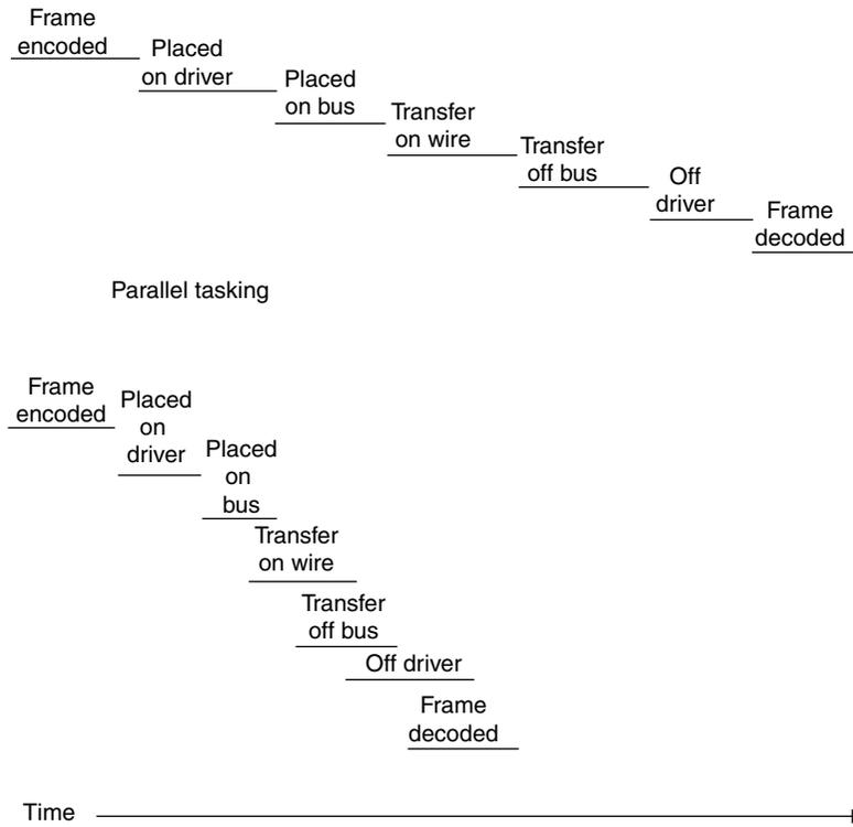
**Figure 11.6** Serial-tasking versus parallel-tasking Ethernet adapters. The use of parallel-tasking Ethernet adapter cards permits the overlapping of many operations, thus reducing the time needed to transfer information and increasing the data transfer capability of the adapter.
