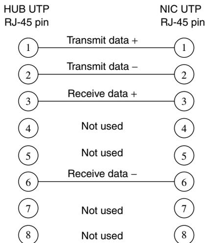
**Figure 3.19** 10BASE-T hub to NIC wiring.
