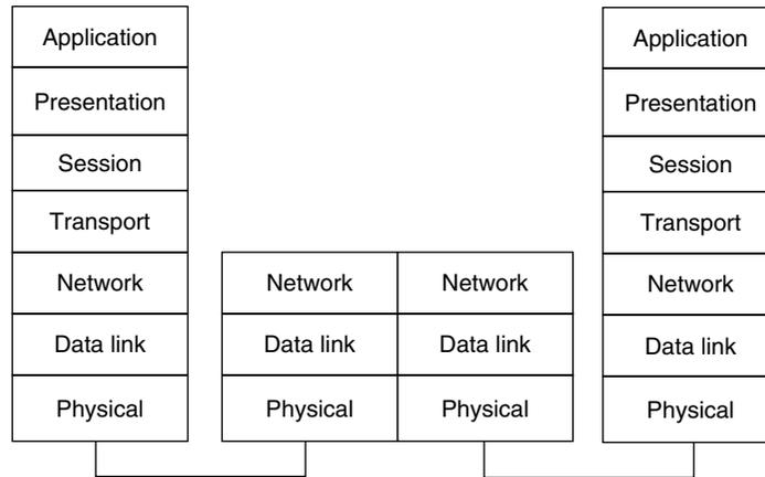
**Figure 5.9** Router operation. A router operates at the network layer of the ISO OSI Reference Model. This enables a router to provide network layer services, such as flow control and frame fragmentation.
