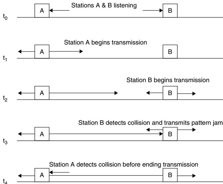
**Figure 4.6** Collision detection.
