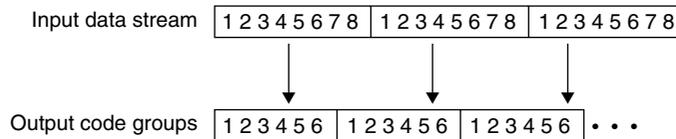
**Figure 3.32** 8B6T coding process.
