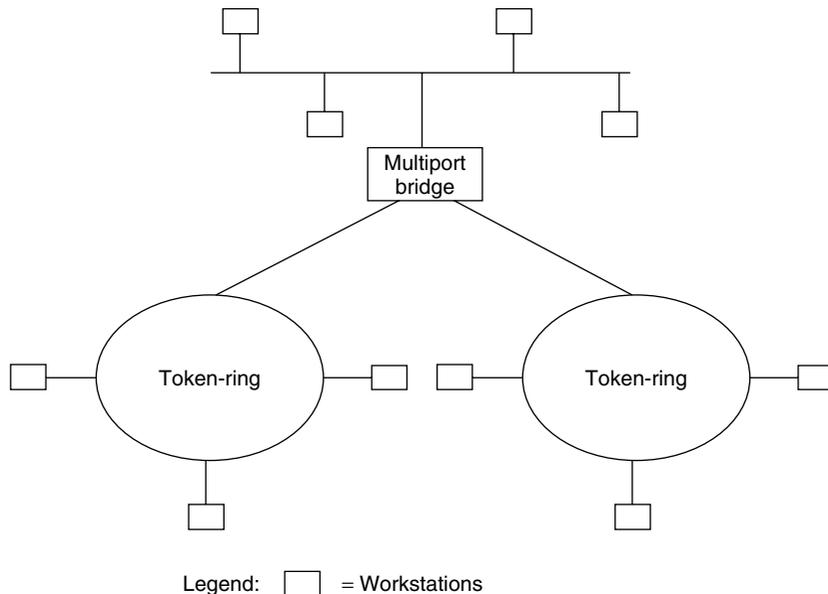
**Figure 5.7** Using a multiport bridge. With a multiport bridge, you can interconnect three or more local area networks.
