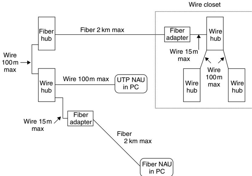
**Figure 3.22** 10BASE-T and FOIRL transmission distance limits.
