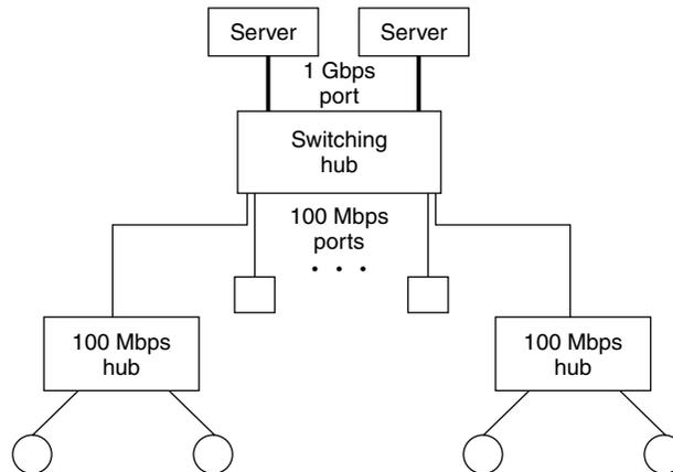
In a switch environment each 1-Gbps port can provide a full-duplex 2-Gbps data transfer capability.
