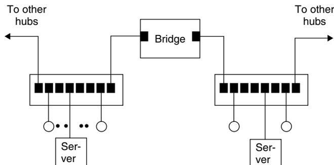
**Figure 6.17** Using a bridge for network segmentation. The use of a bridge and one or more servers on each interconnected segment can significantly increase network capacity by localizing more traffic on each segment.
