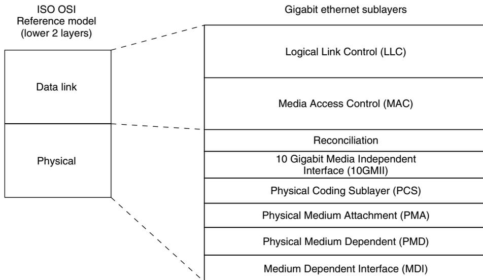
**Figure 3.53** 10 Gigabit Ethernet architecture.
