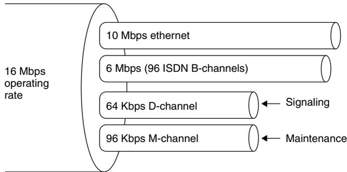
**Figure 3.25** Allocation of isoENET bandwidth.
