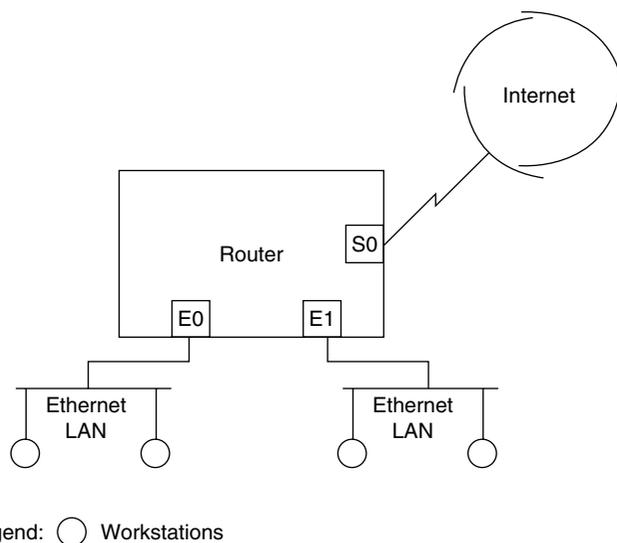
**Figure 9.6** A sample network to be used for illustrating the configuration and operation of Context-Based Access Control (CBAC).
