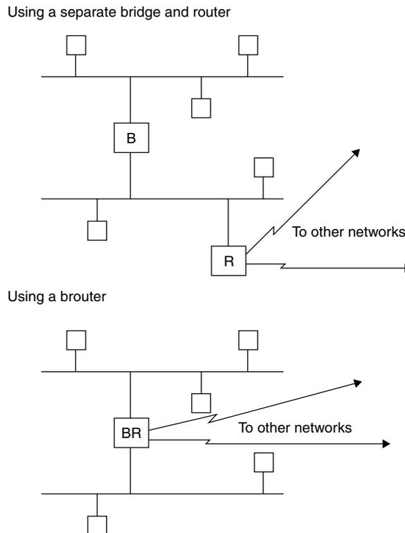
**Figure 5.12** Replacing a separate bridge and router with a brouter.
