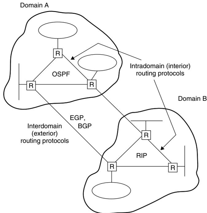
**Figure 7.9** Interior and exterior routing protocols. An interior routing protocol controls the flow of information within a collection of interconnected networks known as a *domain*. An exterior routing protocol provides routers with the ability to determine what networks on other domains they can reach.
