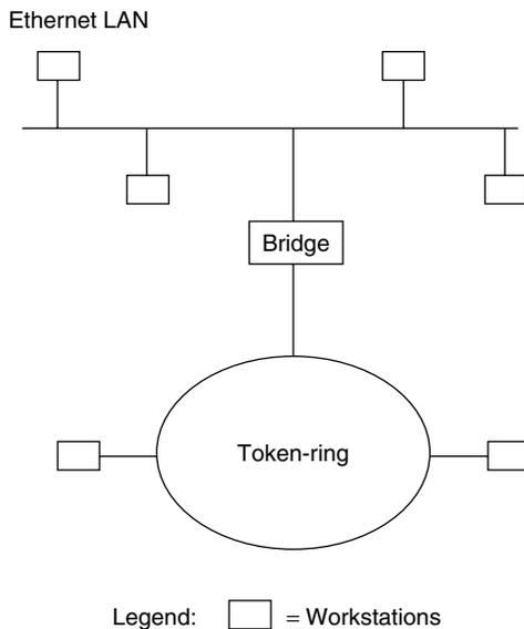
**Figure 5.5** Translating bridge operation. A translating bridge connects local area networks that employ different protocols at the data link layer. In this example, the translating bridge is used to connect an Ethernet local area network to a Token-Ring network.
