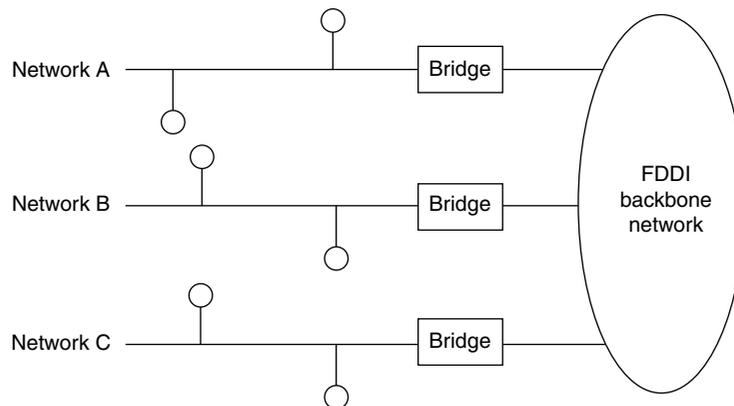
**Figure 11.3** Using a high-speed backbone network. The use of a 100-Mbps FDDI network as a backbone to connect separate Ethernet LANs can remove a large degree of potential internet congestion while permitting the previous investment in Ethernet networks to be maintained.
