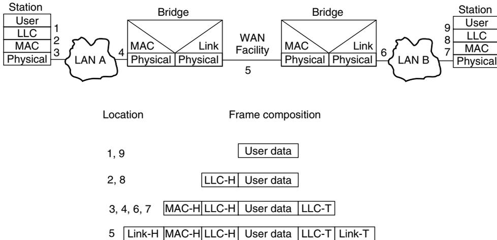
**Figure 5.8** Remote bridge operation. A remote bridge wraps the logical link control (LLC) and media access control (MAC) frames in another protocol for transmission over a wide area network.
