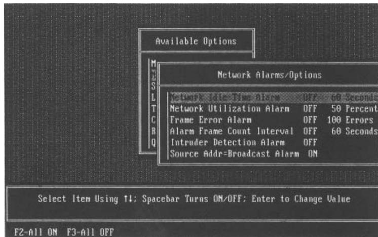
**Figure 10.11** EtherVision network alarms/options screen.
