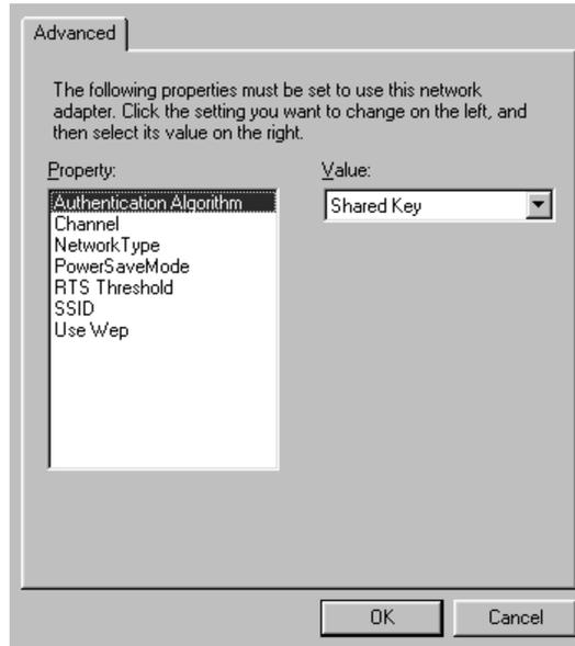
**Figure 8.22** The SMC networks advanced client setup screen provides users with the ability to modify the settings for seven properties.
