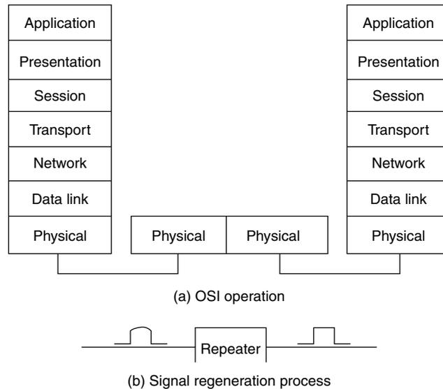
**Figure 5.1** Repeater operation. A repeater connects two local area networks or network segments at the OSI physical layer (cable) by regenerating the signal received on one LAN or LAN segment onto the other network or network segment.
