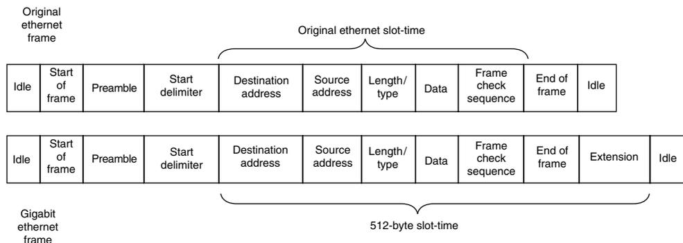
**Figure 4.15** Half-duplex Gigabit Ethernet uses a carrier extension scheme to extend timing so that the slot time consists of at least 512 bytes.
