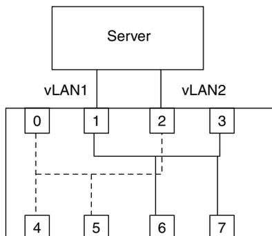
**Figure 6.32** Overcoming the port-based constraint where stations can only join a single vLAN. By installing multiple network adapter cards in a server or workstation, a LAN device can become a member of multiple vLANs.
