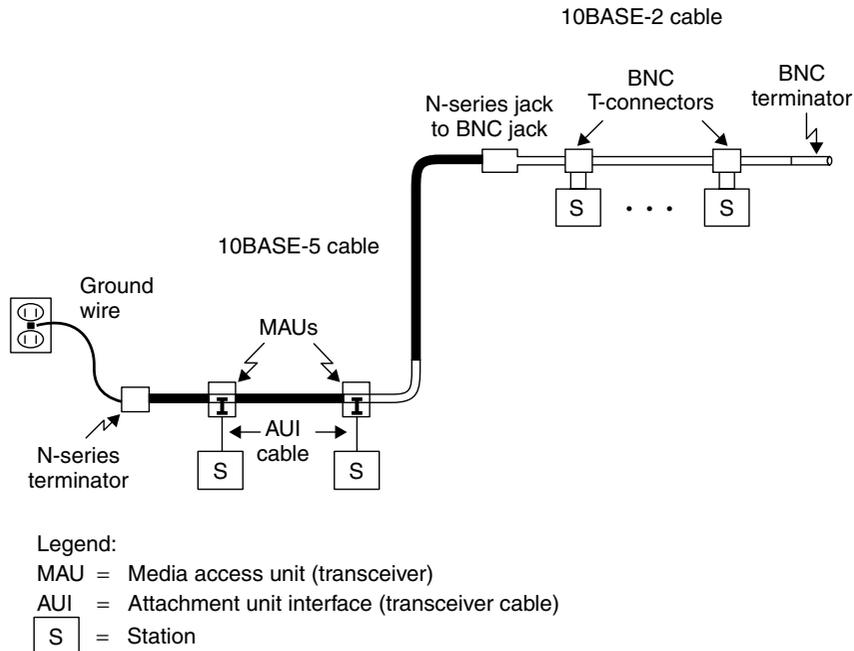
**Figure 3.13** Combined 10BASE-5 and 10BASE-2 cable segment. A combined thick and thin coaxial segment can be used to economically connect a group of stations clustered in one area of a building to a few stations located a relatively long distance away from the cluster.
