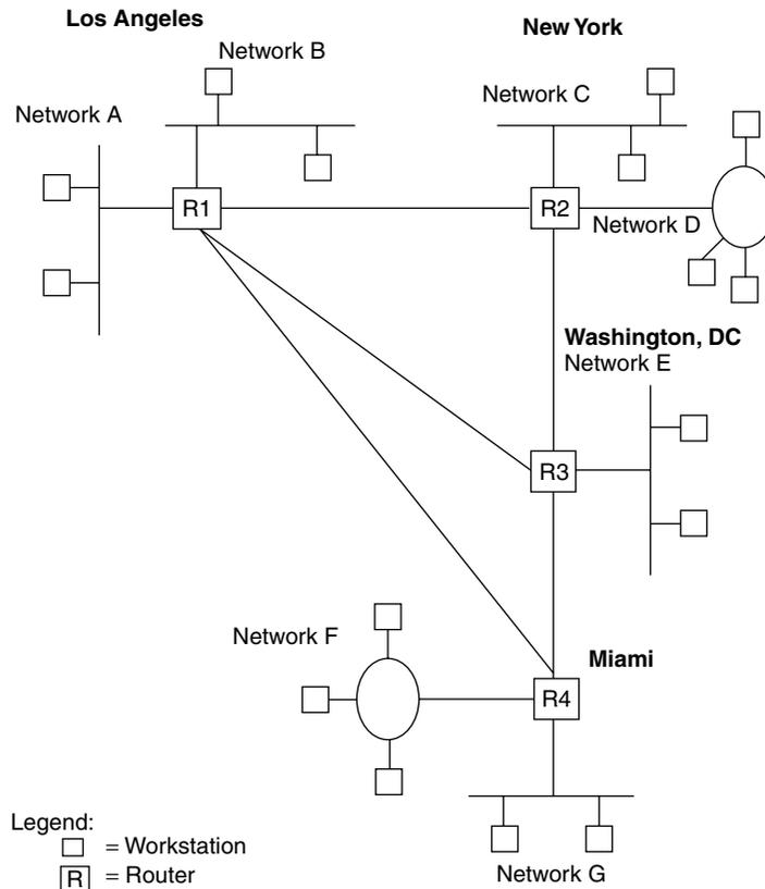
**Figure 5.11** Building an internet using routers. Routers can be used to establish complex networks in which traffic is varied over network facilities. This variation is based on the operational status and utilization of different network paths.
