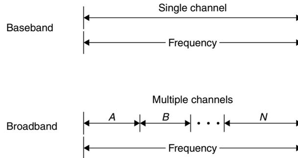
**Figure 1.5** Baseband versus broadband signaling. In baseband signaling the entire frequency bandwidth is used for one channel. In comparison, in broadband signaling the channel is subdivided by frequency into many subchannels.
