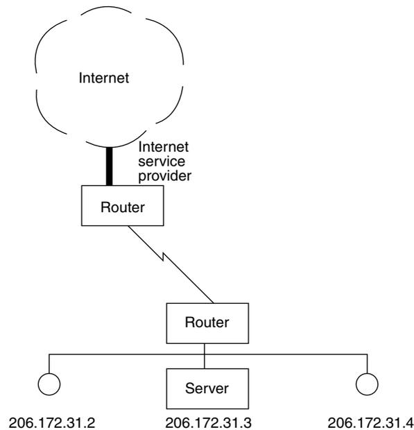
**Figure 7.20** Connecting a corporate LAN to the Internet exposes each corporate computer to a virtually unlimited number of hackers. Through programming router access lists this exposure can be minimized.
