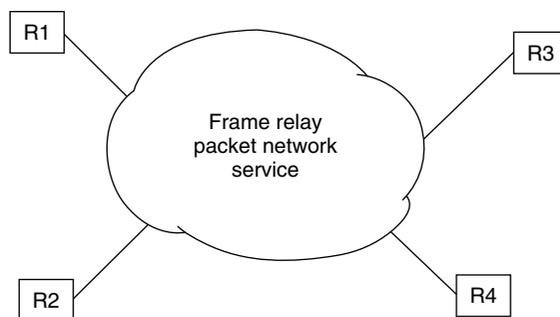
**Figure 7.6** Using a frame relay service. If a frame relay service is used, the packet network provides the capability for interconnecting each network access port to other network access ports. Thus, only one router port is required to obtain an interconnection capability to numerous routers connected to the network.
