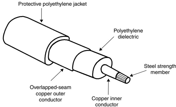
**Figure 1.8** Coaxial cable.
