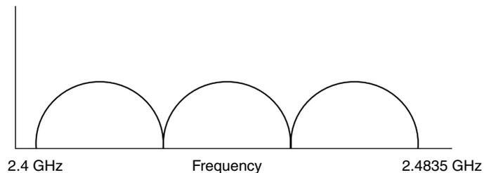
**Figure 8.6** DSSS supports up to three non-overlapping channels in the 2.4 GHz band.
