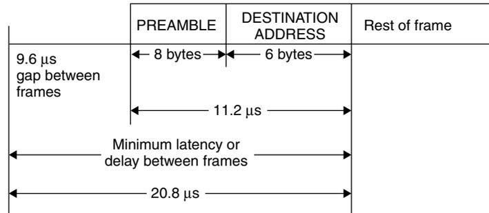
**Figure 6.29** Switch latency includes a built-in delay resulting from the structure of the Ethernet frame.
