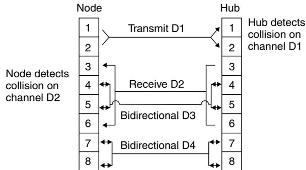
Figure 3.29 100BASE-T4 pin assignments.
