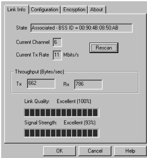
**Figure 8.23** The utility program provided with SMC networks wireless PC cards provides a mechanism to monitor link quality and signal strength.
