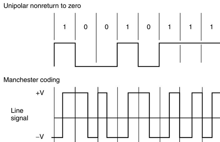
**Figure 1.7** Unipolar nonreturn to zero signaling and Manchester coding. In Manchester coding, a timing transition occurs in the middle of each bit and the line code maintains an equal amount of positive and negative voltage.
