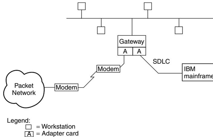
**Figure 5.14** Multiprotocol gateway operation. A multiprotocol gateway can be used to provide local area network stations access to different computational facilities, either directly or through the use of a packet network.
