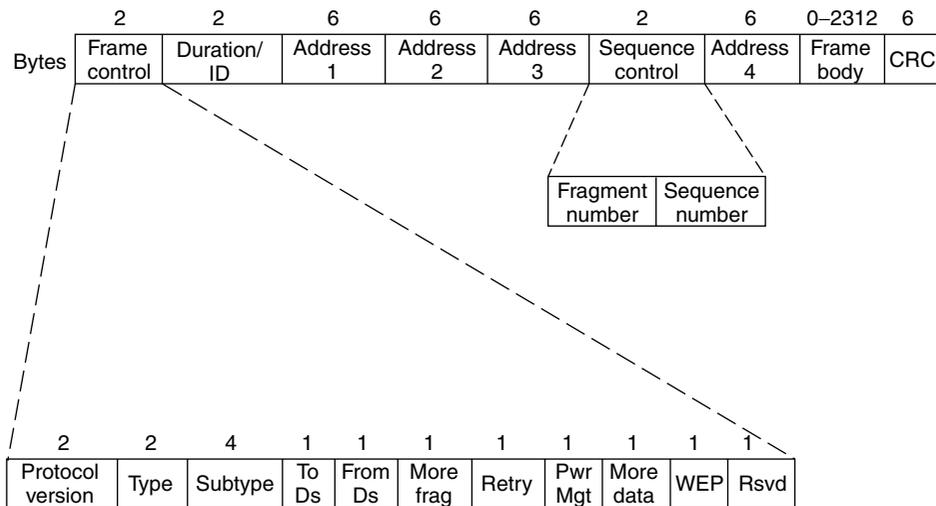
**Figure 8.9** The basic 802.11 MAC data frame format.
