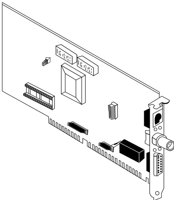
**Figure 3.15** Multiple-media network interface card. Some multiple-media network interface cards, such as the one illustrated, support the direct attachment to UTP and thin coaxial cable, while the DB-15 connector permits the card to be cabled to an MAU connected to thick coaxial cable.
