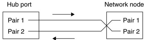
**Figure 3.33** 100BASE-TX cabling.
