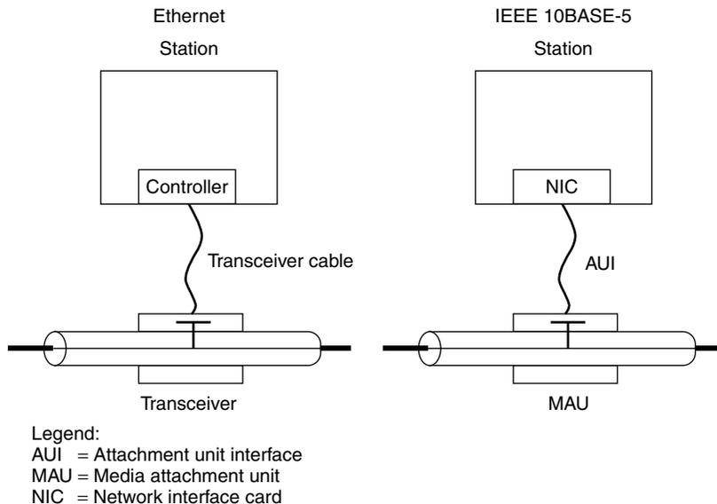
**Figure 3.6** Ethernet and 10BASE-5 media interface differences. Terminology changes under the IEEE 10BASE-5 standard resulted in the transceiver being called the *media attachment unit*, while the transceiver cable is known as the *attachment unit interface*.
