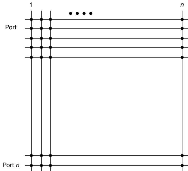
**Figure 6.26** The key to the operation of a switch is a matrix module which enables each port to be cross-connected to other ports. The matrix module of a switch with  $n$  ports can be considered to represent an  $n \times n$  star-wired backplane.
