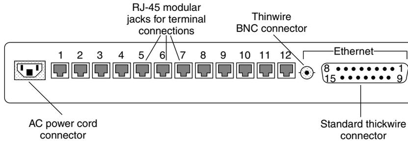
**Figure 3.17** 10BASE-T hub connectors. In addition to 8, 10, or 12 RJ-45 modular jacks for terminal connections, most 10BASE-T hubs contain a BNC and DB-15 port to permit attachment to thin and thick backbone networks.
