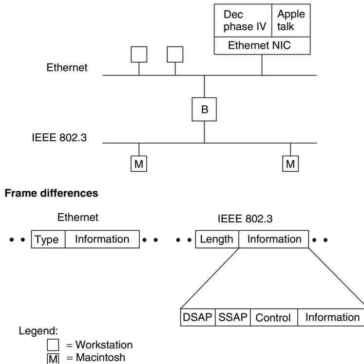
**Figure 6.6** Protocol differences preclude linking IEEE 802.3 and Ethernet networks using transparent bridges. A Macintosh computer connected on an IEEE 802.3 network using AppleTalk will not have its frame pointed to the right process on a VAX on an Ethernet. Thus, the differences between Ethernet and IEEE 802.3 networks require transparent bridges for interconnecting similar networks.
