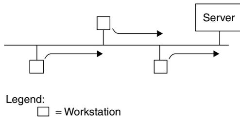
**Figure 5.16** Server placement. The location of a server on a network is critical for ensuring network performance. In this example, because each workstation requires access to the server, its location requires the greatest transmission distance between individual workstations and the server. This, therefore, is probably a poor server location.
