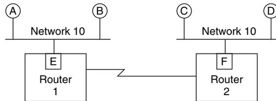
**Figure 5.10** Routing between two networks. When a workstation on one network transmits data to a device on another network, an application program provides the destination network address, which is used by routers as a basis for their routing decisions.
