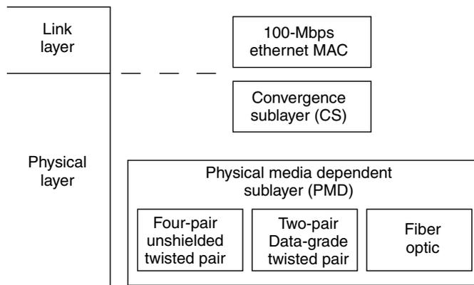
**Figure 3.27** Fast Ethernet physical layering subdivision overview.
