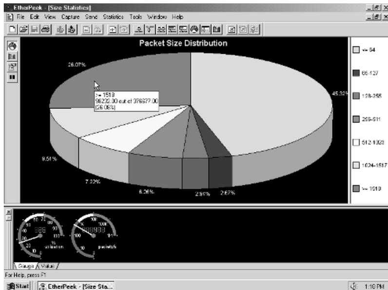
Figure 10.25 Displaying packet size distribution information.
