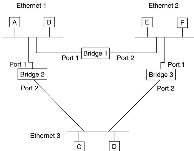
**Figure 6.2** Transparent bridges do not support network loops. The construction of a circular or loop topology with transparent bridges can result in an unnecessary duplication of frames, and may confuse end stations. To avoid these problems, the Spanning Tree Protocol (STP) opens a loop by placing one bridge in a standby mode of operation.
