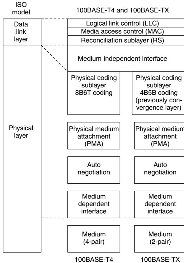
Figure 3.28 100BASE-T4 versus 100BASE-TX physical and link layers.
