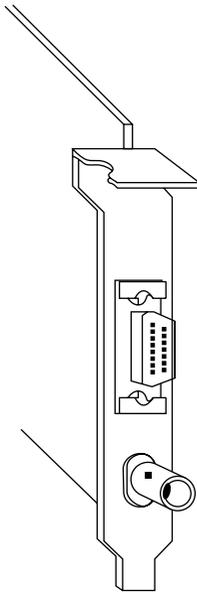
**Figure 3.2** Ethernet interface board connectors. The first generation Ethernet interface boards (network interface cards) contain both DB-15 and BNC connectors to support the use of either thick or thin coaxial cable. A second generation of interface cards included an RJ-45 connector to Accommodate a connection to twisted-wire-based networks.
