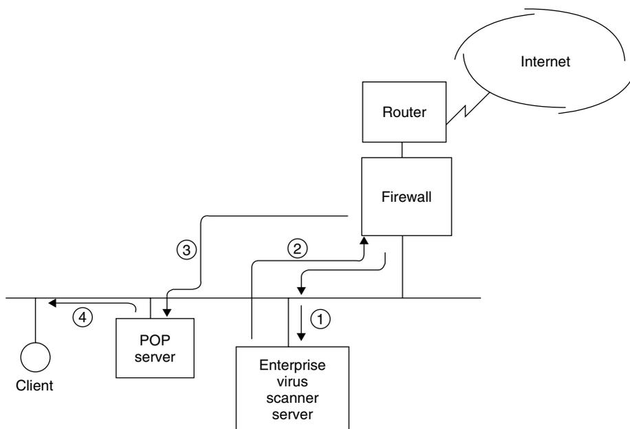
**Figure 9.28** Using an enterprise virus scanner server.
