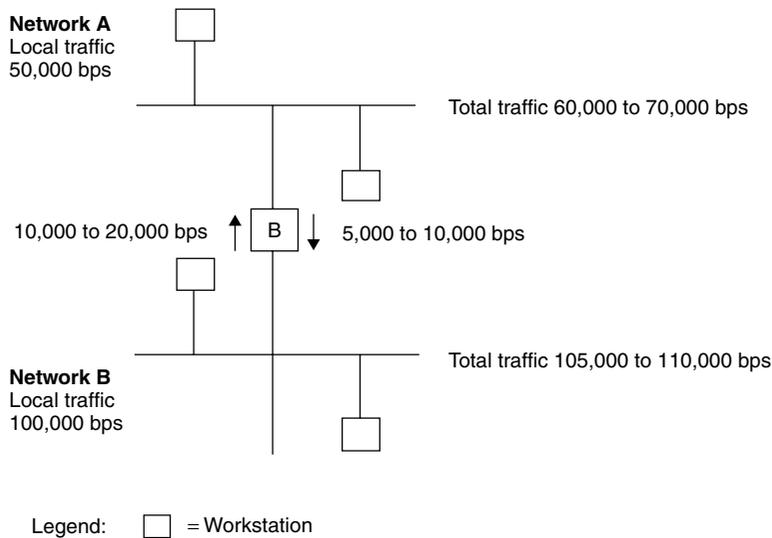
**Figure 6.13** Considering intranet data flow. To determine the traffic flow on separate networks after they are interconnected, you must consider the flow of data onto each network from the other network.
