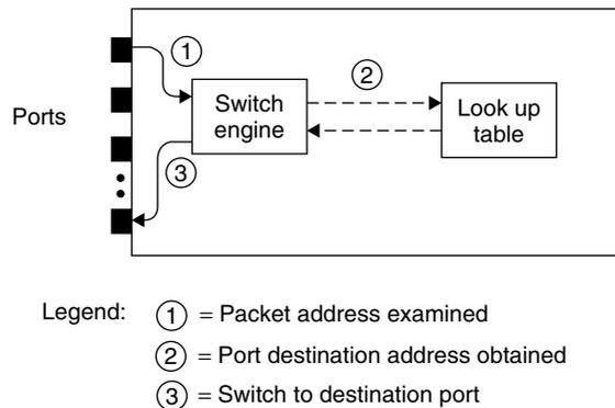
**Figure 6.19** Cross-point/cut-through switching.
