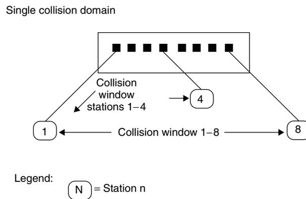
**Figure 4.14** Relationship between a collision domain and collision windows.
