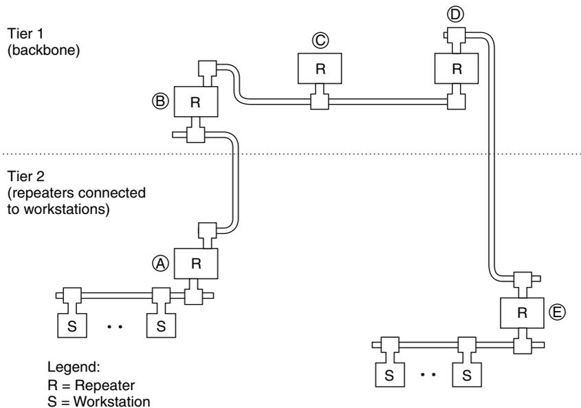
**Figure 3.12** Two-tier thin Ethernet 10BASE-2 network. A two-tier network permits expansion of a 10BASE-2 network by adding another level of repeaters to the backbone. The segment between repeaters B, C, and D is considered to be populated, because repeater C is counted as one connection on the segment.
