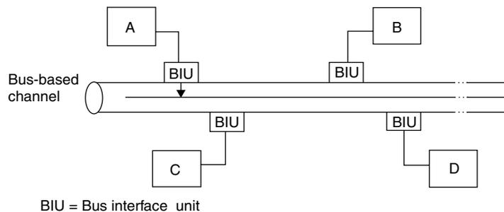
**Figure 1.11** CSMA/CD network operation. In a CSMA/CD network, as the distance between workstations increases, the resulting increase in propagation delay time increases the probability of collisions.
