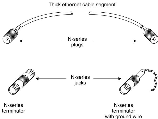
**Figure 3.3** Each Ethernet thick coaxial cable segment has N-series plugs on each end. They are terminated through the use of N-series terminators, one of which contains a ground wire or ground wire connection.
