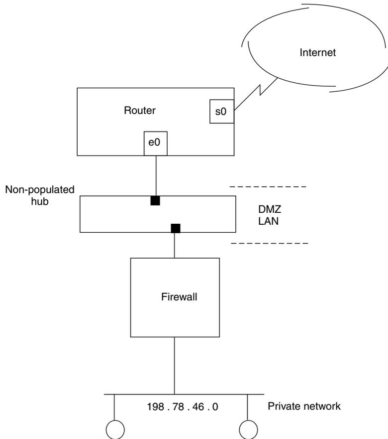
**Figure 9.8** Using a firewall to protect a private network.
