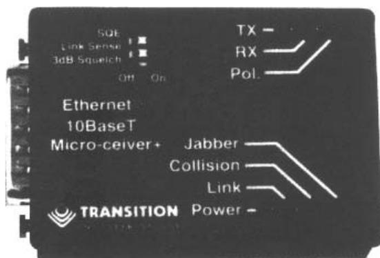
**Figure 3.16** Transition Engineering 10BASE-T transceiver. With a 10BASE-T transceiver, you can connect existing thick or thin 10BASE-5 or 10BASE-2 NICs to a 10BASE-T network. (Photograph courtesy of Transition Engineering, Inc.)
