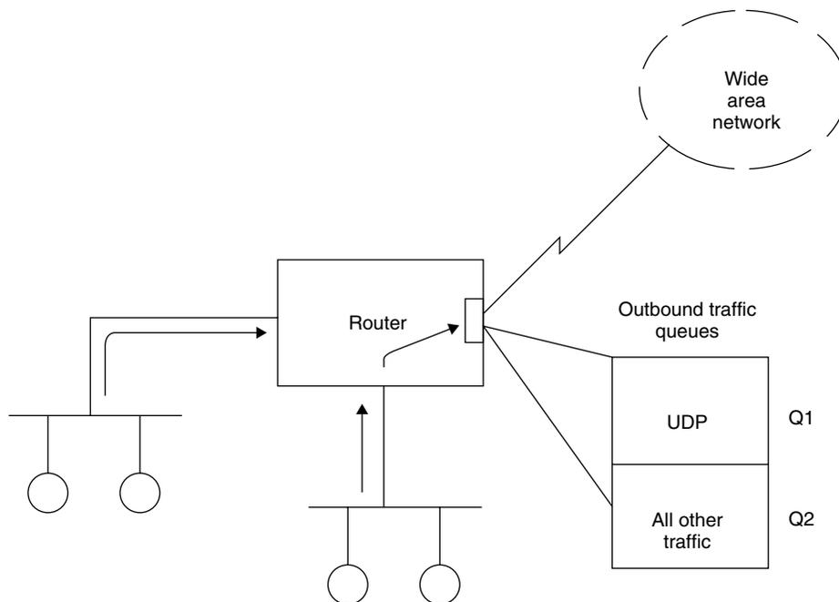
**Figure 7.18** Using an outbound filter to prioritize UDP traffic with a predefined destination port.
