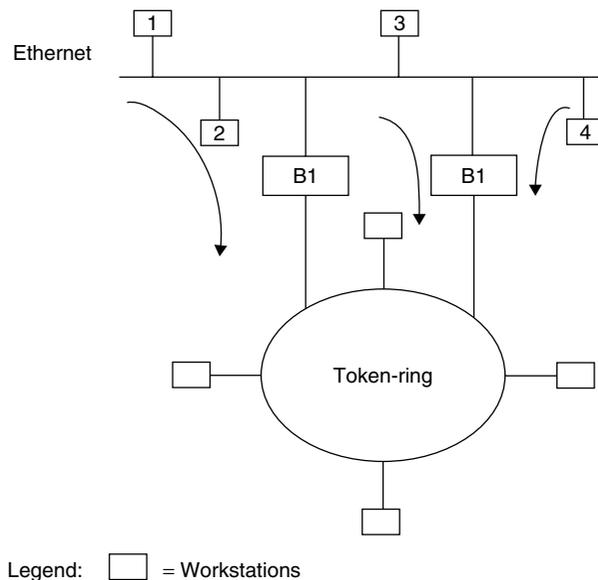
**Figure 5.6** Using bridge selective forwarding capability. Using the selective forwarding capability of bridges enables the data flow between networks to be distributed based upon source or destination addresses.
