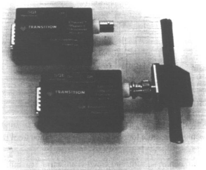
**Figure 3.10** Universal Ethernet Transceiver. The Universal Ethernet Transceiver manufactured by Transition Engineering of Edina, Minnesota, supports both 10BASE-2 and 10BASE-5 coaxial cable connections. (Photograph courtesy of Transition Engineering, Inc.)
