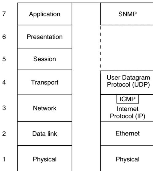
**Figure 10.1** Relationship of SNMP protocol elements to Ethernet.
