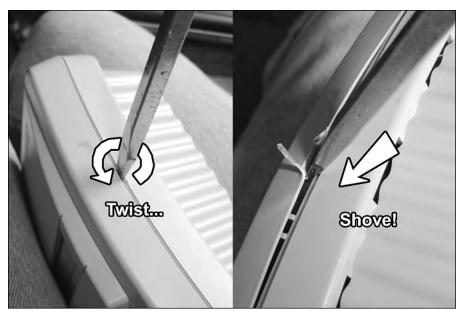
FIGURE 9-2: The screwdriver begins its attack on the mini-SNES.
