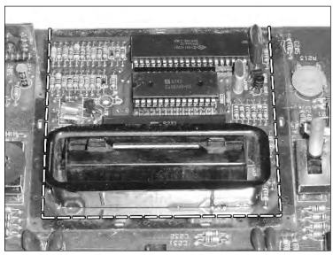
FIGURE 15-4: Where to cut the Atari 2600 board.
