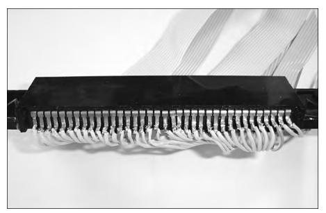
FIGURE 8-15: The second row of pins, with the wires tucked under the connector.
