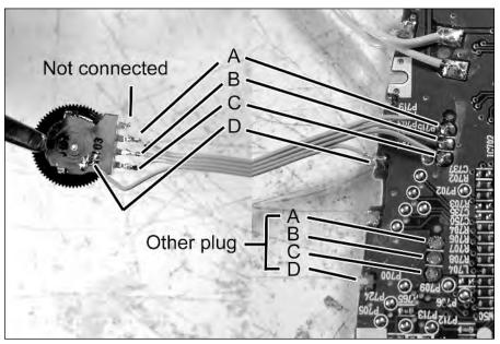
FIGURE 4-15: Reconnecting a knob. Bend out the pins on the knob as shown, using your tweezers for best results.
