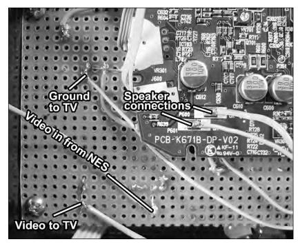
FIGURE 8-35: Connecting the TV to the control board.
