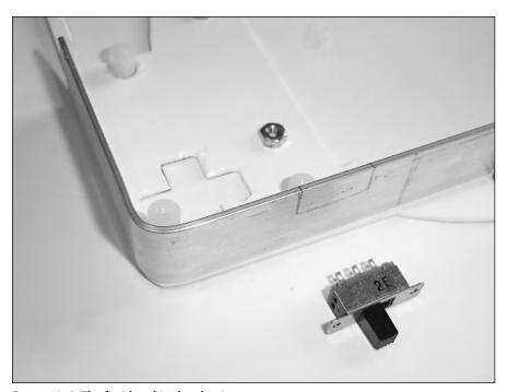
FIGURE 10-6: The first bend in the aluminum.
