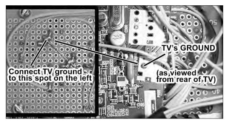
FIGURE 11-28: Connecting the TV's ground to the control board. Also shows the audio/video spots.
