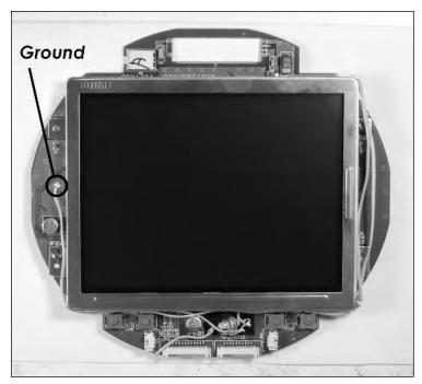
FIGURE 4-29: The completed LED mod, with ground spot indicated.
