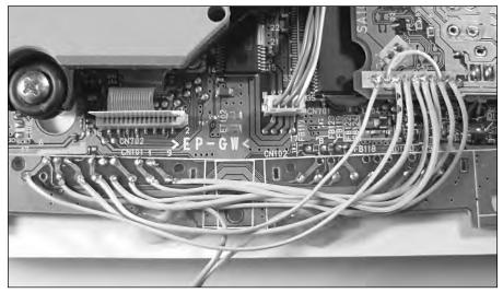
FIGURE 13-32: How to situate the wires going from the PSOne board to the controller board.
