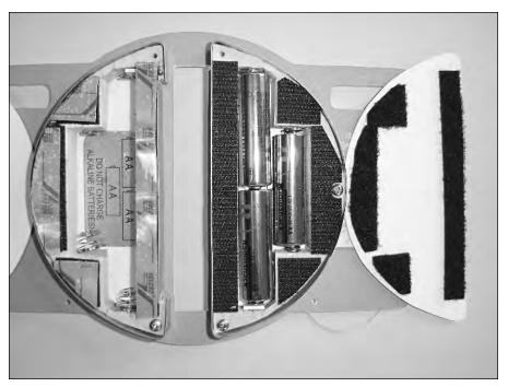
FIGURE 10-18: Velcro placement on the battery compartments and covers.
