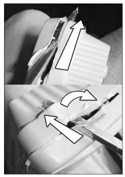
FIGURE 9-3: Separating the case further, and popping a section of plastic.
