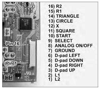
FIGURE 12-9: Button connector pinout.
