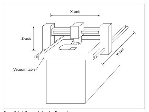
FIGURE 5-1: A three-axis freestanding router.
