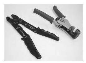
FIGURE 2-25: Two kinds of multigauge wire strippers.
