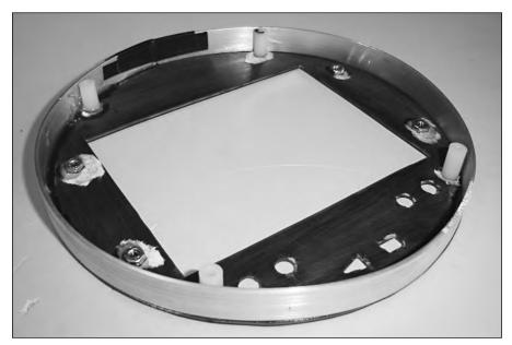
FIGURE 13-5: The front screen plate and aluminum wall thus far.
