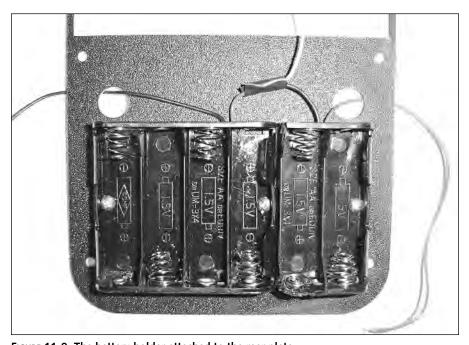
FIGURE 11-9: The battery holder attached to the rear plate.
