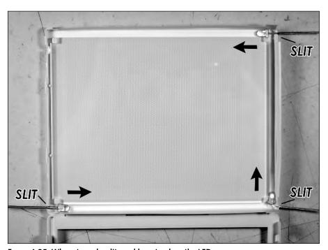
FIGURE 4-25: Where to make slits and how to place the LEDs.
