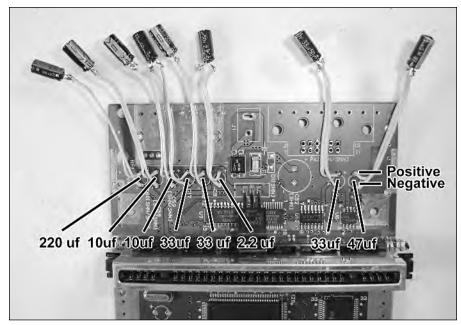
FIGURE 9-8: Reconnecting the eight capacitors.
