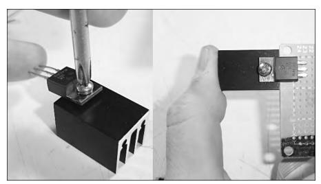
FIGURE 7-22: Attaching the heat sink and installing the regulator.
