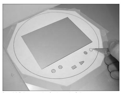
FIGURE 13-2: Taping a paper pattern down to engraving plastic.
