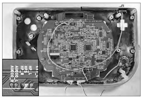
FIGURE 7-18: Attaching the screen, speaker, and power switch.
