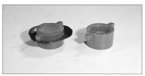
FIGURE 7-26: Modified buttons, after and before. For the ring I used the plastic from the bottom of a store-bought cake tray. (The cake was good, too.)
