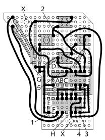
FIGURE 10-24: The connections on the back of the left PC board.
