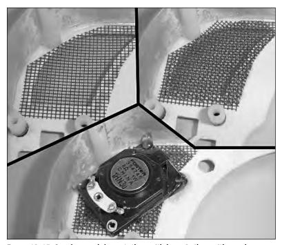
FIGURE 13-15: Speaker mesh layer 1, then with layer 2, then with speaker.
