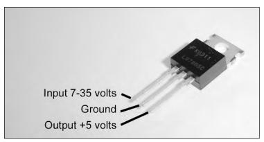
FIGURE 3-4: The 7805 linear power regulator.
