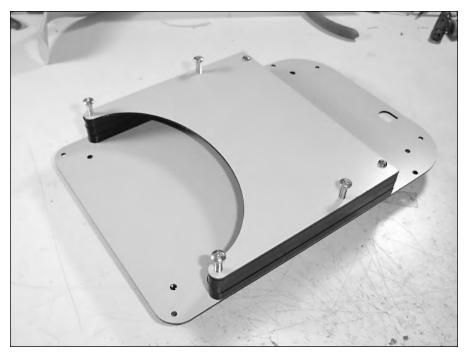
FIGURE 8-25: The cartridge holder attached to the center match plate.
