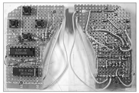
FIGURE 10-25: The front (left) and back (right) of the completed left PC board.
