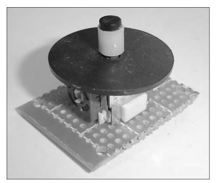
FIGURE 13-24: The right analog joystick.
