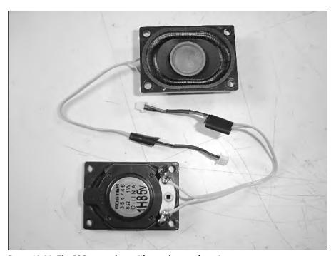
FIGURE 10-20: The PSOne speakers with new, longer plug wires.
