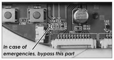
FIGURE 4-30: The fuse that you can bypass, labeled PS1 on the board.
