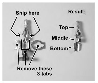
FIGURE 17-4: Where to snip the lead and what the resulting portions are called.
