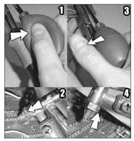
FIGURE 2-11: Desoldering something—a step-by-step pictorial guide!
