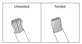
FIGURE 2-5: Stranded wire, untwisted (bad) and twisted (good).
