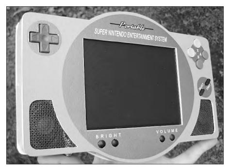
FIGURE 10-1: The hand-built SNES portable.
