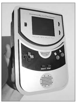
FIGURE 8-1: The completed CNC-built NES portable.
