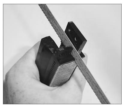
FIGURE 8-7: Where to cut the connector in half. (Don't let your old shop teacher catch you sawing like this!)
