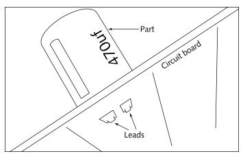
FIGURE 2-10: A part, the circuit board, and the part's leads.
