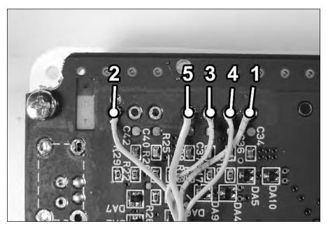
FIGURE 10-40: Connecting the built-in Player 1 controls to the SNES board.
