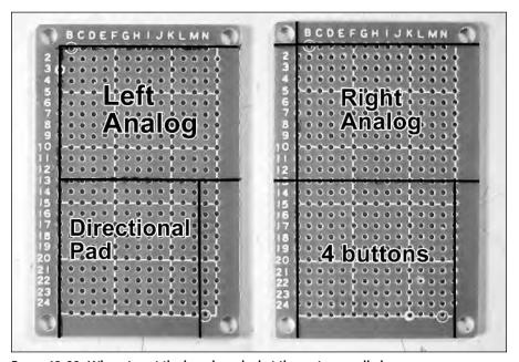
FIGURE 13-22: Where to cut the boards and what the parts are called.
