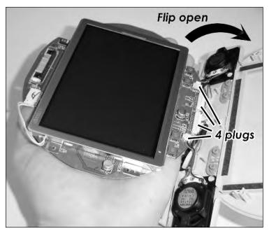
FIGURE 4-22: How to hold the unit, and which plugs to remove.
