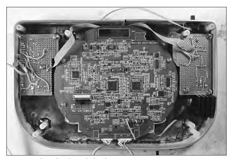
FIGURE 7-27: The PC boards attached to the case.
