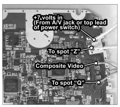
FIGURE 17-12: Audio, video, and power connections to the TV's circuit board.
