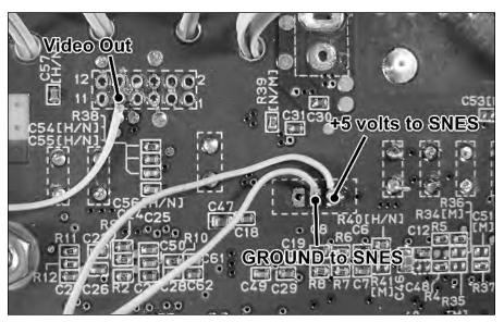
FIGURE 11-29: Connecting video, +5 volts, and GROUND to the SNES.
