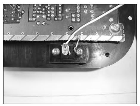
FIGURE 8-36: Where to place the battery jack riser.
