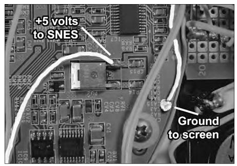
FIGURE 10-36: Connecting wires to the 7805A regulator on the PSOne screen.
