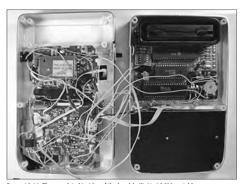
FIGURE 16-14: The completed insides of the hand-built Atari 2600 portable.
