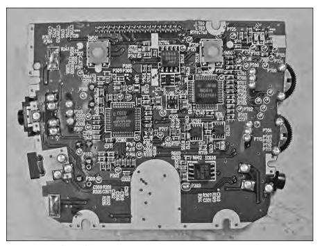
FIGURE 4-7: The front of the lower board, and what you should desolder.
