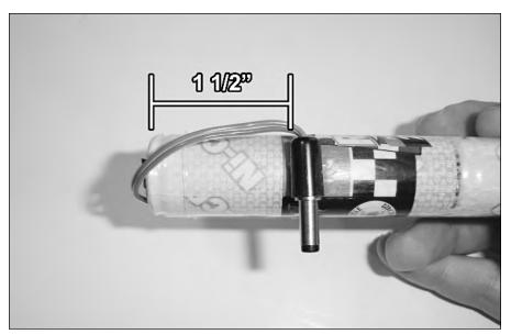
FIGURE 8-40: The power plug attached to the battery.
