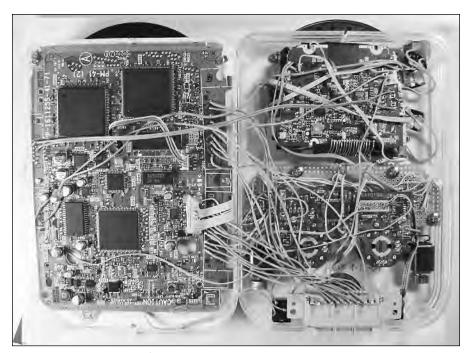
FIGURE 14-23: The insides of the PSOne portable, all wired and ready to go!
