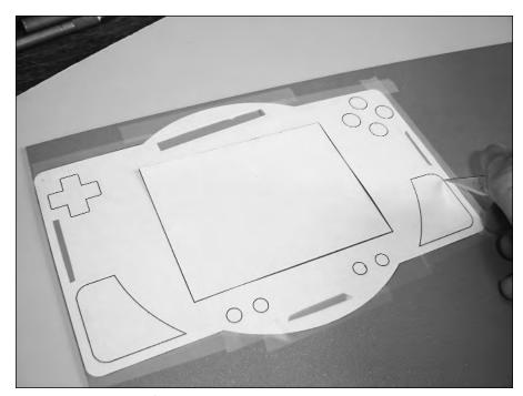
FIGURE 10-2: Cutting the first pattern.
