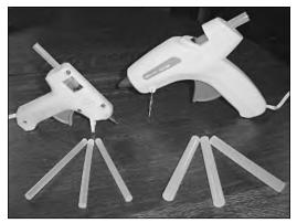
FIGURE 2-20: Mini and standard glue guns, with corresponding sticks.
