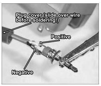
FIGURE 14-24: The wall adapter's new plug.
