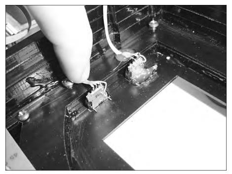
FIGURE 8-33: Inserting the volume and brightness knobs.
