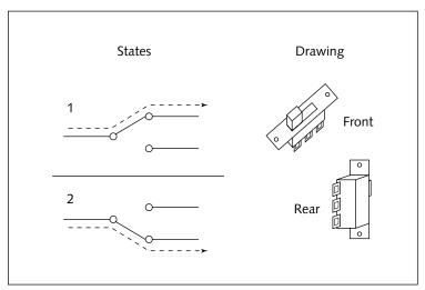
FIGURE 3-10: A SPDT switch in both states.
