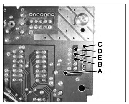
FIGURE 8-38: Attaching the control board to the NES board.
