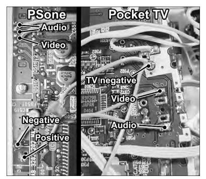
FIGURE 14-22: The audio, video, and power connections between the PSOne and pocket TV.
