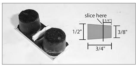
FIGURE 7-16: A rubber stopper to use for buttons.
