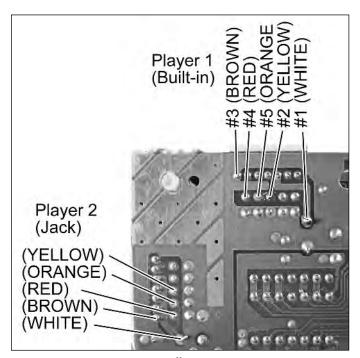
FIGURE 7-30: Reconnecting controllers.
