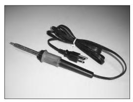
FIGURE 2-3: A lower-power "pencil" soldering iron, 15-watt range.
