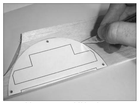
FIGURE 10-11: The battery riser pattern on 3/8" thick balsa wood.
