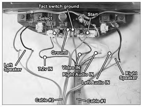
FIGURE 13-6: Both ribbon cables attached to the PSOne screen.
