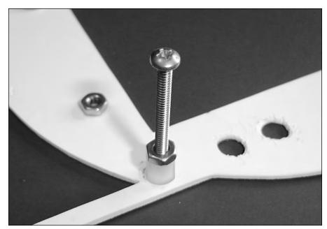
FIGURE 10-5: Attaching the size-4 nuts to nylon spacers.
