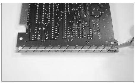
FIGURE 8-4: Where to slice off part of the NES motherboard.
