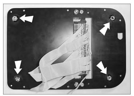
FIGURE 8-17: Where to place the NES board risers. Add a little epoxy around them for added strength.
