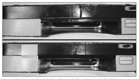
FIGURE 7-35: Using vinyl to straighten the case, before (above) and after (below).
