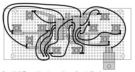
FIGURE 11-19: The remaining wire connections on the control board.
