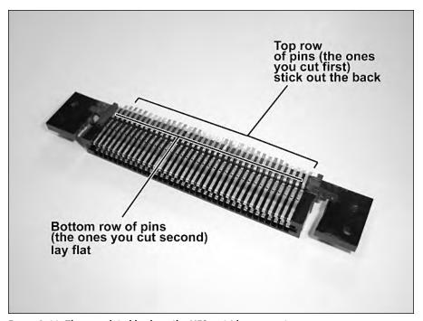
FIGURE 8-11: The completed hack on the NES cartridge connector.
