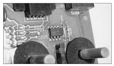
FIGURE 15-2: The small 8-pin IC chip that you may have to rewire.
