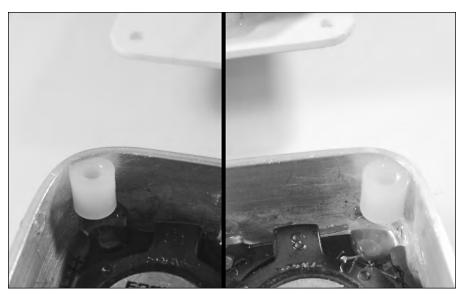
FIGURE 10-42: The final two screw posts to attach to the unit.
