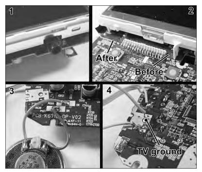
FIGURE 11-24: The four things to do before installing the pocket TV.
