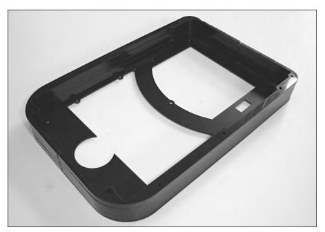
Figure 8-21. Attaching front walls to the front plate.
