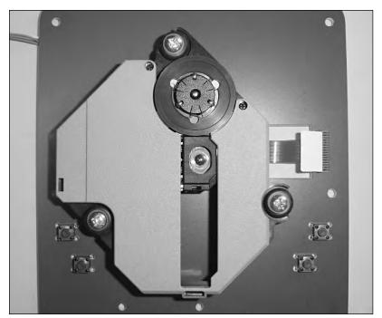
FIGURE 14-6: The CD-ROM drive installed onto the rear plate.
