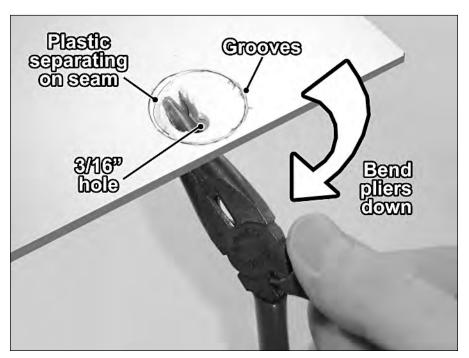
FIGURE 7-3: Bending, cracking, and separating the plastic.
