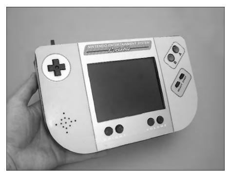
FIGURE 7-1: A hand-built NES portable.
