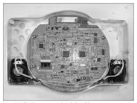
FIGURE 10-21: The PSOne screen inserted into the front of the case.
