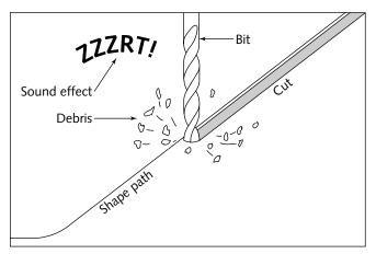
FIGURE 5-6: A bit making an engrave cut.
