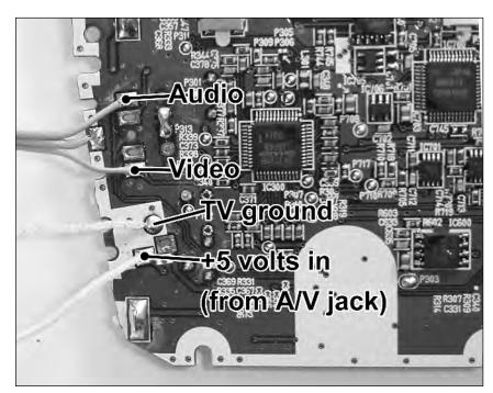
FIGURE 16-11: Audio, video, and ground connections on the EV-680.
