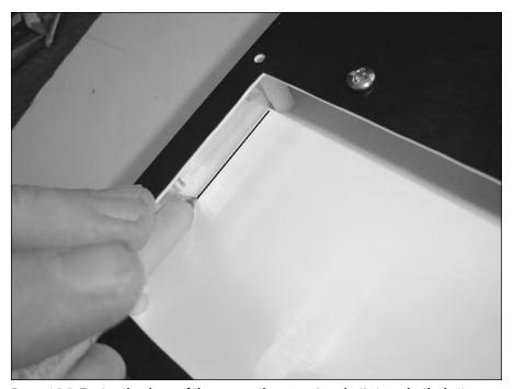
FIGURE 16-5: Tracing the shape of the case on the engraving plastic to make the battery backer.
