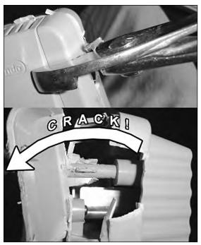
FIGURE 9-4: Prying the case open to reveal the screw posts.
