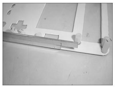
FIGURE 16-2: Where the aluminum should start and placement of the notch.
