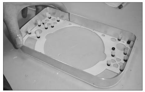
FIGURE 13-11: The aluminum bent around the front plate.
