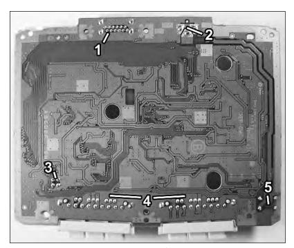
FIGURE 12-4: Desoldering spots on the back of the PSOne board.
