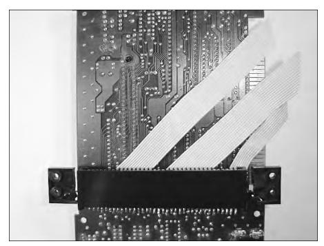
FIGURE 8-14: How the cartridge connector and wires are placed in relation to the NES board.
