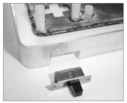
FIGURE 7-9: The power switch hole and the switch itself.
