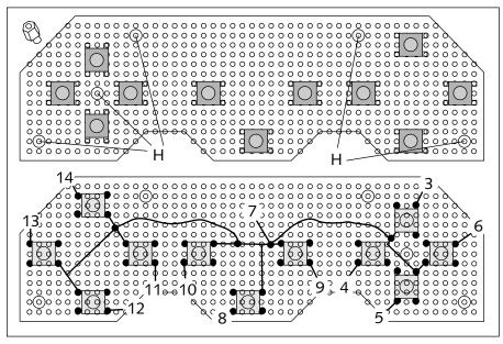
FIGURE 14-14: Placement of tact switches (top drawing) and wiring on the back (bottom drawing).
