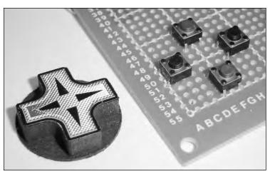
FIGURE 3-14: Tact switch pushbuttons used as an up/down/left/right gamepad.
