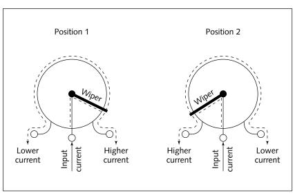
FIGURE 3-16: A potentiometer, shown at two different positions.
