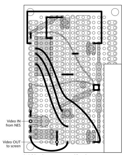
FIGURE 7-20: The left board connections, viewed from the rear.
