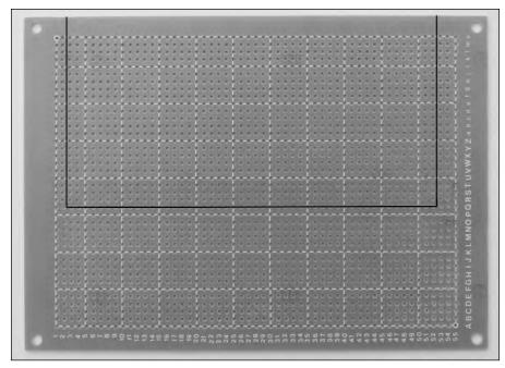
FIGURE 8-26: Where to slice down the raw PC board.
