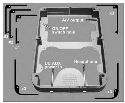
FIGURE 11-4: Which front side walls to stack and glue to the back of the front plate, and where to drill the holes.
