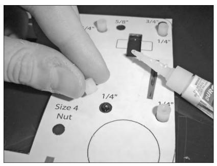
FIGURE 7-7: Placing spacers with superglue on the pattern.
