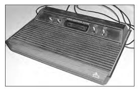
FIGURE 1-7: The four-switch Atari 2600 Video Computer System.
