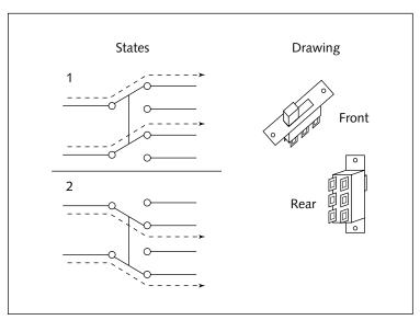
FIGURE 3-11: A DPDT switch in both states.
