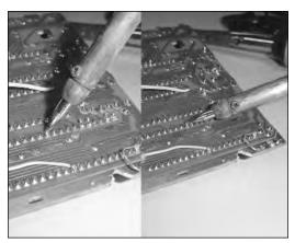
FIGURE 2-8: Tip held straight (correct), and tip tilted too far sideways (incorrect).
