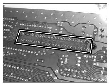
FIGURE 6-3: The leads holding the useless expansion port in place.
