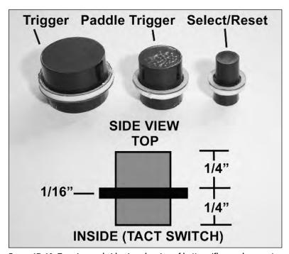
FIGURE 17-10: Top view and side view drawing of buttons/flange placement.
