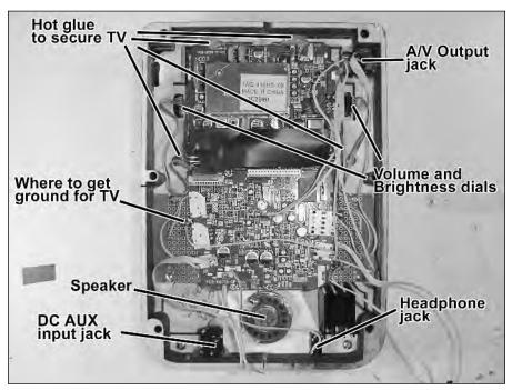
FIGURE 11-25: How the inside of the front of the case should look at this point.
