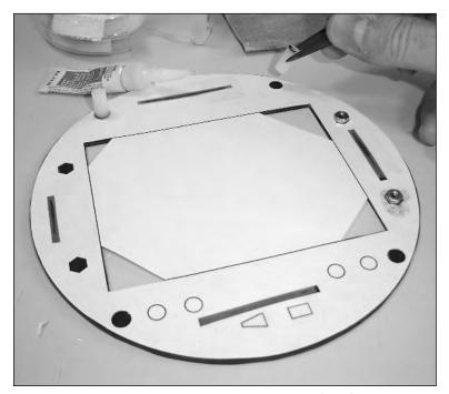
FIGURE 13-4: The screw post pattern taped to the back of the front screen plate.
