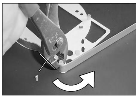
FIGURE 10-8: How to make bend #3 in the aluminum.
