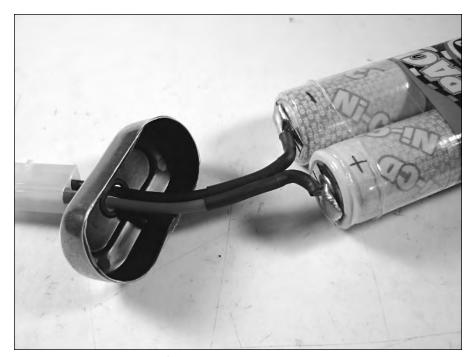
FIGURE 8-39: The cap removed from the 7.2-volt battery pack.
