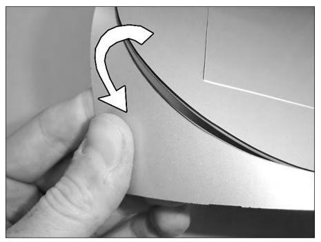
FIGURE 13-3: Bending the plastic around the edges of the front screen plate circle.
