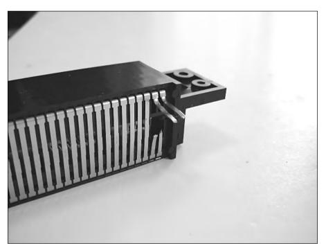
FIGURE 8-8: Snipping and bending the first set of pins.
