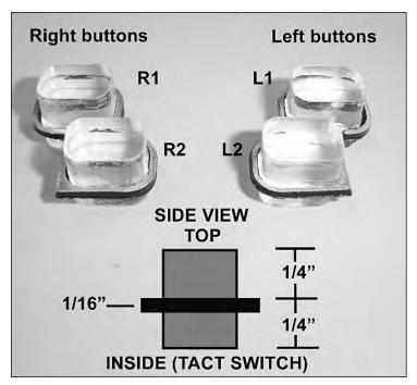
FIGURE 14-7: The shoulder buttons, with handy cross-section drawing.
