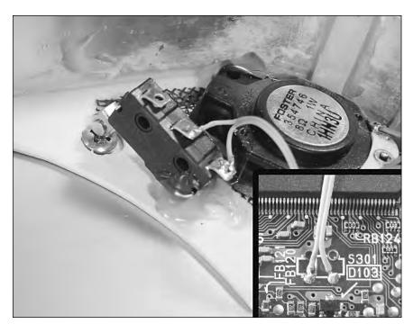
FIGURE 13-29: The lid sensor switch hot-glued in place.
