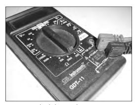
FIGURE 2-17: The dial set to ohms.
