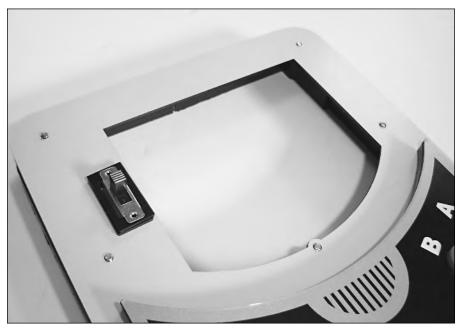
FIGURE 8-31: The five screws, two power switch risers, and the power switch itself, all in place.
