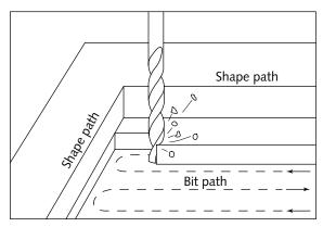
FIGURE 5-10: A bit doing a cleanout.
