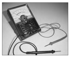
FIGURE 2-14: An analog multimeter.
