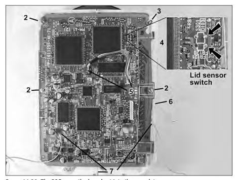
FIGURE 14-20: The PSOne motherboard set into the rear plate.
