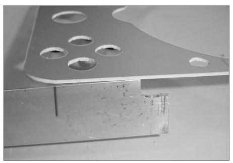
FIGURE 13-10: Where the notched end of the aluminum should start.
