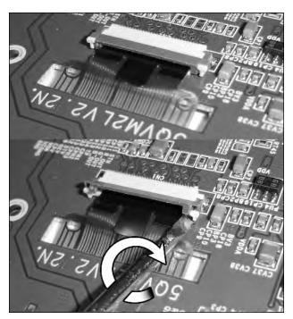
FIGURE 4-23: Unclamping the ribbon cable.
