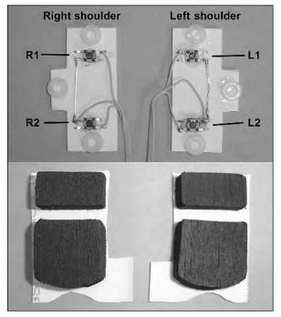
FIGURE 13-18: The tact switches on the shoulder button plates and the shoulder buttons themselves.
