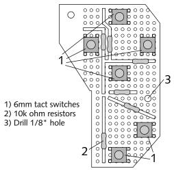
FIGURE 10-26: Placing components on the front of the right PC board.
