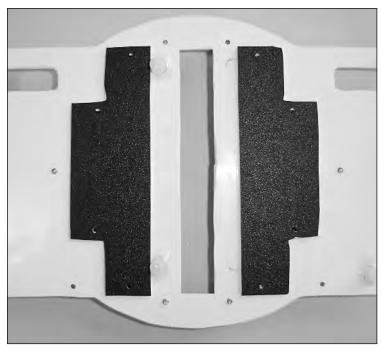
FIGURE 10-14: Gluing down the battery backers.
