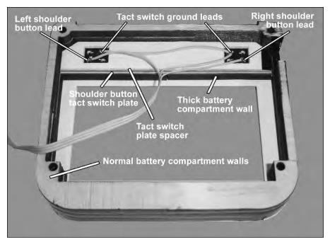
FIGURE 11-5: The battery compartment thus far, with items identified.
