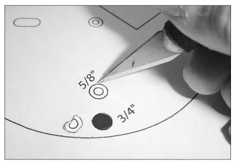
FIGURE 7-6: Cutting out the screw posts on the second pattern.
