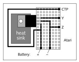
FIGURE 15-7: Sample power supply for Atari 2600.
