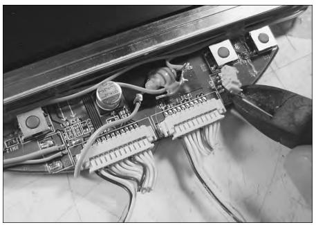
FIGURE 7-17: The cables cut, the speaker wire attached, and the old speaker plugs being removed.
