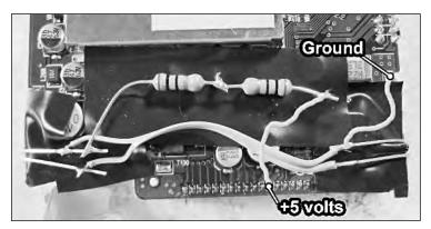
FIGURE 4-11: The LEDs connected in parallel, the resistors connected in series, and the power/ground spots.
