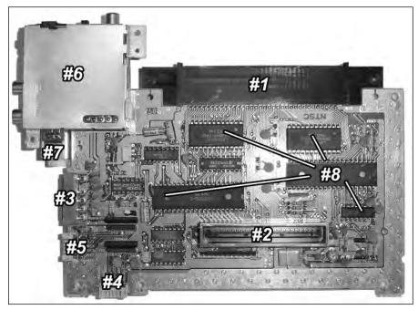
FIGURE 6-2: The NES, with parts labeled.
