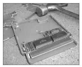
FIGURE 1-2: The guts of a NES cartridge.
