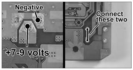
FIGURE 12-7: Where to attach power and how to jump the power switch.
