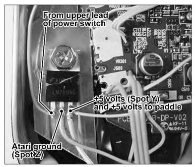
FIGURE 16-13: The installed 7805 regulator and heat sink.
