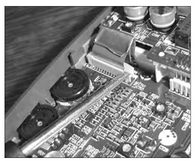
FIGURE 4-6: Releasing the ribbon cable.
