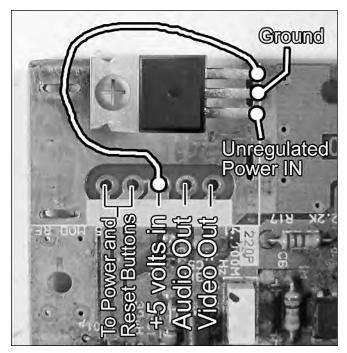
FIGURE 6-6: The audio/video power connection spot on the NES.
