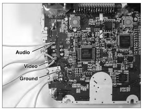
FIGURE 8-32: Attach wires to these three spots before installing the TV screen.
