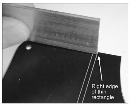
FIGURE 7-12: Initial place to line up the 1"-thick aluminum wall.
