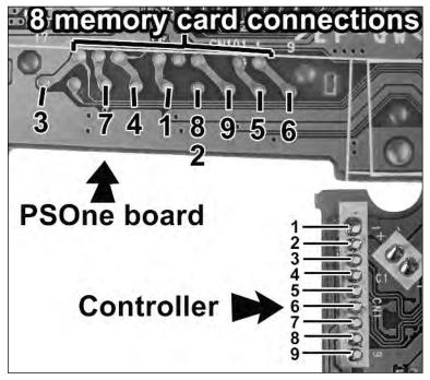
FIGURE 12-11: Controller connector pinout (lower right) and corresponding spots on PSOne board (top).
