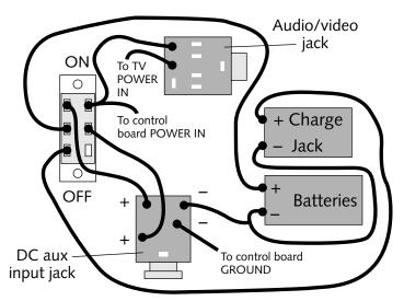
FIGURE 11-26: Power switch and battery connections.
