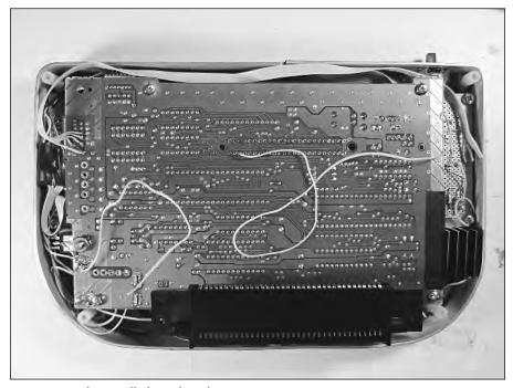
FIGURE 7-31: The installed NES board.
