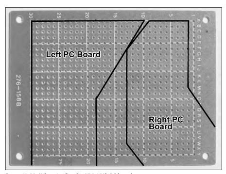
FIGURE 10-22: Where to slice the 276-158b PC board.
