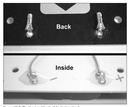
FIGURE 17-5: The front and back of the battery leads.
