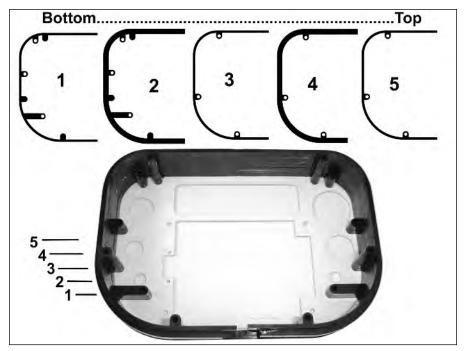
FIGURE 17-3: The front of the case and the order in which to apply wall layers.
