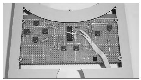
FIGURE 8-30: The control board attached to the front plate.
