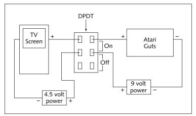
FIGURE 3-12: A DPDT switch used for a dual power supply. (Confession: I did this with the very first portable Atari that I built.)
