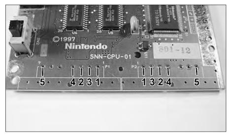
FIGURE 9-12: How the custom-made controllers hook up to the SNES board.
