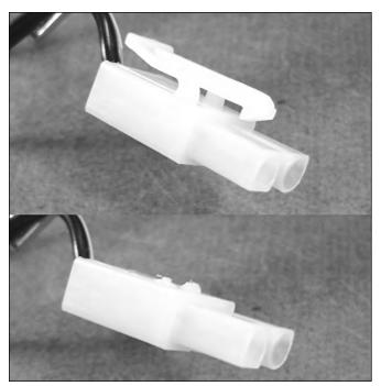
FIGURE 11-27: The charger plug, before and after snipping the tab off.
