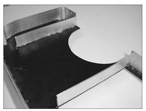
FIGURE 7-14: Inside walls attached to rear plate.
