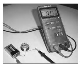
FIGURE 2-18: The current goes from the battery through the multimeter, then through the motor, and back to the battery.
