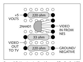
FIGURE 6-7: How to wire the video amplifier for the NES.
