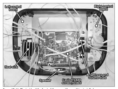
FIGURE 17-11: The inside of the front of the case with everything installed.
