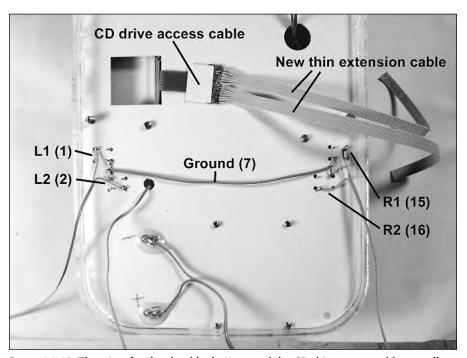
FIGURE 14-18: The wires for the shoulder buttons and the CD drive access cable as well.
