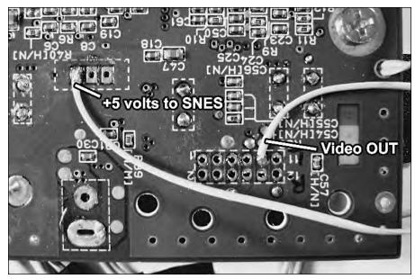
FIGURE 10-38: Connecting the power and the video wire to the SNES board.
