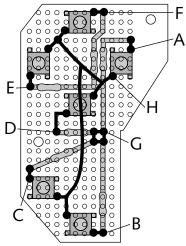
FIGURE 10-27: Connections to make on the back of the right board.
