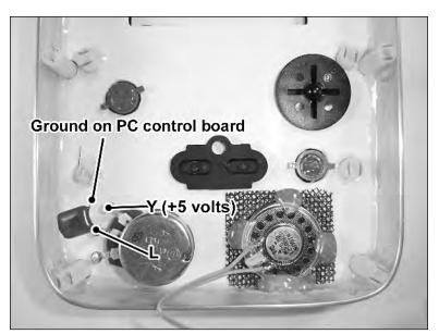
FIGURE 16-10: The case with the paddle, green capacitor, buttons, and speaker installed.
