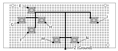
FIGURE 15-8: Sample controller for hacked-up Atari 2600.
