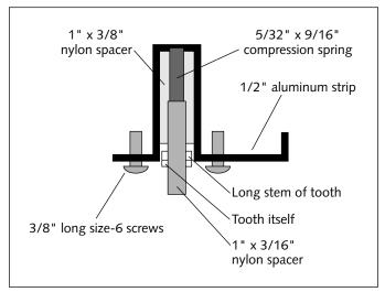
FIGURE 13-12: The latch assembly with parts labeled.
