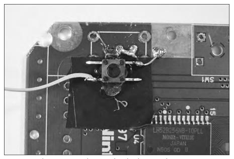
FIGURE 10-31: Placing a tact switch on SNES board and snipping the corner.
