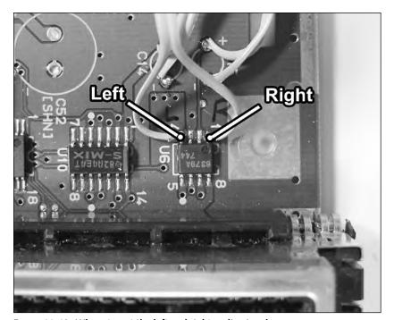
FIGURE 11-12: Where to get the left and right audio signals.
