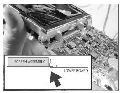
FIGURE 4-16: Placing the lower board against the screen assembly.
