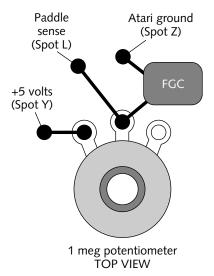
FIGURE 15-9: How to hook a paddle controller to the Atari.
