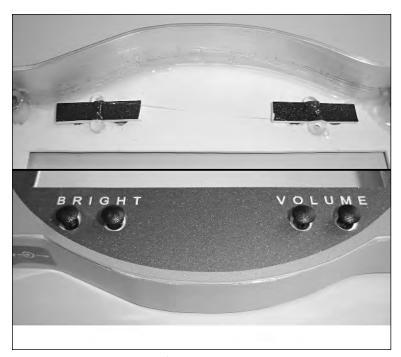
FIGURE 10-19: Front and back of the new brightness and volume buttons, glued in place.
