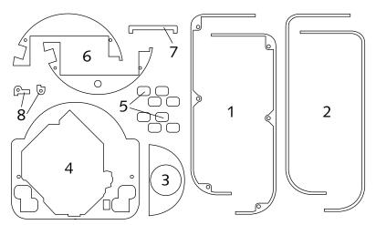
FIGURE 14-3: The 1/4"-thick side wall parts.
