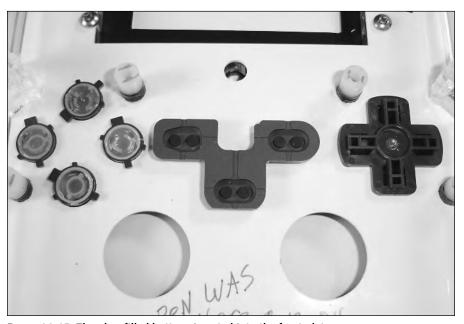
FIGURE 14-15: The glue-filled buttons inserted into the front plate.
