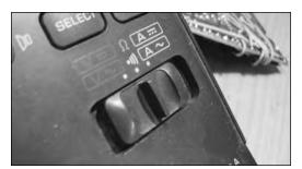
FIGURE 2-16: The selector switch on an autoranging multimeter. From left to right: voltage, resistance, and amperage.
