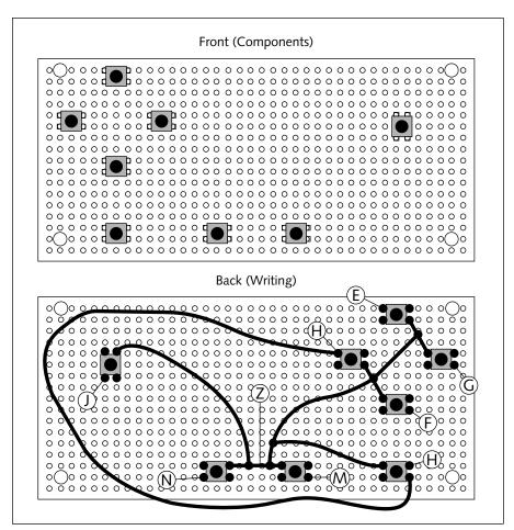
FIGURE 16-9: Placement of components (front) and wiring (back) on the PC control board.
