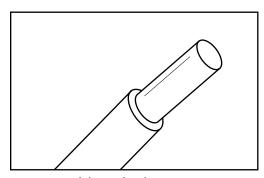
FIGURE 3-7: Solid wire detail.
