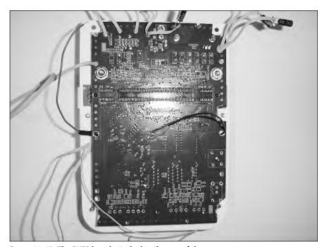
FIGURE 11-15: The SNES board attached to the rear of the case.
