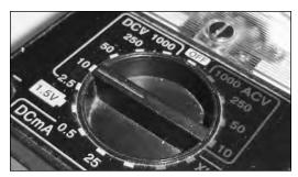
FIGURE 2-15: Multimeter set to test DC voltage.
