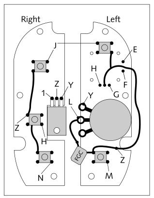
FIGURE 17-8: Wiring on the backs of the left and right control boards.
