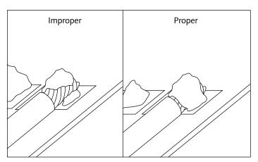
FIGURE 2-6: Improperly covered wire and properly covered wire.
