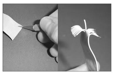
FIGURE 3-8: Slicing and stripping ribbon cable.
