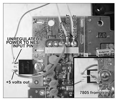
FIGURE 7-29: The 7805 regulator attached to the NES, with connections made.
