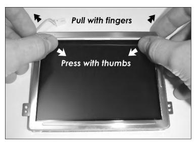
FIGURE 4-24: Removing the shield. (Don't eat potato chips just before doing this.)
