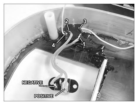
$\begin{tabular}{ll} Figure 7-32: The auxiliary DC input jack installed in the rear of the case, along with the battery connector. \end{tabular}$
