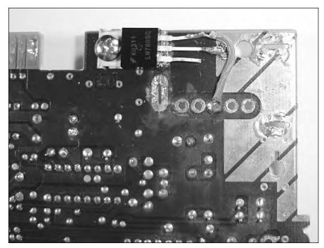
FIGURE 8-18: How to attach the 7805 regulator to the NES board.
