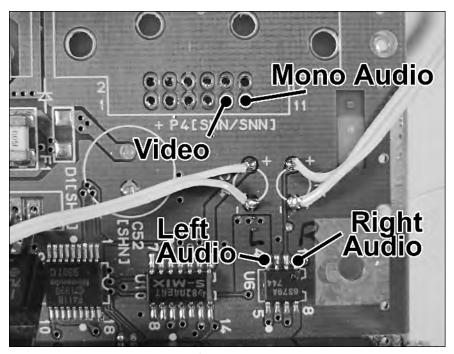
FIGURE 9-9: Video, mono audio, and left and right audio sources.
