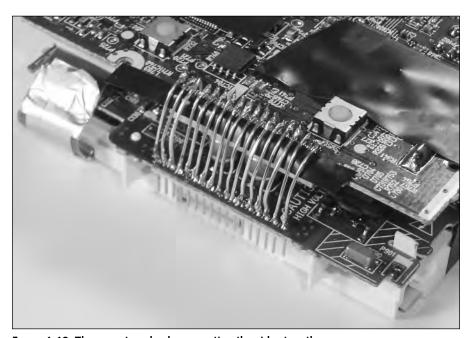
FIGURE 4-18: The seventeen leads connecting the sides together.
