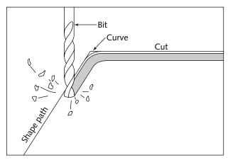
FIGURE 5-8: A bit making a female cut.
