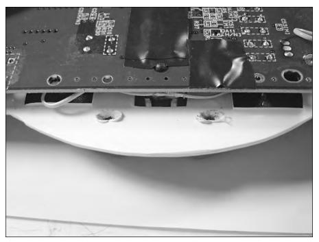
FIGURE 10-44: Making "targeting slits" in the plastic.
