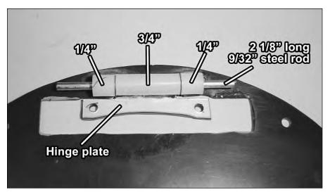
FIGURE 13-9: The nylon spacers, steel rod, hinge plate, and rear screen plate.
