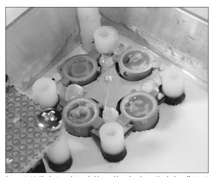
FIGURE 13-25: The buttons, button holder, and hot glue drops. (Crude, but effective.)
