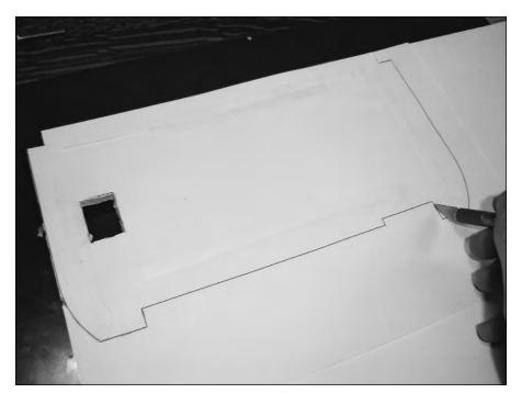
FIGURE 7-15: Cutting the 1/4" spacer. An X-Acto foam board is shown here.
