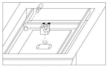
FIGURE 5-3: A laser engraver and the cutting beam.
