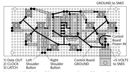
FIGURE 11-18: The first layer of things to connect on the rear of the control board.
