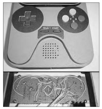
FIGURE 11-23: The installed control riser and board, front and inside.
