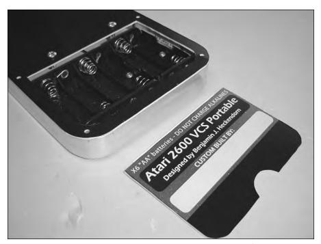
FIGURE 16-7: The battery holder in the rear case and the door to protect it from the elements.
