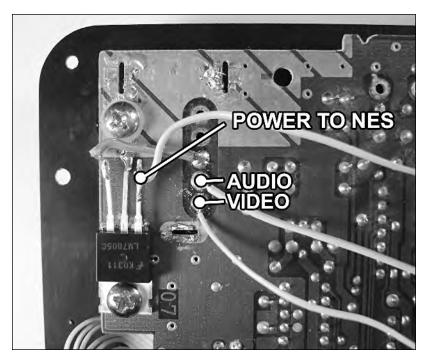
FIGURE 8-37: Attaching audio, video, and power to the NES board.
