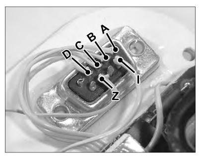
FIGURE 17-14: Connecting the Player 2 joystick port to the Atari.
