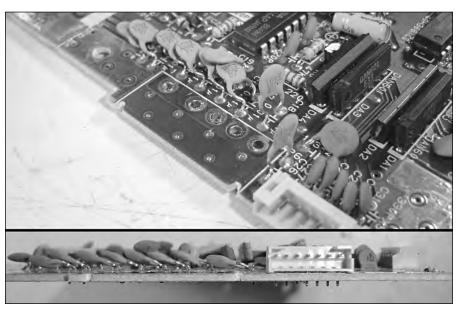
FIGURE 6-4: Bent and unbent capacitors. Also a view from the side!
