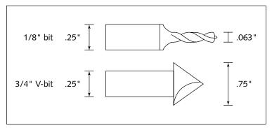
FIGURE 5-2: Examples of different router bit sizes.
