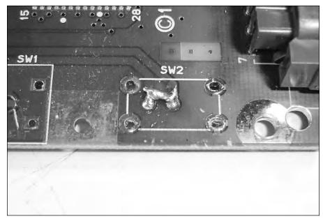
FIGURE 9-7: Jumping the power switch to be always "on."
