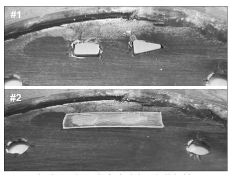
FIGURE 13-7: The select/start buttons sliced and with plastic glued behind them.
