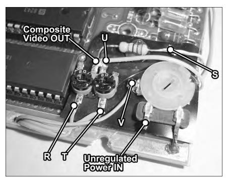
FIGURE 15-6: Atari 2600 composite video circuit.
