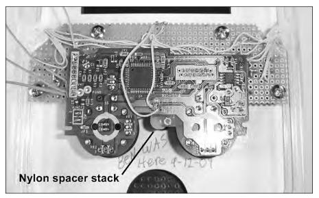
FIGURE 14-16: The controller board and nylon spacer all securely hot-glued in place!
