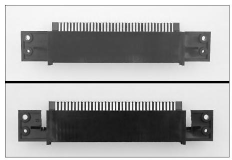
FIGURE 8-5: A NES cartridge connector, before and after hacking.
