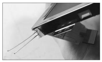
FIGURE 4-26: Where the metal frame may need cutting.
