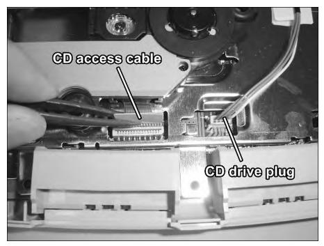
FIGURE 12-2: Removing the plugs and cables.
