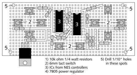
FIGURE 11-17: Where to place components on the front of the control board.
