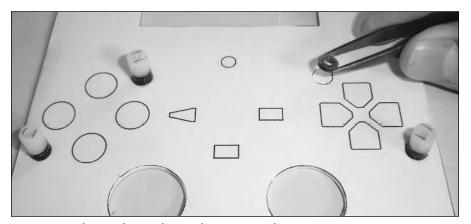
FIGURE 14-4: Gluing nylon washers and spacers into the screw post spots.
