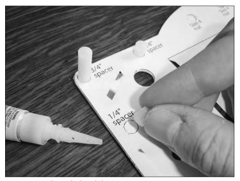
FIGURE 10-4: Parts being glued into holes.
