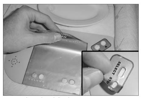
FIGURE 7-5: Applying graphics to the front plate.
