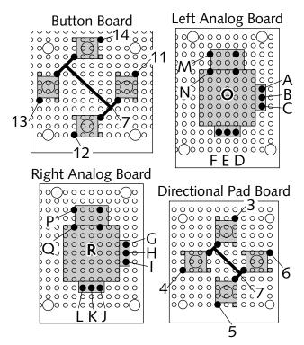
FIGURE 13-31: Wiring connections on the backs of the four PC boards.
