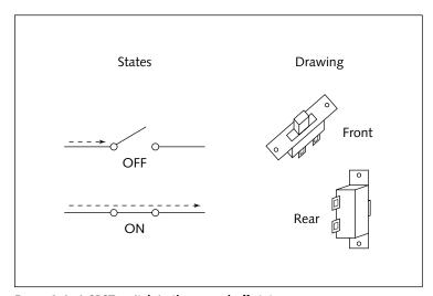
FIGURE 3-9: A SPST switch in the on and off states.
