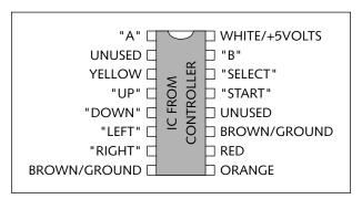
FIGURE 6-9: The pinouts of the IC inside the NES controller. Notice the groove on one end of the IC—this tells you which way to install it.
