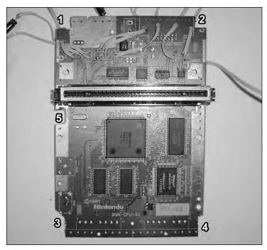
FIGURE 11-13: The SNES with portions cut off the motherboard.
