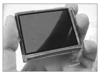
FIGURE 4-1: The LCD glass, properly held.
