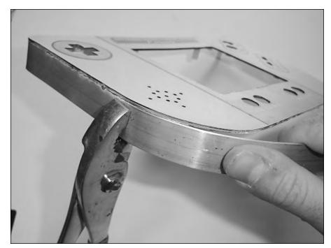
FIGURE 7-10: Bending the second curve. The pliers keep the already-glued portions from bending.
