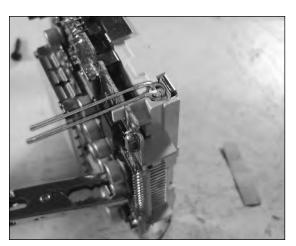
FIGURE 4-9: Placement of left LED, with bent wires.
