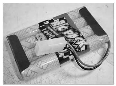
FIGURE 3-1: A remote-control car's Ni-MH battery pack, rated for 9.6 volts at 1600 mA.
