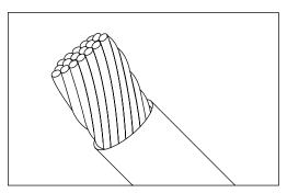
FIGURE 3-6: Stranded wire detail.
