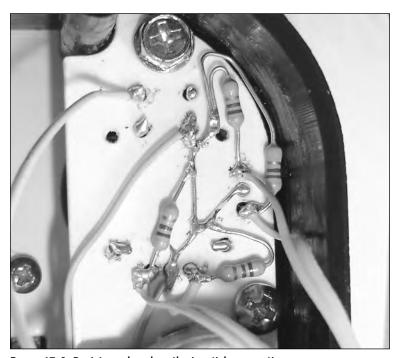
FIGURE 17-9: Resistors placed on the joystick connections.
