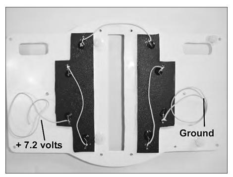
FIGURE 10-17: Attaching power wires to the battery terminals.
