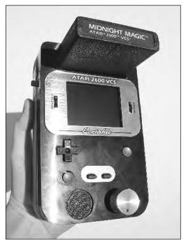
FIGURE 16-1: A simple, compact Atari 2600 portable.
