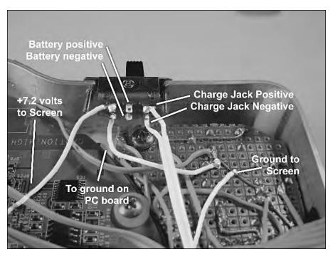
FIGURE 10-35: The ON/OFF switch installed, with wiring.
