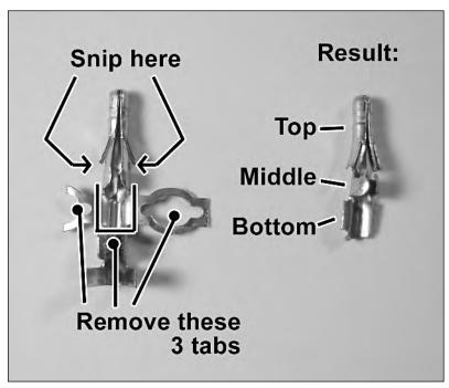
FIGURE 13-17: Where to snip the lead and what the resulting portions are called.
