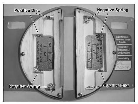
FIGURE 10-16: The placement of the battery terminals and decals.
