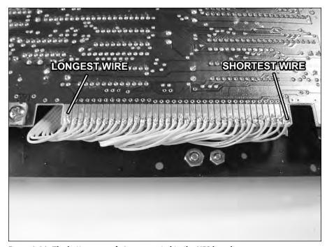
FIGURE 8-20: The bottom row of pins connected to the NES board.
