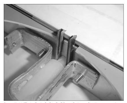
FIGURE 13-14: The teeth attached to the lid open button and resting on engraving plastic and folded paper.
