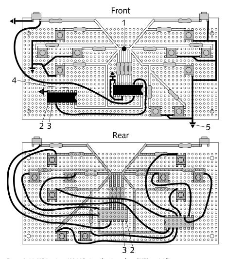
FIGURE 9-11: Wiring two 4021 ICs together to make a SNES controller.
