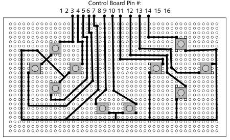
FIGURE 12-10: Sample PSOne controller on a piece of PC board.
