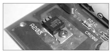
FIGURE 3-3: The power regulator in the Atari 2600.
