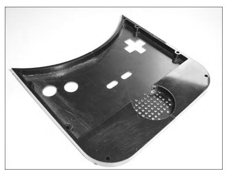
FIGURE 8-23: The control riser walls glued to the control plate.
