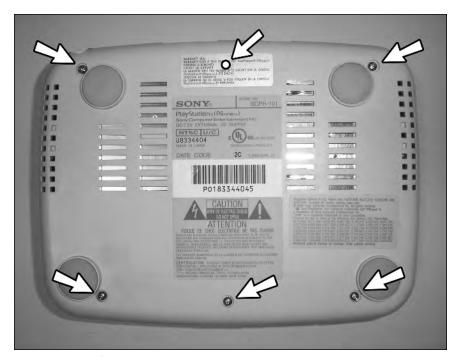
FIGURE 12-1: The first six screws to remove, including the warranty-voiding one!
