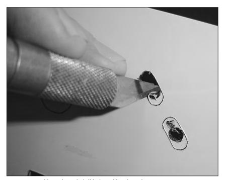
FIGURE 7-4: Grabbing through drill hole and bending plastic apart.
