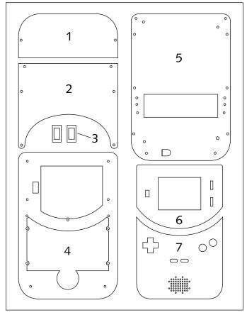
FIGURE 8-2: The plates for the CNC-built NES (made of 1/16"-thick engraving plastic).
