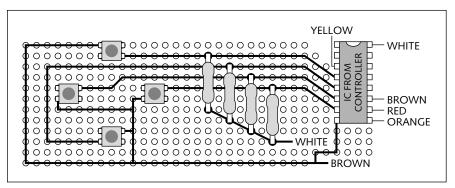
FIGURE 6-10: A rebuilt NES controller circuit. The gray things are all 47K ohm resistors. White is +5 volts, and brown is ground/negative.
