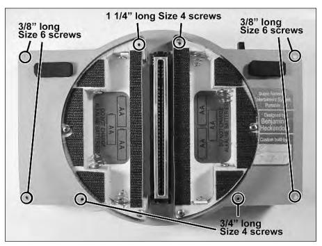
FIGURE 10-43: Which screws to use for the final assembly.
