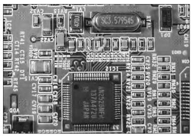
FIGURE 4-31: Bypass CV23 to make the screen brighter.
