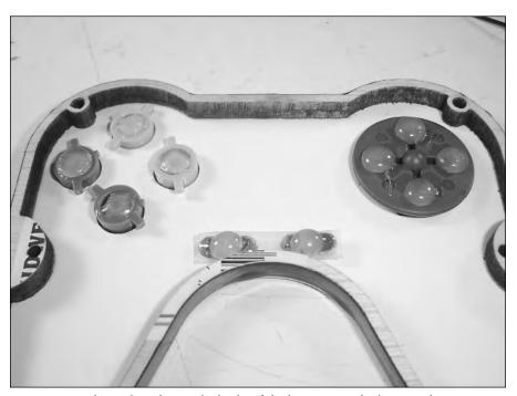
FIGURE 11-22: Placing hot glue on the backs of the buttons, inside the control riser.
