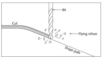
FIGURE 5-7: A bit making a male cut.
