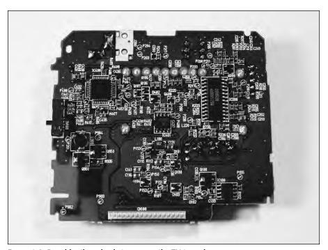
FIGURE 4-8: Desolder these leads to remove the TV tuner box.
