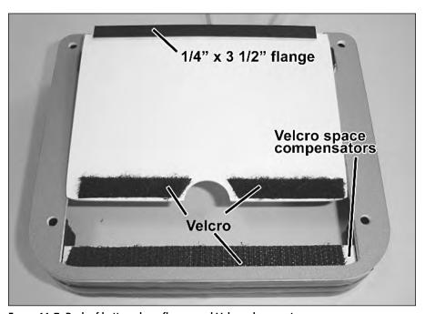
FIGURE 11-7: Back of battery door, flange, and Velcro placement.
