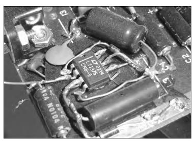
FIGURE 3-5: The eight-pin chip in the center is a switching regulator wired to provide 5 volts.
