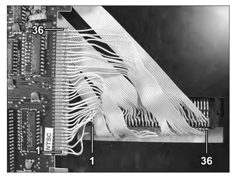
FIGURE 8-19: The top row of pins connected to the NES board.
