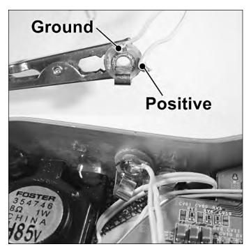
FIGURE 10-34: Wiring the charging jack and installing it in the unit.
