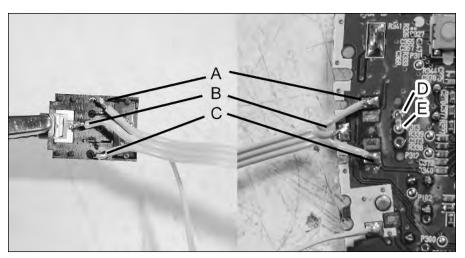
FIGURE 4-13: Connect to the plug and board as shown. (Note how wire B is longer on the plug side.)
