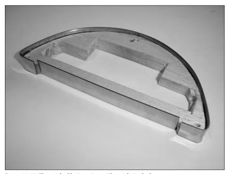
FIGURE 10-13: The notched battery riser, with metal attached.
