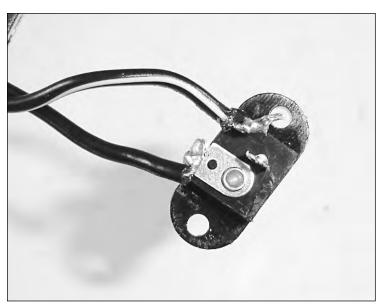
FIGURE 8-42: The new size K plug attached to the charging unit.
