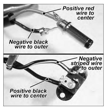
FIGURE 7-33: TOP: The plug replaced on the battery pack. BOTTOM: The jack connected to the battery charger.
