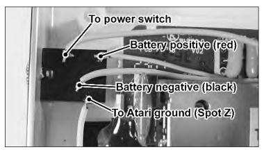
FIGURE 16-12: Connections to the DC AUX input jack.
