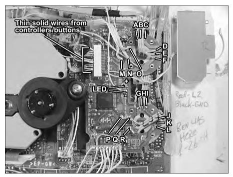
FIGURE 13-30: Placement of the controller board and pinouts.
