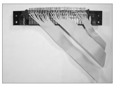
FIGURE 8-13: Attaching ribbon cable to the cartridge connector.
