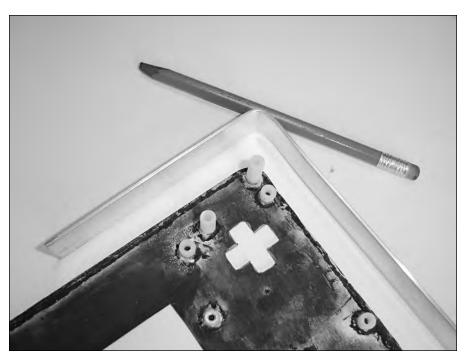
FIGURE 7-8: The first bend in the aluminum.
