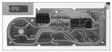
FIGURE 6-8: The inside of a standard NES controller.
