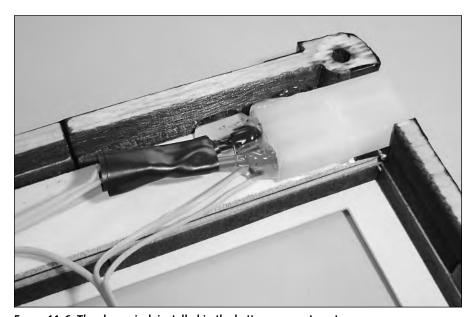
FIGURE 11-6: The charge jack installed in the battery compartment.
