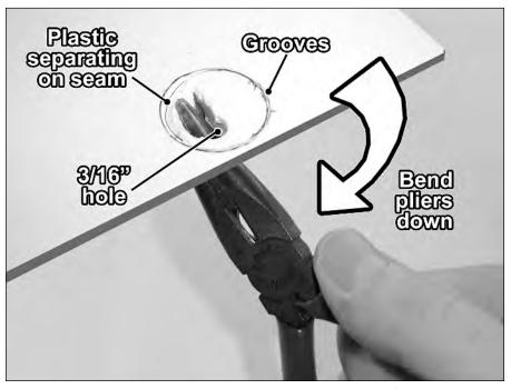
FIGURE 10-3: Bending the shapes out using the pilot holes and a pair of needle-nose pliers.
