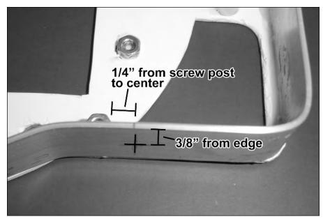
FIGURE 10-9: Target for drill hole for power jack.
