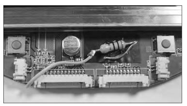
FIGURE 4-28: Placement of the 10-ohm resistor.
