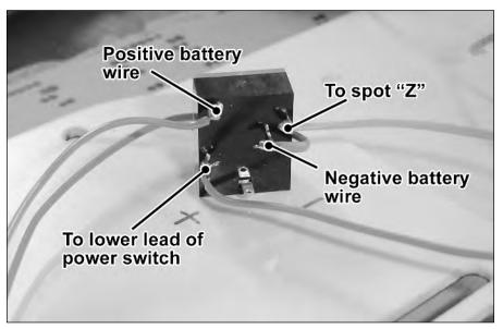
FIGURE 17-13: Wiring the DC AUX input jack.
