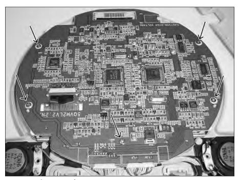
FIGURE 4-21: The next set of screws to remove.
