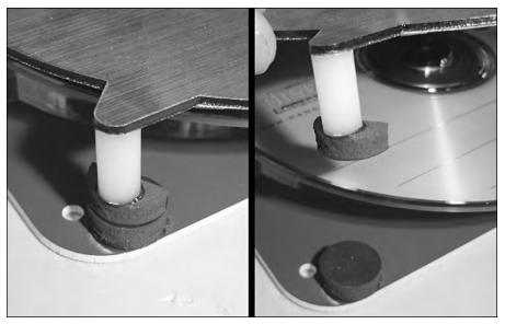
FIGURE 14-12: Magnets: An "attractive" way to make a CD lid latch.
