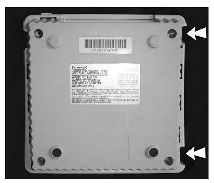
FIGURE 9-1: The correct approach angles for grinding into a mini-SNES.
