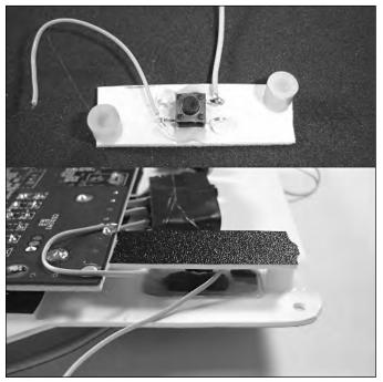
FIGURE 10-33: The tact switch and spacers attached to the engraving plastic.
