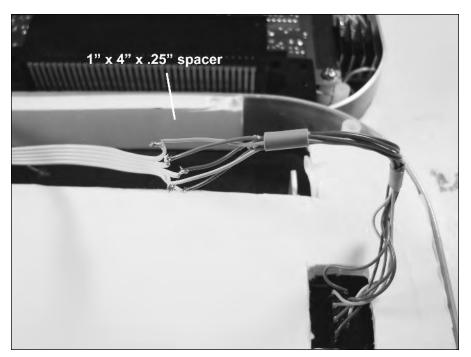
FIGURE 7-34: Attaching the Player 2 cable to the jack and the  $1" \times 4"$  spacer.
