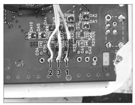
FIGURE 11-30: Attaching the controller to the SNES board.
