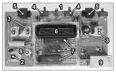
FIGURE 15-3: The Atari 2600 board with labeled parts.
