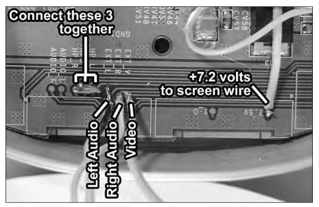
FIGURE 10-39: Connections to be made at the base of the PSOne screen.
