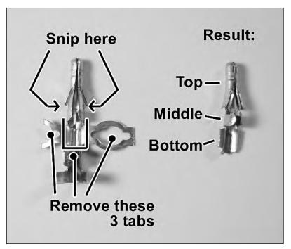
FIGURE 14-9: Where to snip the lead and what the resulting portions are called.
