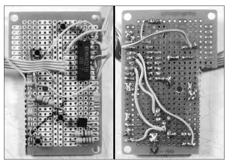
FIGURE 7-21: The completed left board, front and back.
