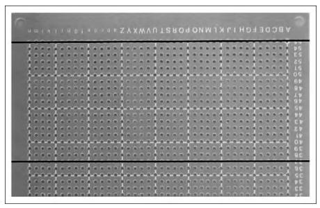
FIGURE 11-16: Where to cut apart the PC board.
