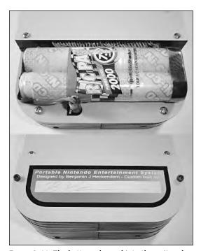
FIGURE 8-41: The battery plugged into the unit and with the holder over it.
