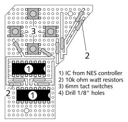
FIGURE 10-23: Placement of components on the front of the left PC board.
