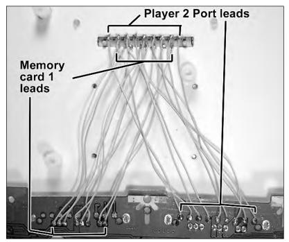
FIGURE 13-20: The memory card and Player 2 port connected to the PSOne motherboard.
