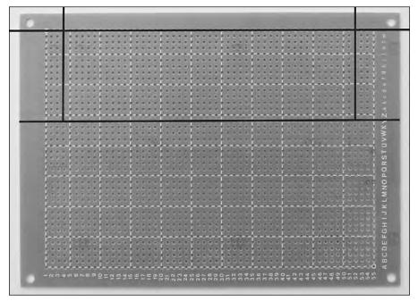
FIGURE 14-13: Where to cut the PC board.
