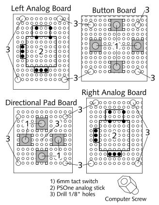
FIGURE 13-23: The placement of components on the four PC boards.
