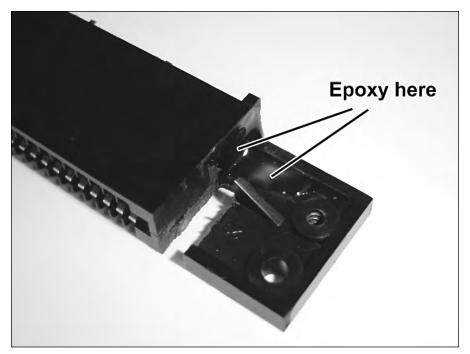
FIGURE 8-12: The sides of the connector with epoxy glopped on for added support.
