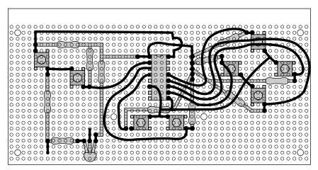
FIGURE 8-28: Connections to make on the back of the control board.
