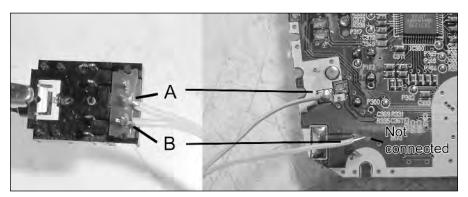
FIGURE 4-12: Connect to the plug and board as shown ("B" is not yet connected on the board side).
