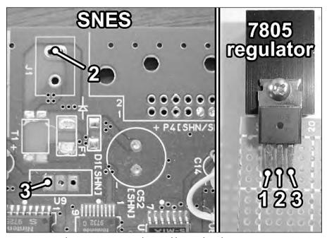
FIGURE 9-10: Hooking a new 7805 regulator and heat sink to the SNES.
