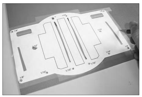
FIGURE 10-10: The rear plate being cut. Note the extra slits in the paper that allow it to be taped down in more places.
