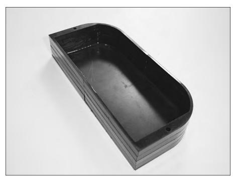
FIGURE 8-24: The battery holder walls glued to the battery holder plate.
