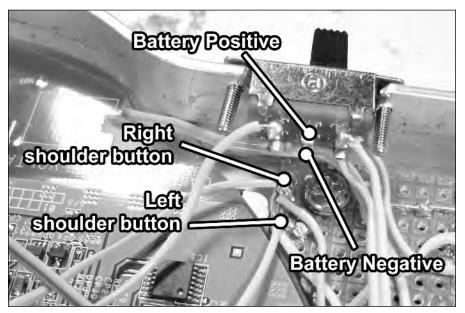
FIGURE 10-37: Connecting the right and left shoulder buttons to the PC board.
