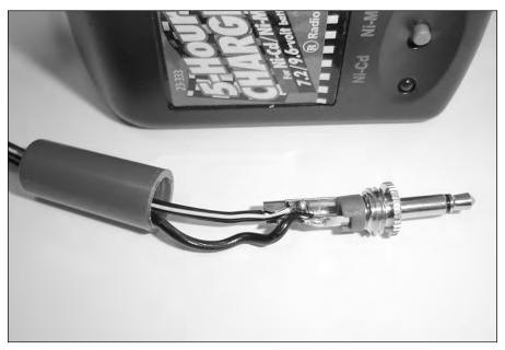
FIGURE 10-41: Attaching a new plug on the end of the battery charger.
