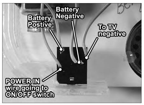
FIGURE 14-21: The DC AUX INPUT jack, with wires attached.
