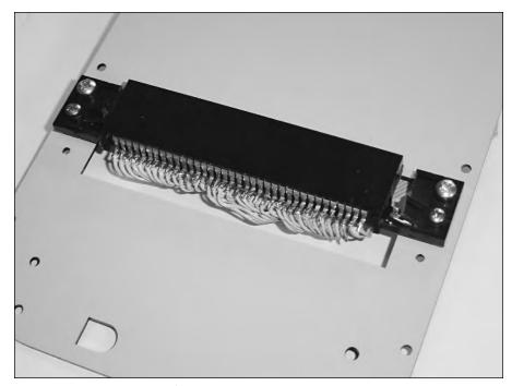
FIGURE 8-16: The placement of the cartridge connector on the center match plate.
