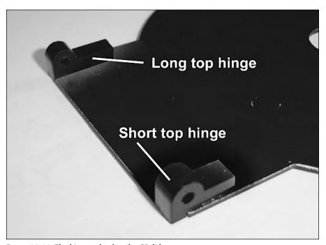
FIGURE 14-11: The hinges glued to the CD lid.
