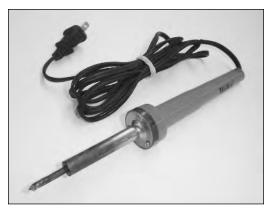
FIGURE 2-2: A medium-power soldering iron, 40-watt range.
