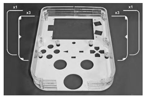
FIGURE 14-5: The side walls attached to the front plate.
