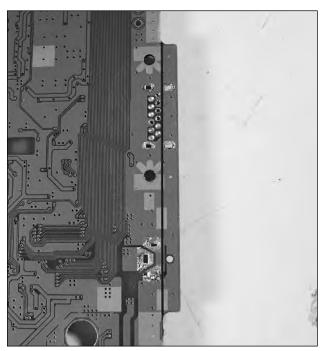
FIGURE 14-19: Where to slice off the top portion of the PSOne board.
