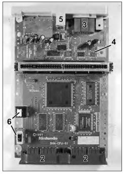
FIGURE 9-6: The SNES board with important parts labeled.
