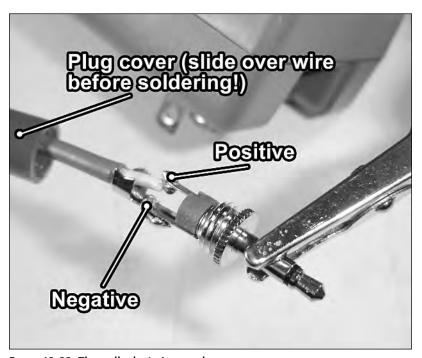
FIGURE 13-33: The wall adapter's new plug.
