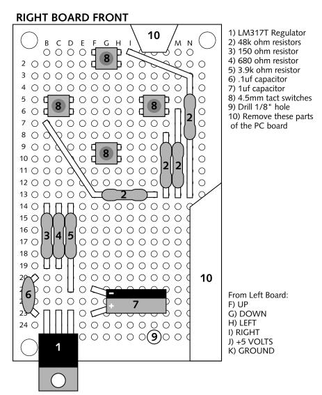
FIGURE 7-23: Installing parts on the right board.
