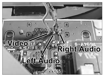
FIGURE 13-28: The video and audio connections from the PSOne board to the screen.
