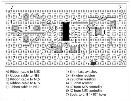
FIGURE 8-27: Where to place components on the front of the control board.
