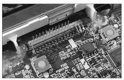
FIGURE 4-17: Bending pins and soldering them in place.
