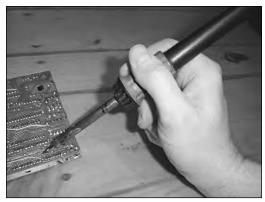
FIGURE 2-7: The proper way to hold a soldering iron. (If you're left-handed, hold this page up to a mirror.)
