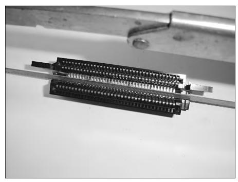
FIGURE 8-10: Saw through the pins like this.
