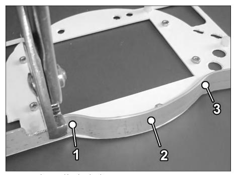
FIGURE 10-7: The second bend in the aluminum.
