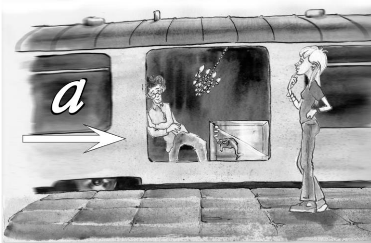
Fig. 1.3 The water in an accelerated fish tank. The rear wall of the tank rushes upon the water, raising its adjacent surface, while the front wall accelerates away from the water, giving it extra
