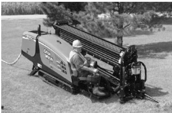
FIGURE 4.6 Directional drilling machine [DitchWitch].
