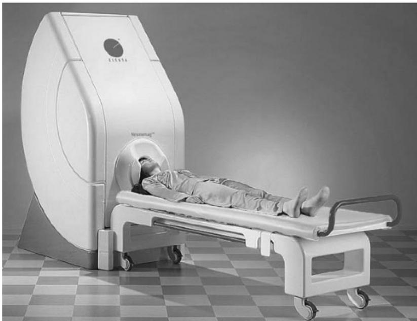
**Figure 11.11** Multichannel SQUID system for neuromagnetic studies of the brain. With permission from Neuromag.
