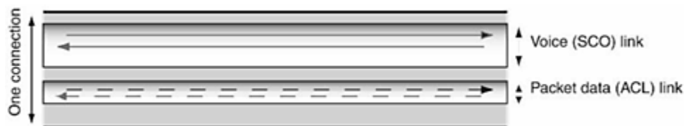
Figure 5.4 ACL and SCO links sharing one connection.
