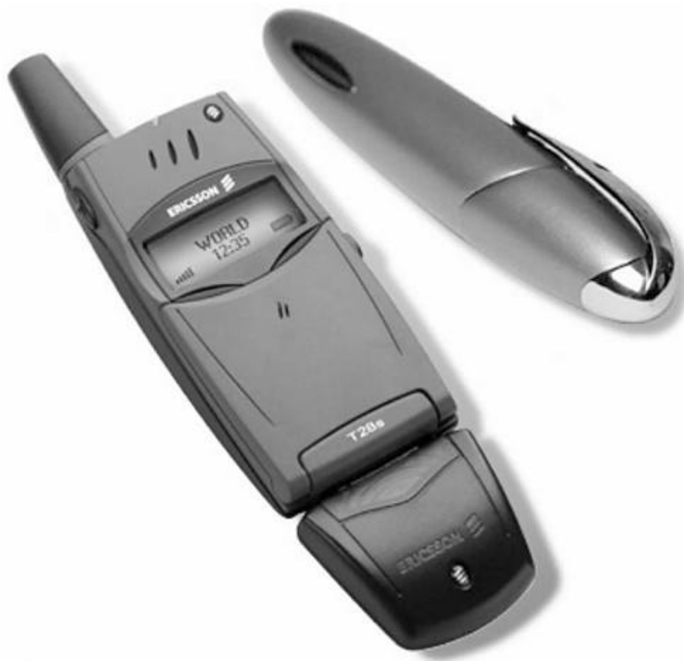
Figure 10.4 Anoto technology with a Bluetooth-enabled pen.
