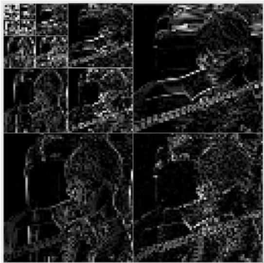
Figure 3.35 Five-stage wavelet decomposition of image
