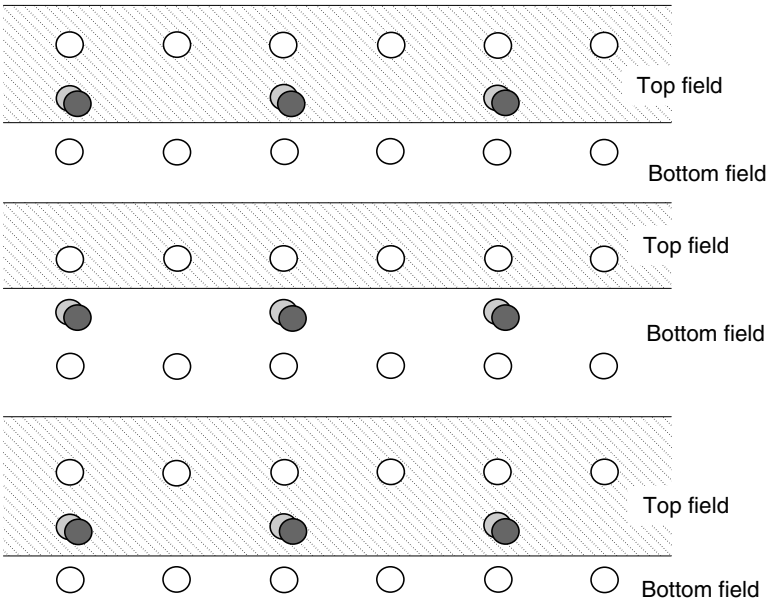
Figure 2.12 Allocation of 4:2:0 samples to top and bottom fields
