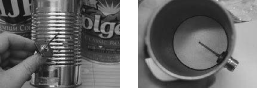
Figure A.30 Inserting the connector and probe into the can.
