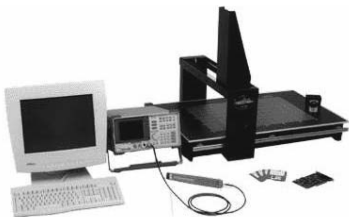
Figure 9.48 EMC scanner for top-sided electromagnetic field measurements. (Photograph courtesy of Detectus AB.)
