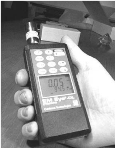
Battery-powered probe with directional antenna and LCD display of field strength in V/m
