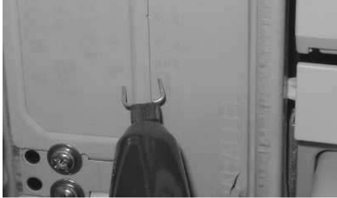
Figure 9.40 Voltage measurement across seam using a differential probe. (Photograph courtesy of Doug Smith.)
