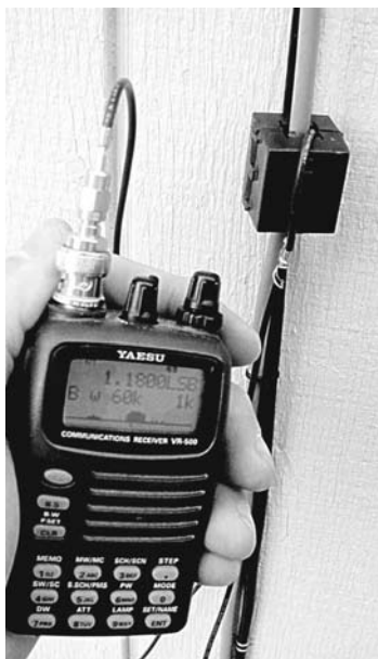
Figure 9.25 Using a radio receiver for EMI troubleshooting. (Photograph courtesy of Cortland Richmond.)
