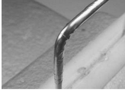
Figure A.5 Detail of bend in a corner. Three layers of tape are used to seal the crack on the outer portion of the wire.
