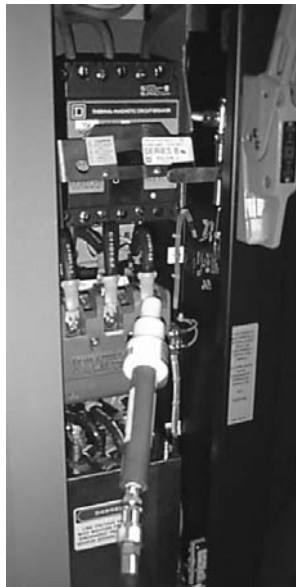
Figure 6.6 Use of a voltage probe to measure mains interference in situ.
