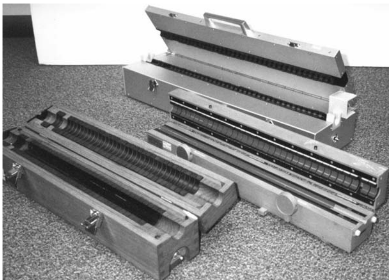
Figure 5.15 Typical absorption clamps. (Photograph courtesy of EMC Compliance Journal [2].)
