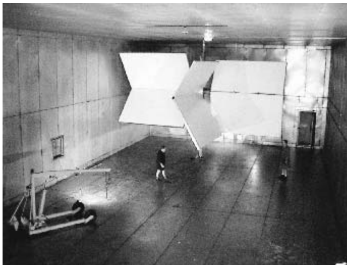
Figure 4.18 Typical reverberating chamber. (Photograph courtesy of Defence Science and Technology Organisation, Australia.)
