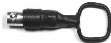
Figure A.9 Another layer of heat-shrink tubing finishes off the loop.
