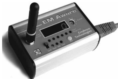
Figure 7.14 ESD environmental sensor. (Photograph courtesy of Credence Technologies.)
