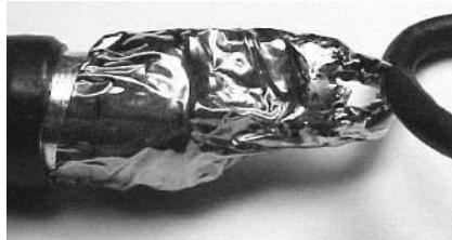
Figure A.8 Copper tape and solder connects two ends of loop foil together.
