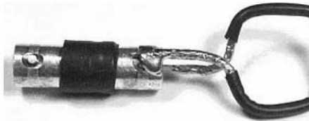
Figure A.7 Loop installed in BNC connector. Shield and wire are soldered to shell.
