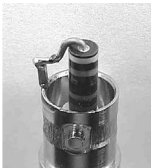
Figure A.21 Test circuit for measurement of capacitor self-inductance and ESR.
