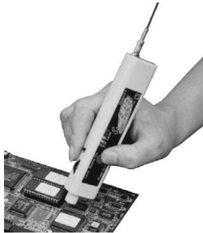
Battery-powered close-field probe with LED indication
