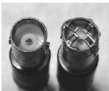
Step 1a 50-ohm termination.
