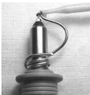
Figure A.19 FET probe shorted with short wire.
