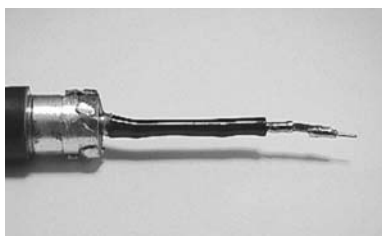
Step 4 Add heat shrink tubing.
