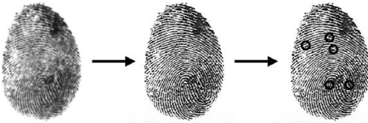
Figure 7.2. Automatic extraction of minutia.
