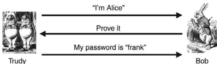
Figure 9.4. Simple authentication replay attack.
