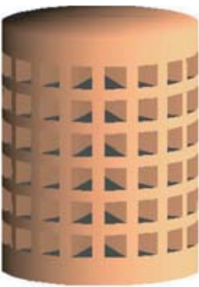
Figure 8.31. Dual polarized circular cylinder array with square waveguide aperture radiators, spacings 0.5 \lambda . Six of the 18 columns are active, tapered to -20 dB side-lobes, and phase steered.
