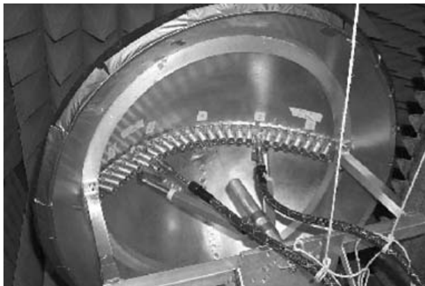
Figure 7.19. The inside of the experimental antenna when measuring the array mutual coupling along the y axis (cf. Figure 7.1). The probes, as well as the terminated elements in between are clearly visible. Courtesy of Ericsson Microwave Systems AB, Göteborg, Sweden.
