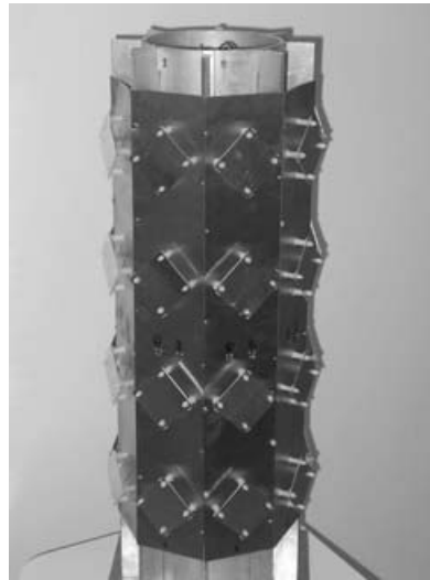
Figure 8.7. Cross section (a) of a cylindrical array demonstrator (b) with aperture-coupled patches [Raffaelli and Johansson 2003]. See also color insert, Figure 11. (Courtesy of Ericsson AB, Göteborg, Sweden.)
