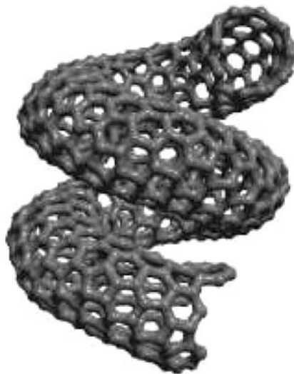
FIGURE 4.4 Nanotube with bends.
