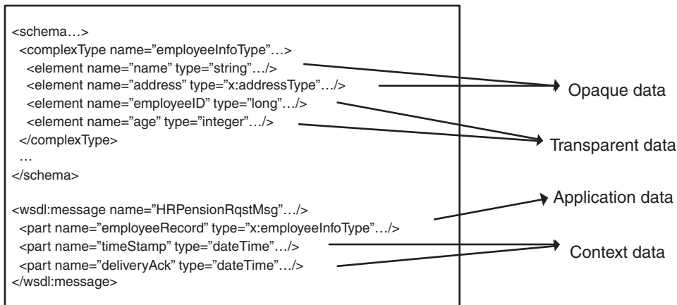
Figure 13.7 Data representation using WSDL messages.
