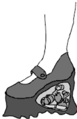
Figure 9.1 Nested doll TRIZ principle applied to shoe design. (From Shpakovsky, N. and Novitskaya, E., 2002, "Multifunctional Heel," downloaded from Generator Website at http://www.gnrtr.com/solutions/en/s040.html .)
