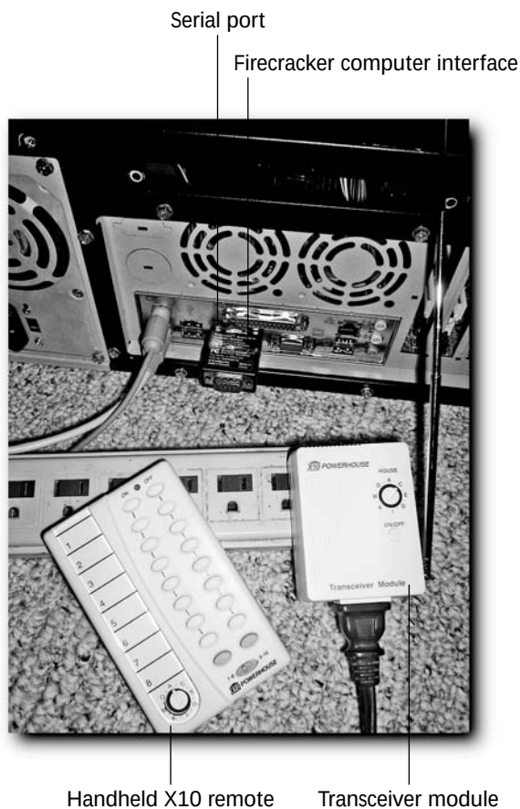
FIGURE 7-2: Firecracker requires a serial port and an electrical outlet to start.
