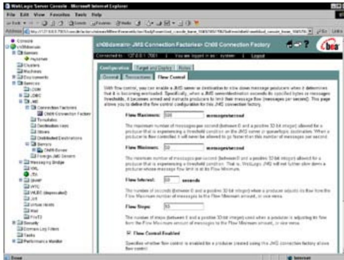
Figure 9.6: Configuring the flow control parameters.
