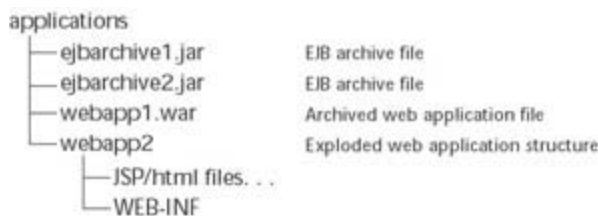
Figure 8.6: EJBs and Web apps deployed as separate applications.
