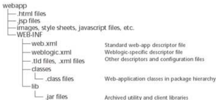
Figure 5.2: Standard Web application directory structure.
