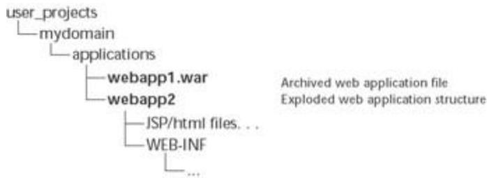
Figure 5.6: Web applications deployed in applications directory.
