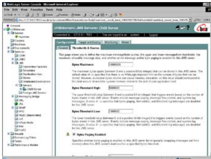
Figure 9.5: Configuring a JMS server's thresholds and quotas.
