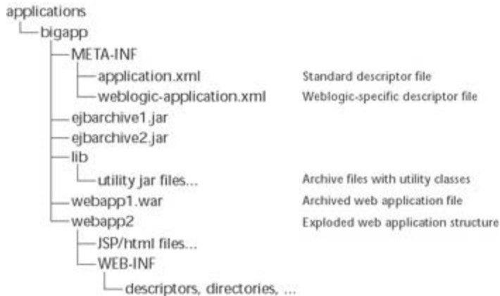
Figure 8.8: Standard enterprise application directory structure.
