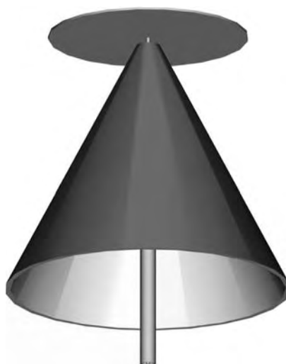
FIGURE 5-32 Disccone antenna with coaxial feed with a center conductor connected to the upper disk and a shield connected to the lower cone.
