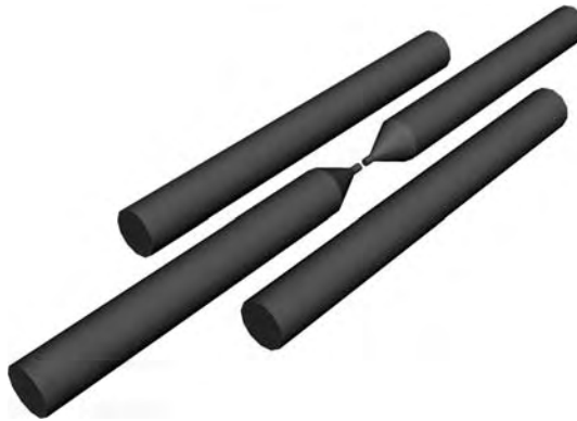
FIGURE 5-26 Open-sleeve dipole with conical input taper.
