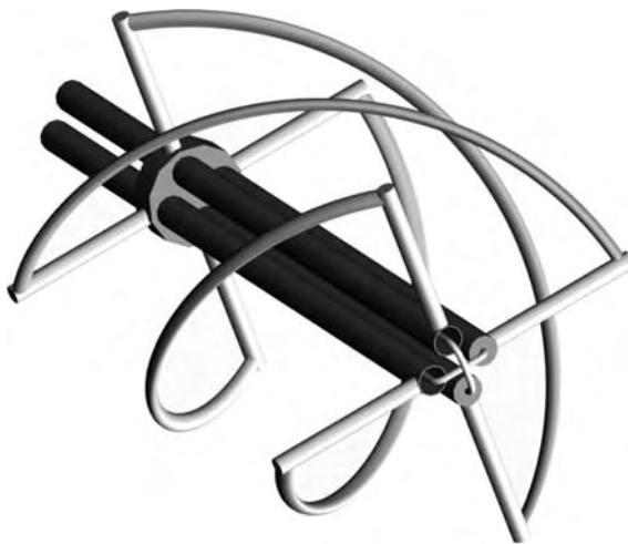
FIGURE 5-54 Half-turn quadrifilar helix fed from two folded baluns.
