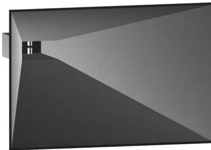
FIGURE 2-13 MOM model of a pyramidal horn using flat plates fed by a small dipole. (From [14, p. 229].)
