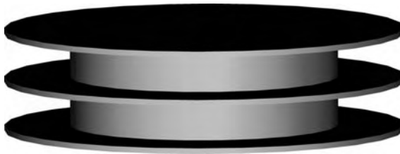
FIGURE 7-12 Ground plane with short-circuited radial transmission-line corrugations.
