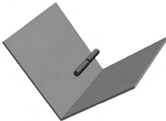
FIGURE 2-4 Corner reflector with a dipole located between two flat plates.
