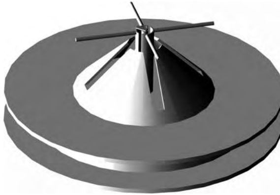
FIGURE 5-14 Turnstile dipole mounted over a notched cone on a finite circular ground plane with radial line chokes to reduce the backlobe.
