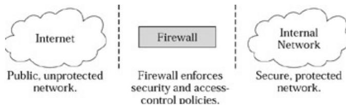
Figure 6.1: How a firewall works.
