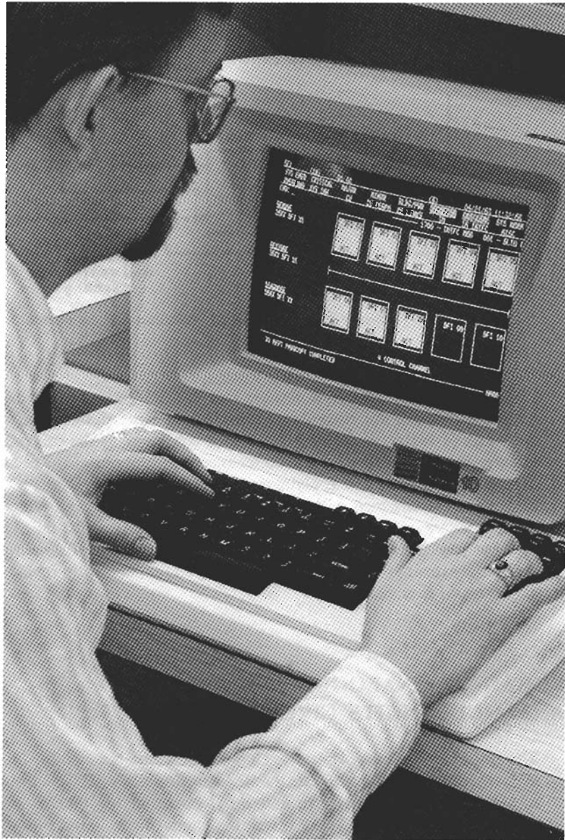
Figure 36.2 Maintenance workstation. The AT&T 5ESS telephone exchange now includes a video monitor that displays colour-coded diagrams, each of which indicates the status of a certain part of the system. A central office technician is checking the status of digital trunks. ( Courtesy of AT&T )
