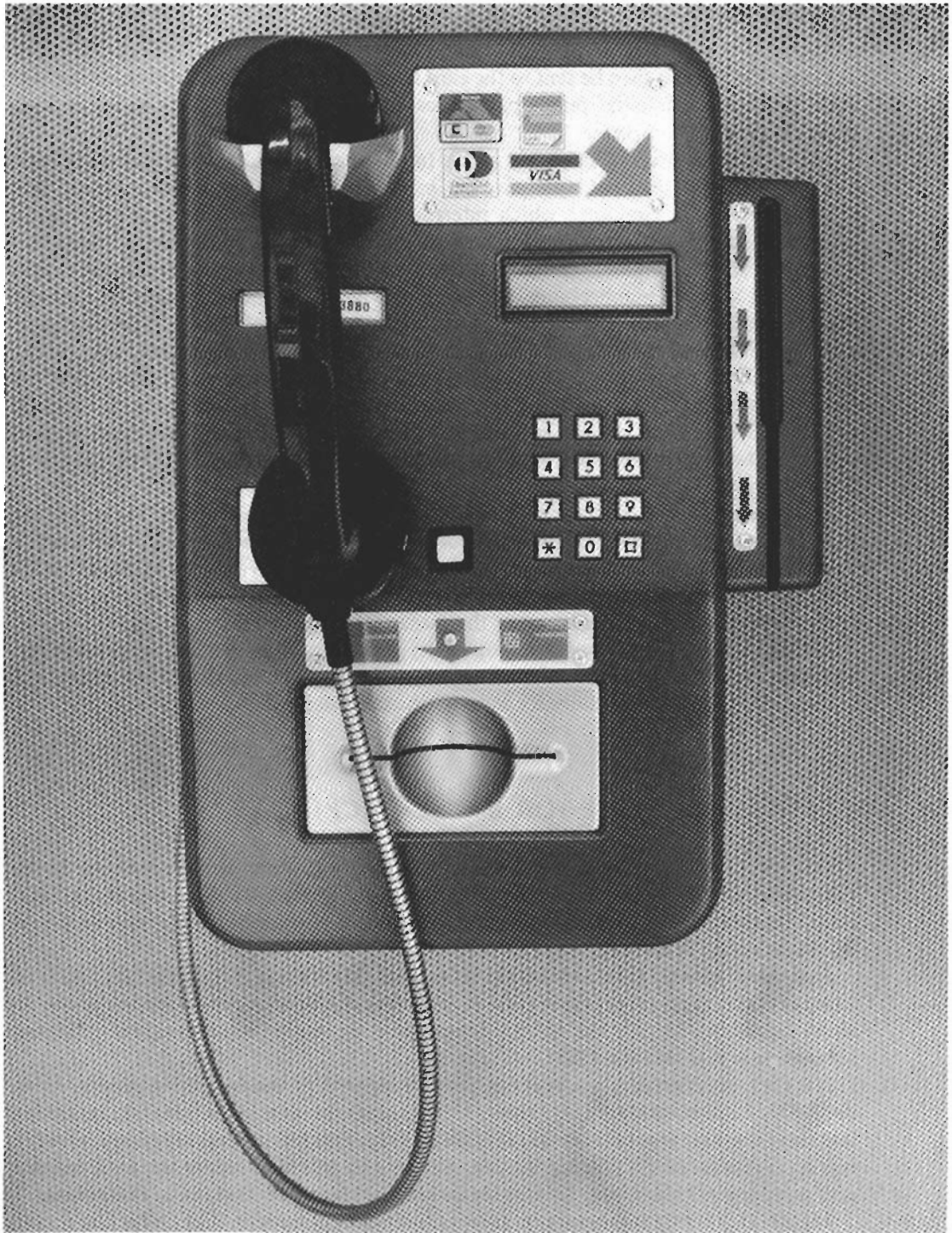
Figure 11.2 Credit card telephone. Telephone specially designed to allow payment for public telephone calls by credit or calling card. (Courtesy of British Telecom)
