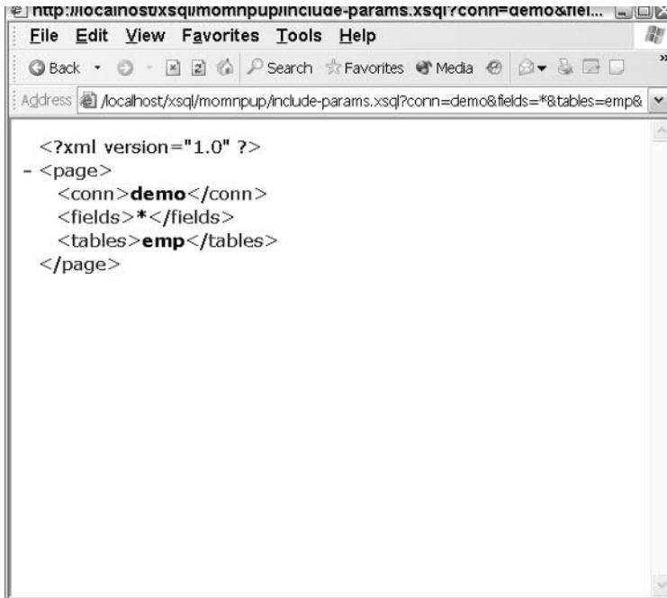
Figure 6.2 XML representation of parameters.
