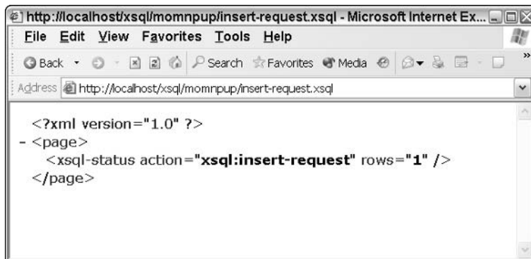
Figure 7.3 Result of insert-request action.
