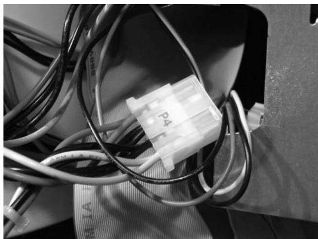
Figure 7-2: Power connectors located inside of your PC cabinet.
