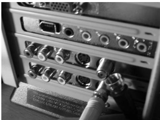
Figure 6-5: Connecting a set-top box to the TV tuner card using an S-Video connection.
