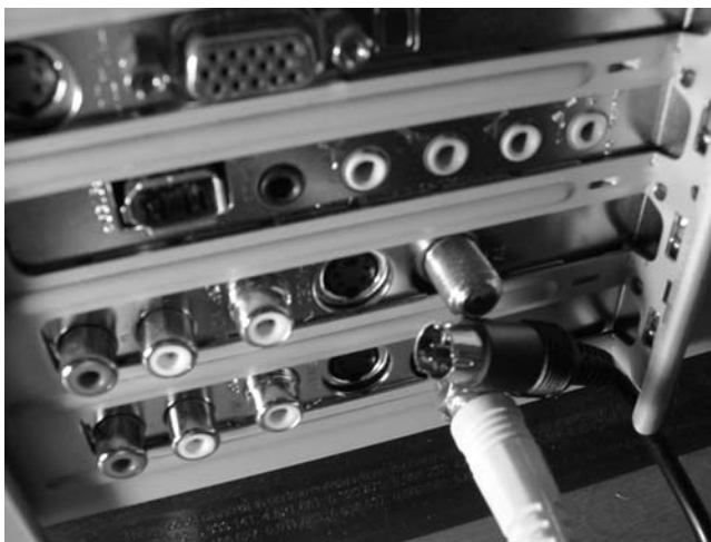
Figure 6-3: Antenna and basic cable connection.
