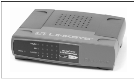
Figure 4-2: This compact Ethernet switch from Linksys is about the size of a paperback book. The sixth connector (on the right) can be used to expand the network using a second switch.
