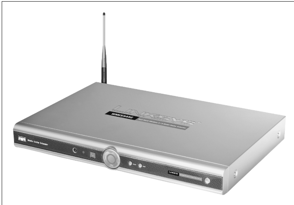
Figure 2-13: A Media Center Extender—such as the Linksys model shown here—brings Media Center PC features to any TV in your home. (Photo courtesy of Linksys.)
