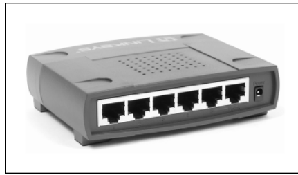
Figure 4-2: This compact Ethernet switch from Linksys is about the size of a paperback book. The sixth connector (on the right) can be used to expand the network using a second switch.
