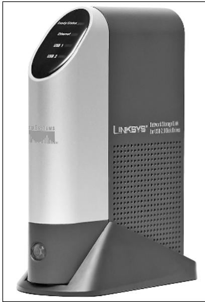
Figure 14-5: The Linksys NSLU2 NAS server packs a lot of power into a 5 1/2" box.
