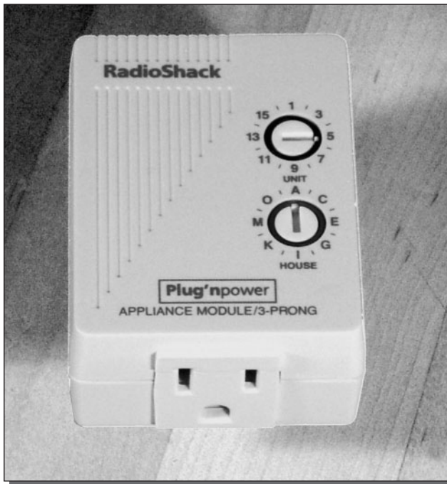
FIGURE 3-4: Heavy-duty appliance module
