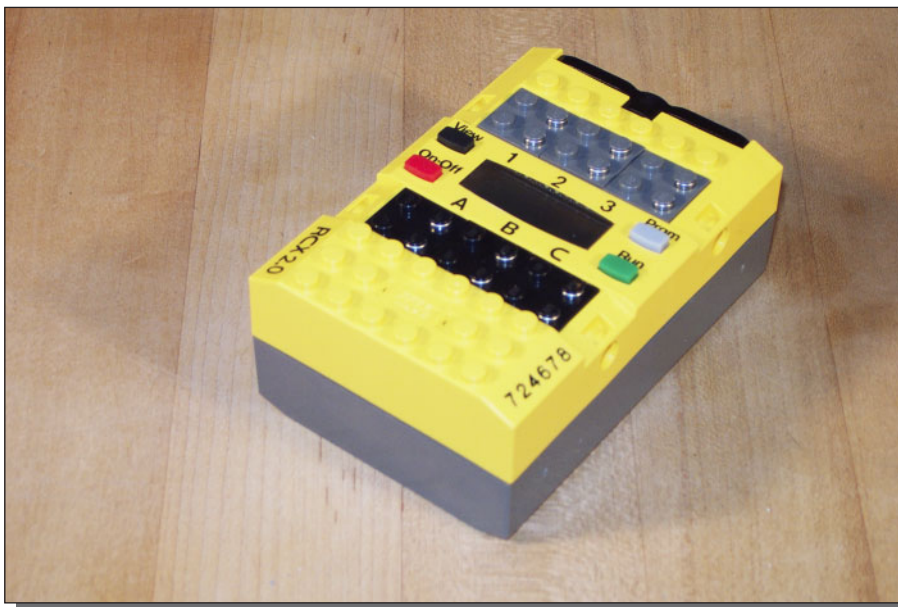
FIGURE 12-2: LEGO Robot Invention System RCX controller
