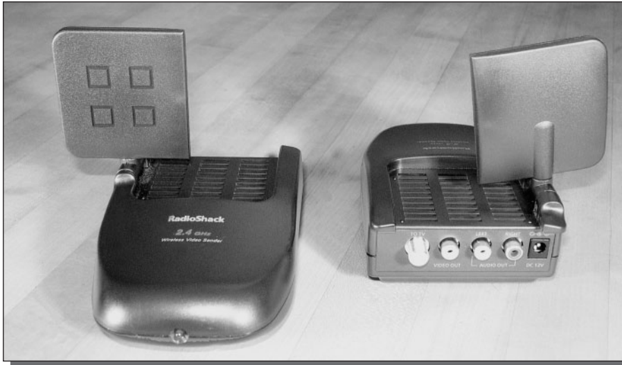
FIGURE 2-8: You can avoid running cables with a wireless connection, but you may lose some sound quality.
