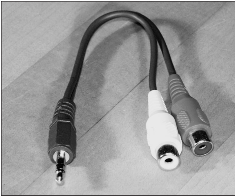
FIGURE 2-7: The female RCA connectors on this Y cable let you use any length patch cord to cable into your stereo preamp.
