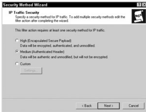
Figure 9-37: The IP Traffic Security screen
