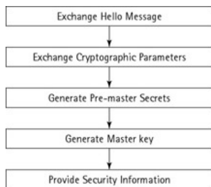
Figure 7-1: TLS Handshake Protocol
