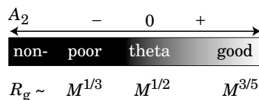
Figure 2.27. Molecular-weight ( M ) dependence of the radius of gyration R_g changes as the solvent quality, and therefore the second virial coefficient A_2 , change.
